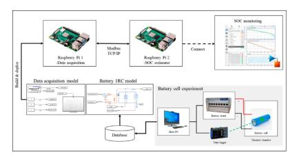
Figure 4. System architecture of SOC estimation using embedded boards.
