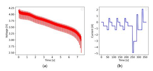
Figure 6. DST operating profile: (a) measured voltage and (b) current in one cycle (360 s).
