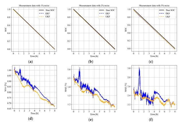
**Figure 11.** Estimation results in operating temperature 25  $^{\circ}$ C: true SOC vs. estimation methods according to including noise (a) 1%, (b) 2%, (c) 5%. Difference between the true SOC and the estimated SOC of the estimation methods in noise (d) 1%, (e) 2%, (f) 5%.
