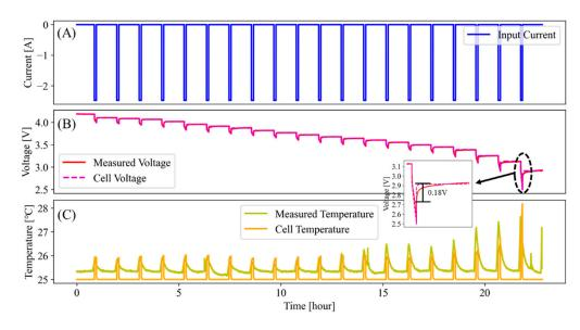
**Figure 3.** Results of battery model: **(A)** current profile, **(B)** comparison with simulation voltage and measured voltage, **(C)** cell temperature.
