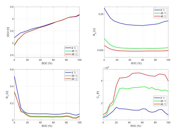
Figure 2. Battery parameter obtained for first-order RC circuit according to operating temperature.
