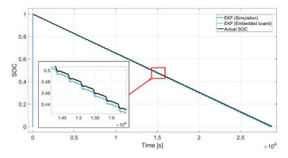
Figure 9. SOC estimation between embedded board and simulation.
