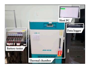
Figure 5. Battery experimental platform.
