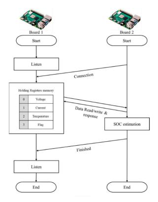
Figure 8. Scheme of communication protocol between Raspberry Pi.
