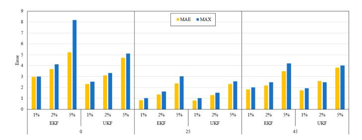
**Figure 12.** Comparison of overall EKF and UKF performances according to operating temperature including input noise.
