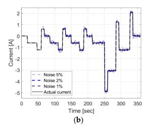
Figure 10. Measured voltage and current profile from a noise model: (a) voltage and (b) current.
