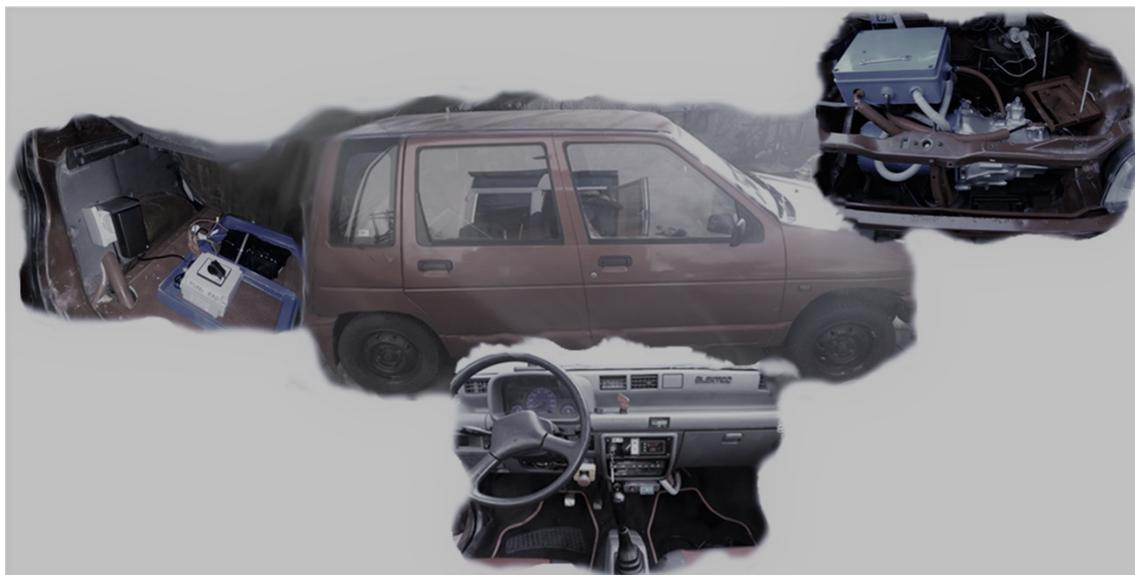
**Figure 1.** Laboratory production of EV Daewoo Tico with the AGM battery pack.
