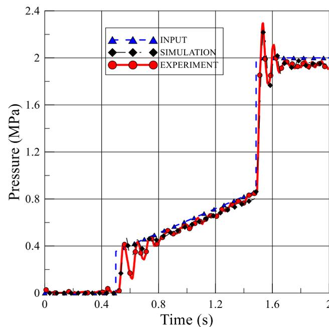
**Figure 10.** Buffer characteristics experiment and simulation comparison curve.
