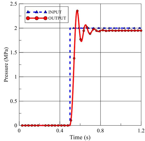
**Figure 5.** The 2D digital buffer valve's step characteristic curve.
