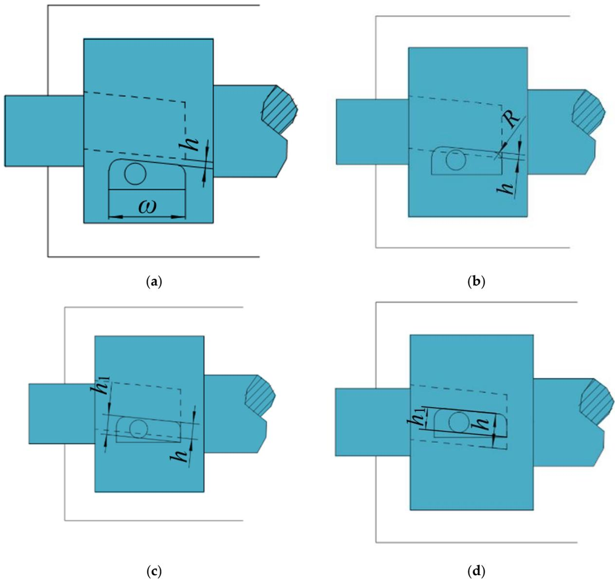
**Figure 3.** Change in overlap area between high- and low-pressure holes and chute: (a)  $h \leq 0$ ; (b)  $0 < h \leq R$ ; (c)  $R < h \leq h_1$ ; (d)  $h_1 < h$ .
