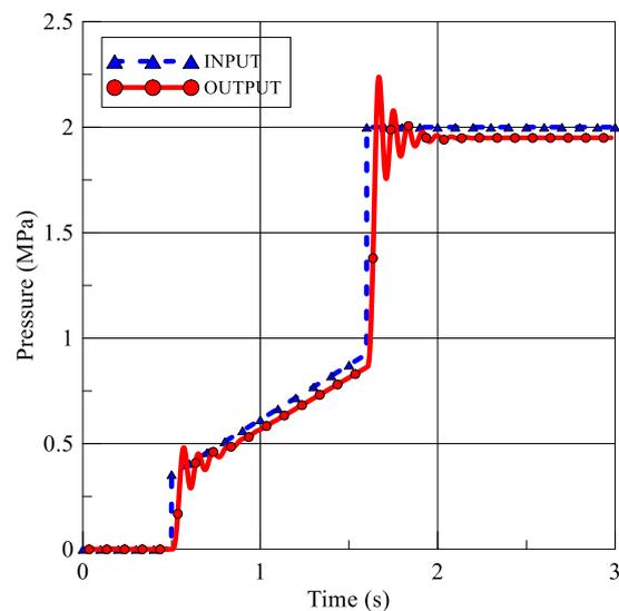
**Figure 6.** The 2D digital buffer valve cushioning characteristic curve.
