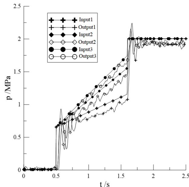
**Figure 11.** The 2D digital buffer valve's buffer following the characteristic curve.
