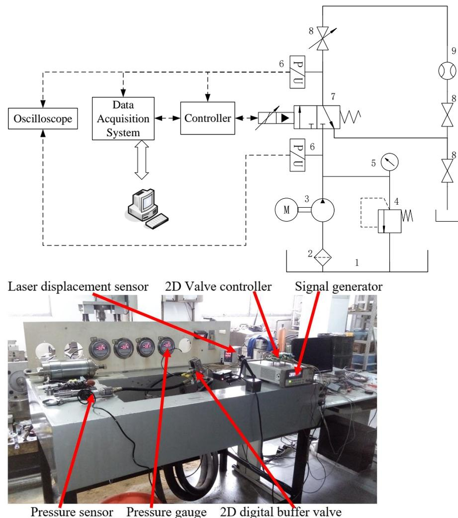
**Figure 7.** The 2D digital buffer valve buffer characteristics test platform. 1: tank; 2: filter; 3: pump; 4: relief valve; 5: pressure gauge; 6: pressure sensor; 7: 2D digital buffer valve; 8: globe valve; 9: flowmeter.
