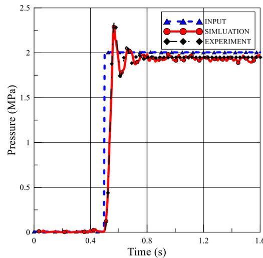
Figure 9. Step response characteristics of 2D digital buffer valve.
