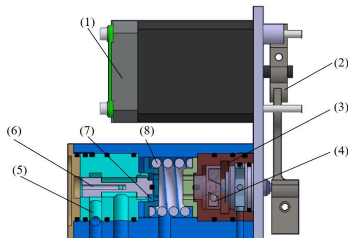
**Figure 1.** Diagram of 2D digital buffer valve structure. (1) Electromechanical converter; (2) transmission mechanism; (3) pilot valve sleeve; (4) pilot main spool; (5) main valve sleeve; (6) main spool; (7) spring seat; (8) spring.
