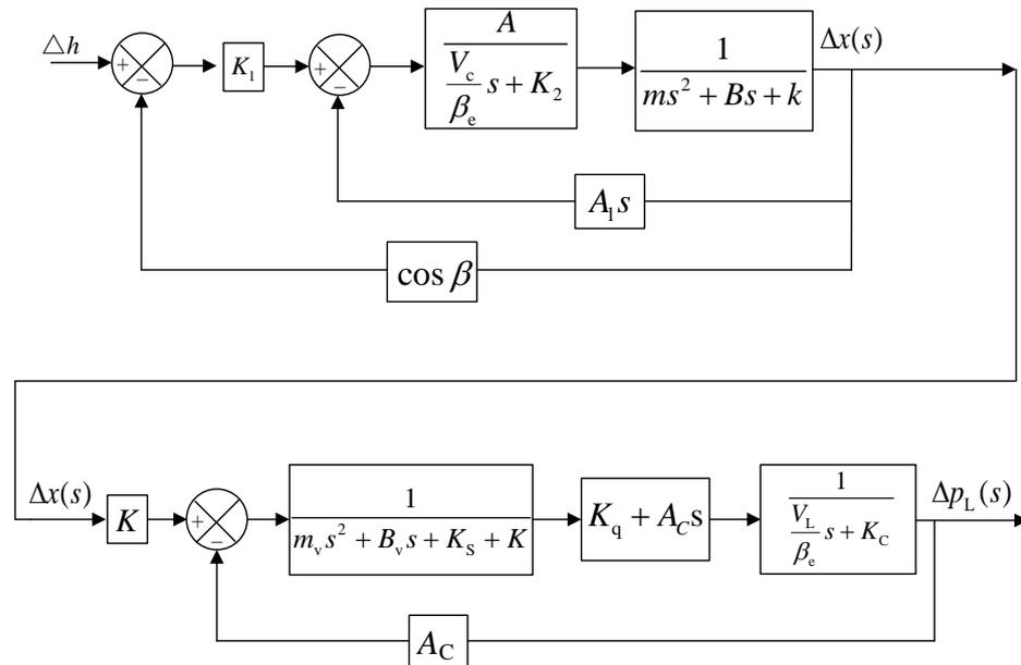
Figure 4. The 2D digital buffer valve transfer function block diagram.
