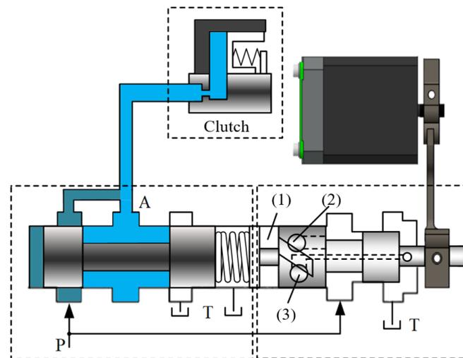
**Figure 2.** Diagram of 2D digital buffer valve working principle. (1) Sensitive cavity; (2) high-pressure hole; (3) low-pressure hole.
