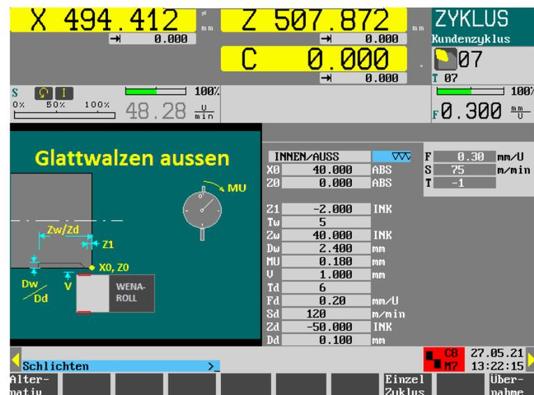
**Figure 3.** Roller burnishing cycle mask (German edition). Source: R&D Steuerungstechnik GmbH & Co.KG.
