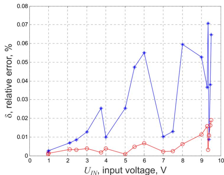
**Figure 4.** Graphs of the processing error of the multifunctional ADCF converter: 10-bit (blue \*) and 12-bit (red o), for five input voltages.
