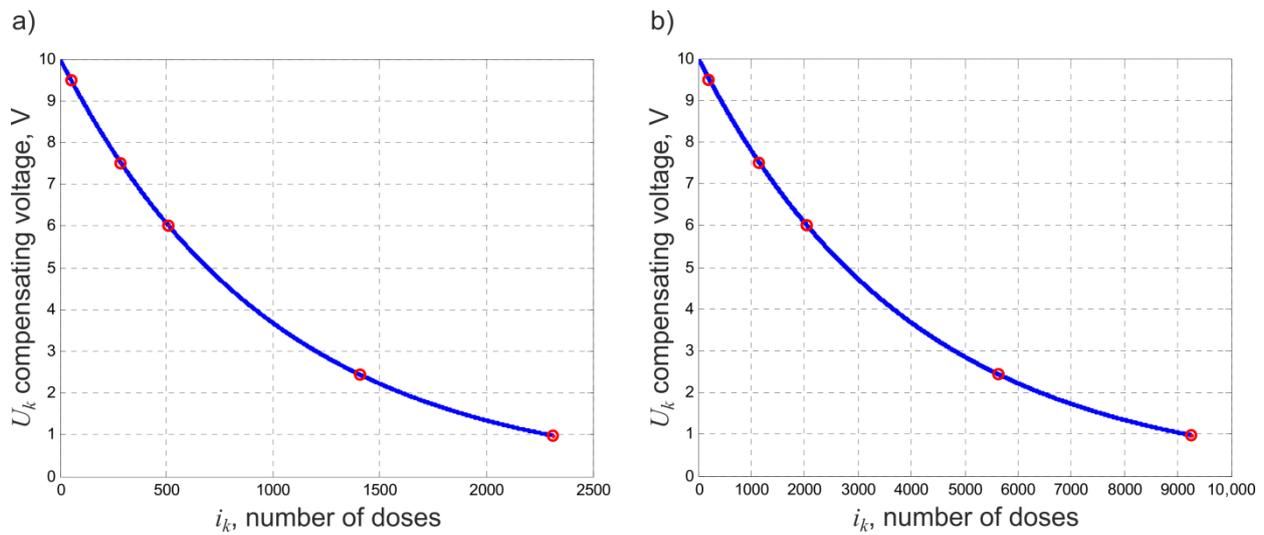
**Figure 3.** Operation graphs of the multifunctional ADCF converter for five input voltages:  $U_{IN1} = 9.5$  V;  $U_{IN2} = 7.5$  V;  $U_{IN3} = 6$  V;  $U_{IN4} = 2.44$  V;  $U_{IN5} = 0.99$  V for the given errors: (a) 0.1% and (b) 0.025%.
