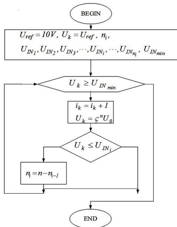
Figure 2. Generalised block diagram of the algorithm of operation of a multi-input multifunctional ADCF.
