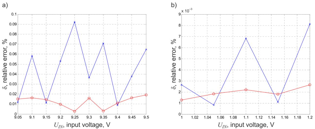
**Figure 6.** Graphs of the relative processing error of the multifunctional ADCF converter for 10 input voltages and set errors of 0.1% (blue x) and 0.025% (red o): (a) for the upper part of the operating range; (b) for the lower part of the operating range.
