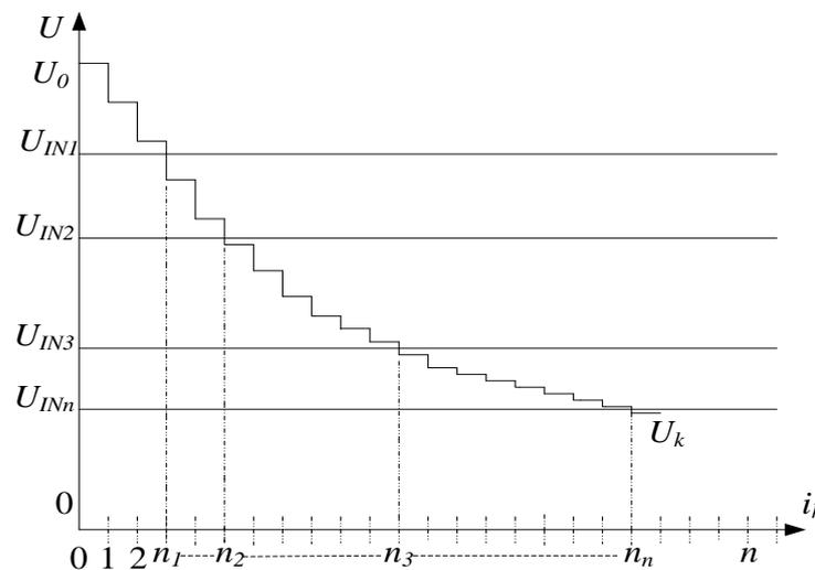
Figure 1. Voltage diagrams of a new method for functional analogue-to-digital conversion.
