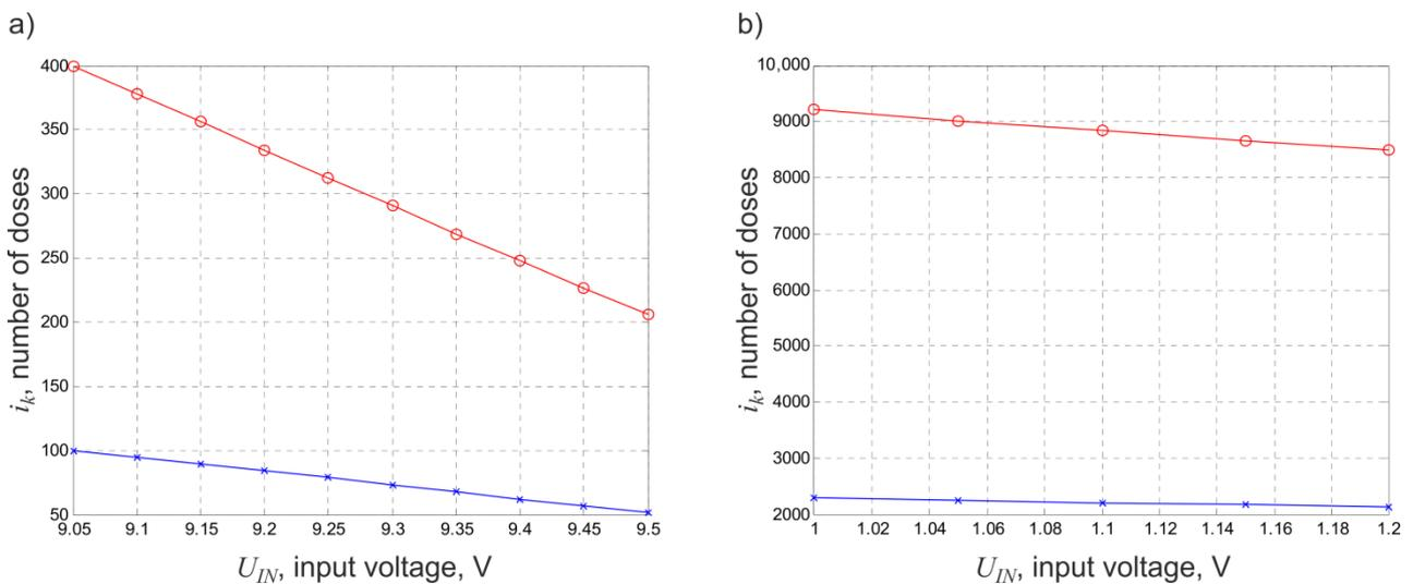
**Figure 7.** Processing time diagrams of the multifunctional ADCF converter for 10 input voltages and set errors of 0.1% (blue x) and 0.025% (red o): (a) for the upper part of the operating range; (b) for the lower part of the operating range.
