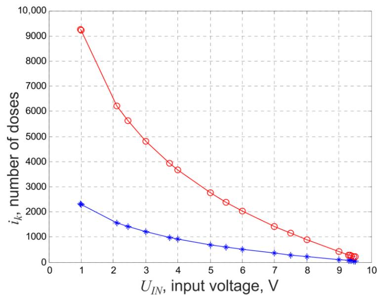
**Figure 5.** Graphs of processing time of the multifunctional ADCF: 10-bit (blue \*) and 12-bit (red o), for five input voltages.
