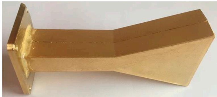
**Figure 16.** Assembled horn antenna with a gold-plated surface.
