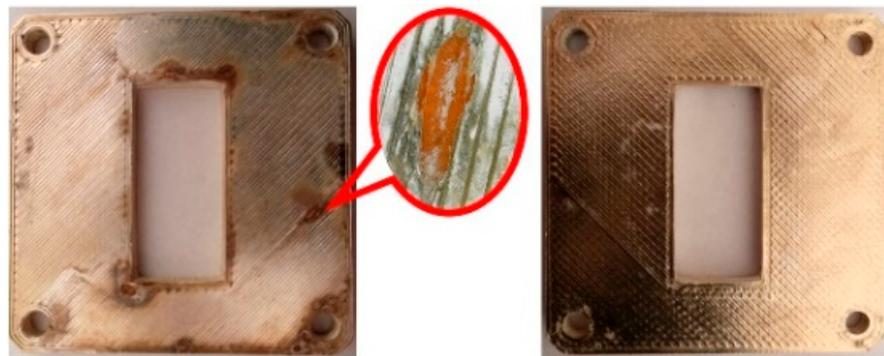
**Figure 14.** Horn antenna flange with (left) wrong thickness of gold layer; (right) proper thickness of gold layer.
