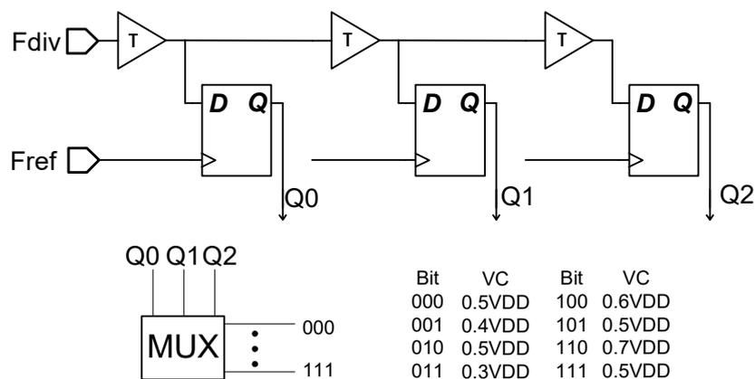
Figure 3. The transformation between phase error and common-mode voltage.
