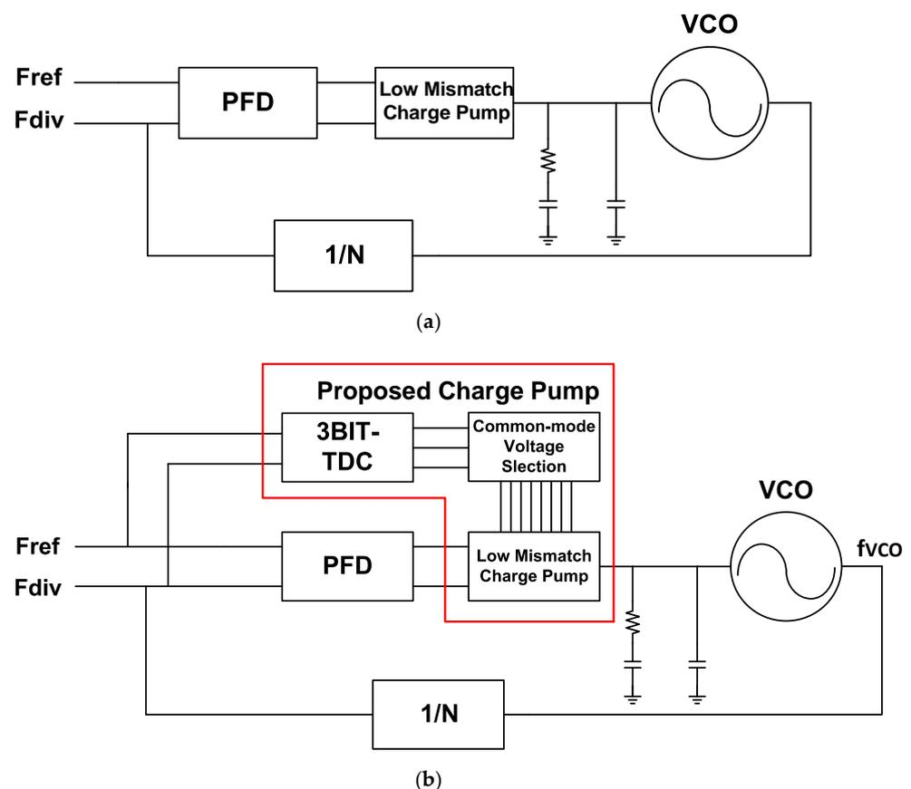
Figure 1. The main structure of (a) a traditional PLL design, and (b) the proposed CP in PLL.
