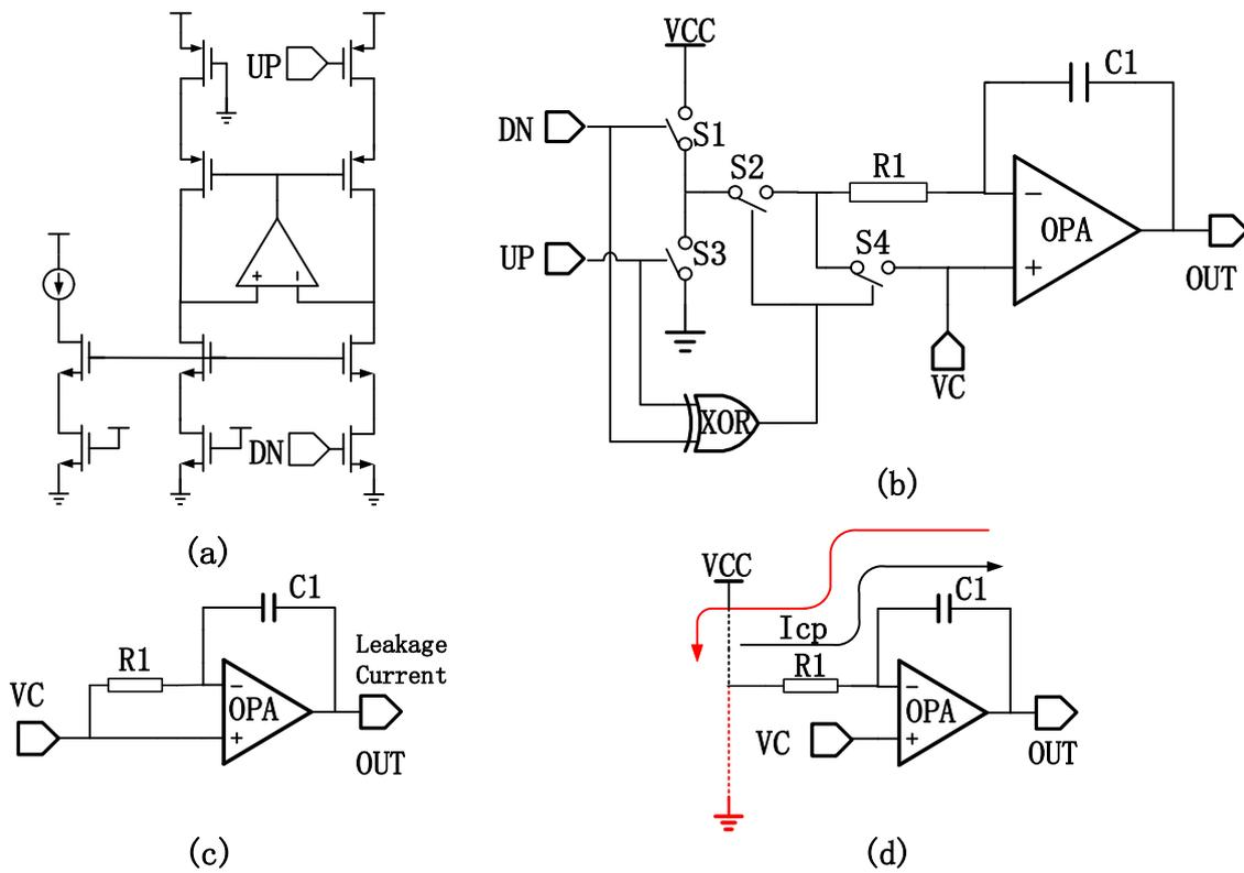
**Figure 2.** (a) Structure of a traditional OPA-based CP; (b) circuit schematic of the optimized CP; (c) the optimized CP in locking mode; and (d) the optimized CP in discharging/charging mode.
