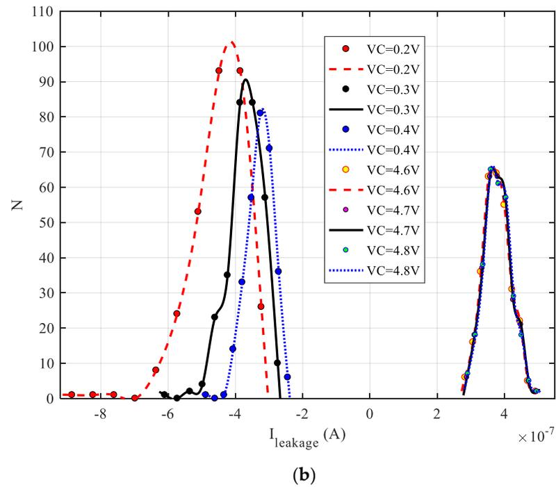
**Figure 5.** (a) Variation of the leakage current with the common mode voltage, and (b) leakage current corresponding to extended VC.
