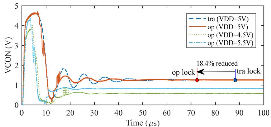
**Figure 10.** The simulated settling time of the optimized CP and traditional CP without phase error compensation under different supply voltages.
