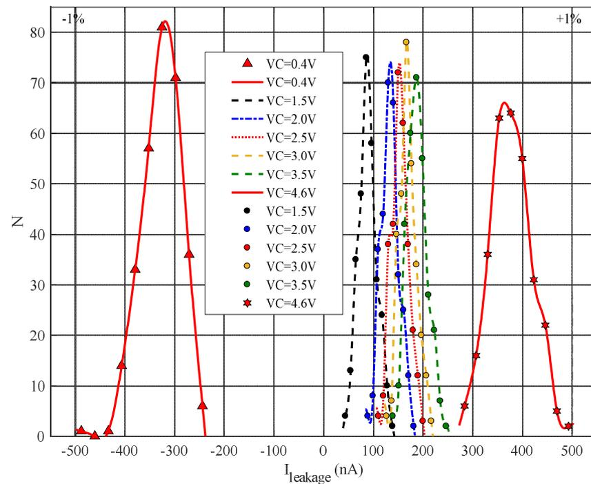
**Figure 6.** Distribution of leakage current for various common mode voltages. The result is obtained from Monte Carlo simulation with 300 points.
