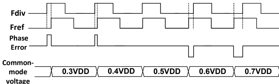
Figure 4. The timing diagram of the sampling circuit.
