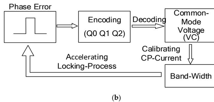
**Figure 9.** (a) Simulated PLL lock process optimized by the proposed CP; and (b) the workflow of the PLL locking process.
