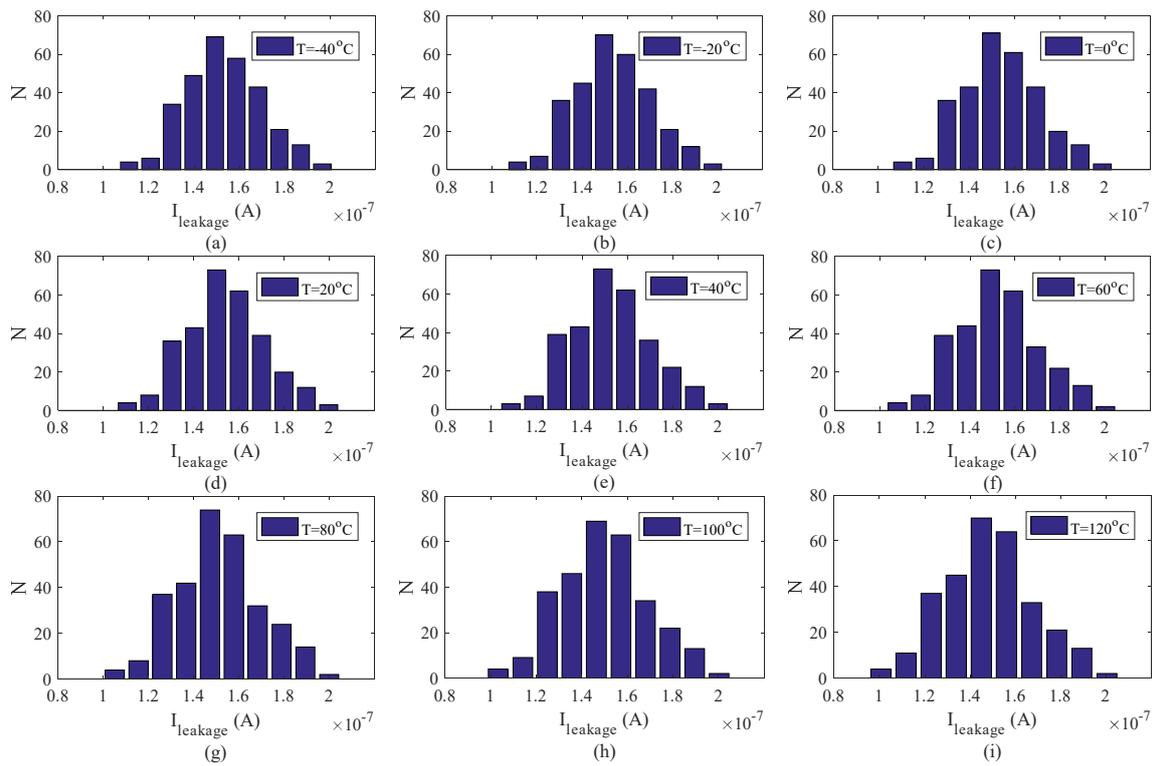
**Figure 7.** Distribution of leakage current  $I_{leakage}$  for  $VC = 2.5$  V at various temperatures: (a)  $-40$  °C, (b)  $-20$  °C, (c)  $0$  °C, (d)  $20$  °C, (e)  $40$  °C, (f)  $60$  °C, (g)  $80$  °C, (h)  $100$  °C and (i)  $120$  °C.
