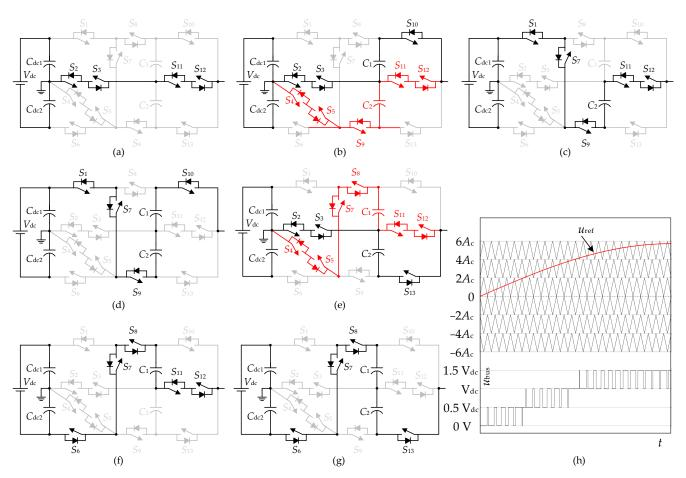
**Figure 2.** Main switching states of the proposed three-phase SCMLI at (**a**) 0 V, (**b**) 0.5 V<sub>dc</sub>, (**c**) V<sub>dc</sub>, (**d**) 1.5 V<sub>dc</sub>, (**e**) -0.5 V<sub>dc</sub>, (**f**)  $-V_{dc}$ , and (**g**) -1.5 V<sub>dc</sub>. (**h**) The waveform of the phase opposition disposition PWM in the positive quarter cycle (switching frequency  $f_s = 5$  kHz).
