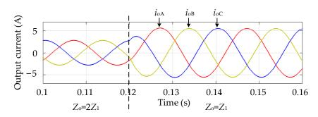
Figure 20. The output current of each phase during a resistive-inductive load transient.
