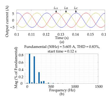
**Figure 9.** (**a**) The output current of each phase under the resistive–inductive load condition. (**b**) The FFT result of the A-phase output current.
