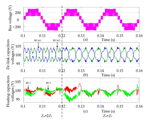
ages were limited to 96–104 V, as before. Figure 13c shows the A-phase floating capacitor voltages. During the same transient process,  $u_{C2}$  was momentarily larger than 105 V. After that, the floating capacitor voltages quickly returned to the steady state.
