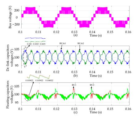
**Figure 7.** (**a**) The bus voltage, (**b**) DC-link capacitor voltages and (**c**) floating capacitor voltages of the A-phase under the resistive–inductive load condition.
