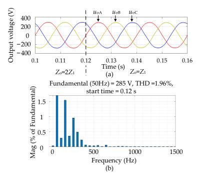
**Figure 11.** (**a**) The output voltage of each phase during a resistive–inductive load transient. (**b**) The FFT result of the A-phase output voltage.
