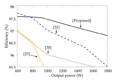
Figure 16. Recorded efficiency of different topologies.
