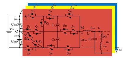
Figure 1. Proposed seven-level three-phase SCMLI topology.
