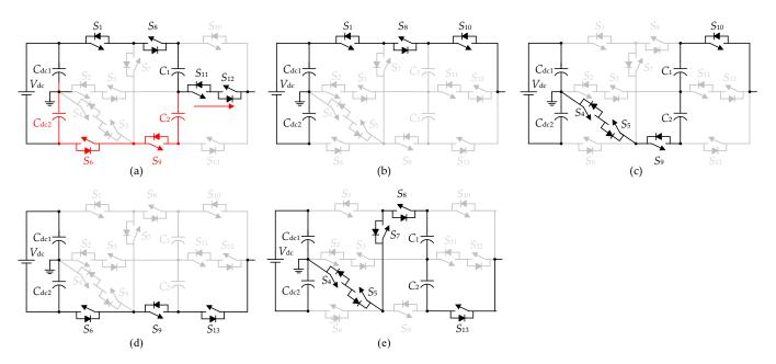
**Figure 5.** Redundant switching states of the proposed three-phase SCMLI structure at (**a**) 0 V, (**b**) 0.5 V<sub>dc</sub>, (**c**) V<sub>dc</sub>, (**d**) -0.5 V<sub>dc</sub>, and (**e**)  $-V_{dc}$ .
