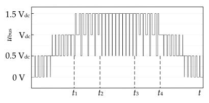
**Figure 6.** The new modulation wave in the positive half cycle (switching frequency  $f_s = 5$  kHz).
