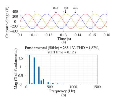
**Figure 8.** (a) The output voltage of each phase under the resistive–inductive load condition. (b) The FFT result of the A-phase output voltage.
