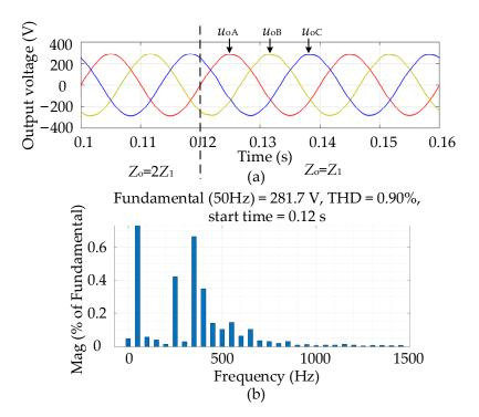
**Figure 19.** (**a**) The output voltage of each phase during a resistive–inductive load transient. (**b**) The FFT result of the A-phase output voltage.
