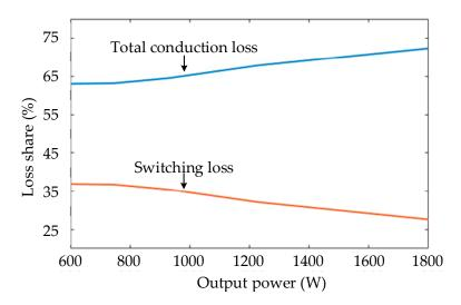
Figure 17. The share of switching loss and total conduction loss.
