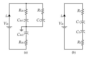
Figure 3. Equivalent circuit of (a) approach I and (b) approach II.
