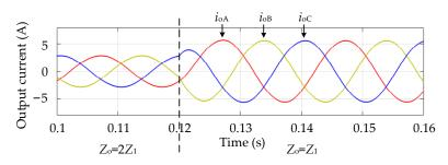
Figure 12. The output current of each phase during a resistive-inductive load transient.
