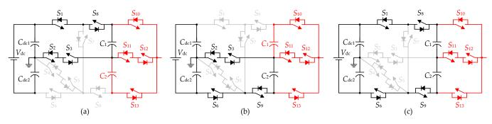
**Figure 4.** Switching states when (**a**) approach I is realized and  $C_1$  is used, (**b**) approach I is realized and  $C_2$  is used, and (**c**) approach II is realized.
