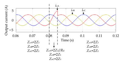
Figure 15. The output current of each phase when the disturbance load was added to the A-phase.
