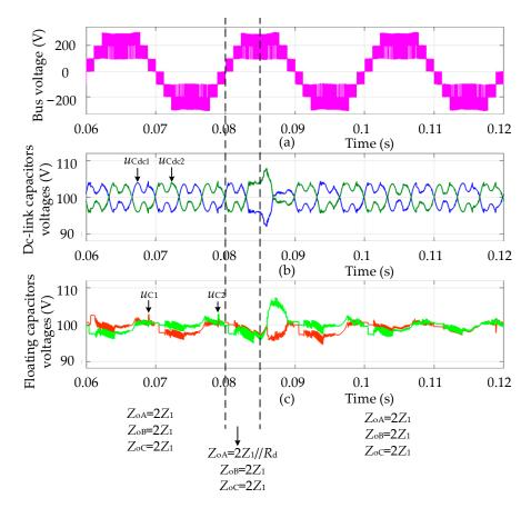
**Figure 13.** (**a**) The bus voltage, (**b**) DC-link capacitor voltages and (**c**) floating capacitor voltages of the A-phase when the disturbance load was added to the A-phase.
