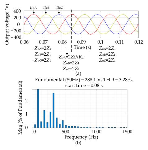
**Figure 14.** (**a**) The output voltage of each phase when the disturbance load was added to the A-phase. (**b**) The FFT result of the A-phase output voltage.
