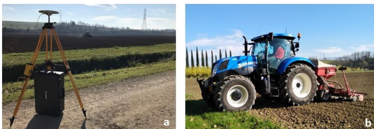
Figure 1. (a) RTK Base Station; (b) Tractor with technology IntelliSteer equipped with a pneumatic seeder.
