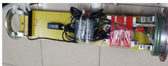
Figure 3. Photo of the experimental equipment with one three-axis fluxgate magnetic sensor.
