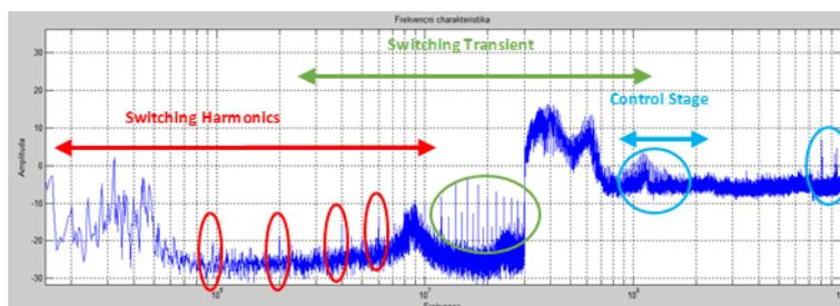
Figure 19. Measurements of power electronics effects as a function of the frequency range of power electronics.
