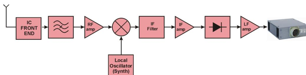
Figure 13. Superheterodyne receiver—simplified block diagram [5,14,20].
