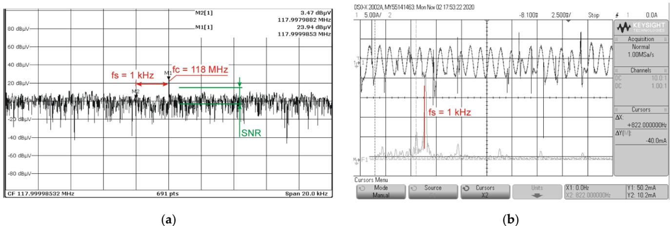
**Figure 7.** VHF receiver circuits in the disturbing environment, signal in the RF spectrum (a) and LF output signal, in time domain and its spectrum (b).
