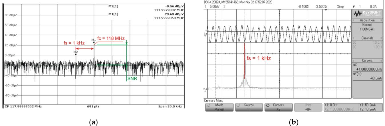
**Figure 6.** Test signal in the VHF bandwidth for aeronautical mobile services, (a) signal in the RF spectrum and the low-frequency (LF) output signal (b), in time domain and its spectrum.
