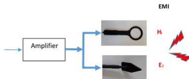
Figure 15. Realization of special electric and magnetic field probes.
