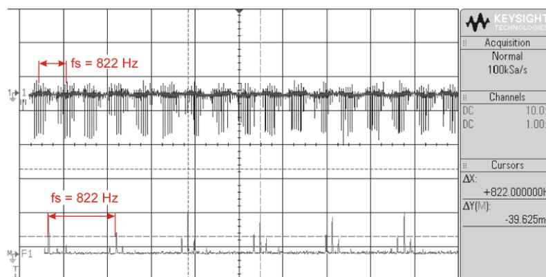
**Figure 5.** Characteristics of burst signal produced by power electronics.
