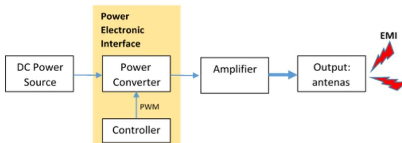
Figure 14. Testing source of electromagnetic interference.
