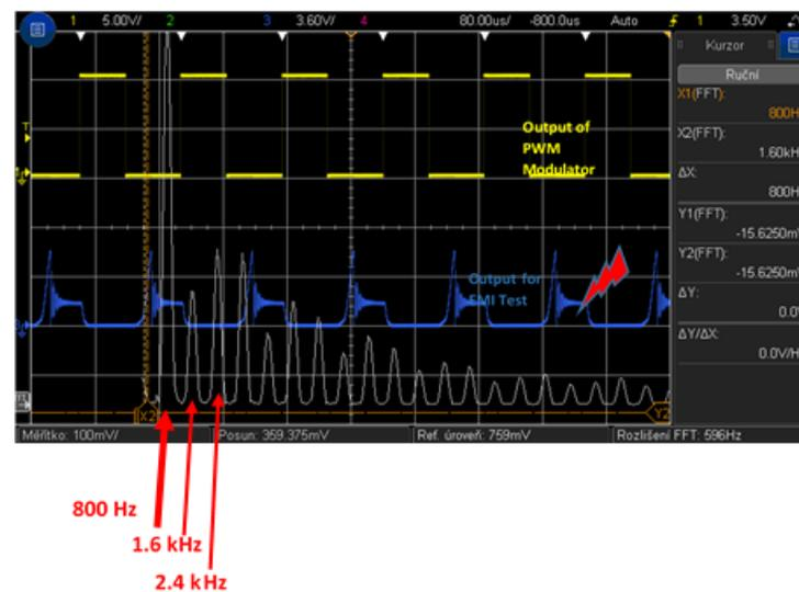
Figure 16. Generated interference signals.
