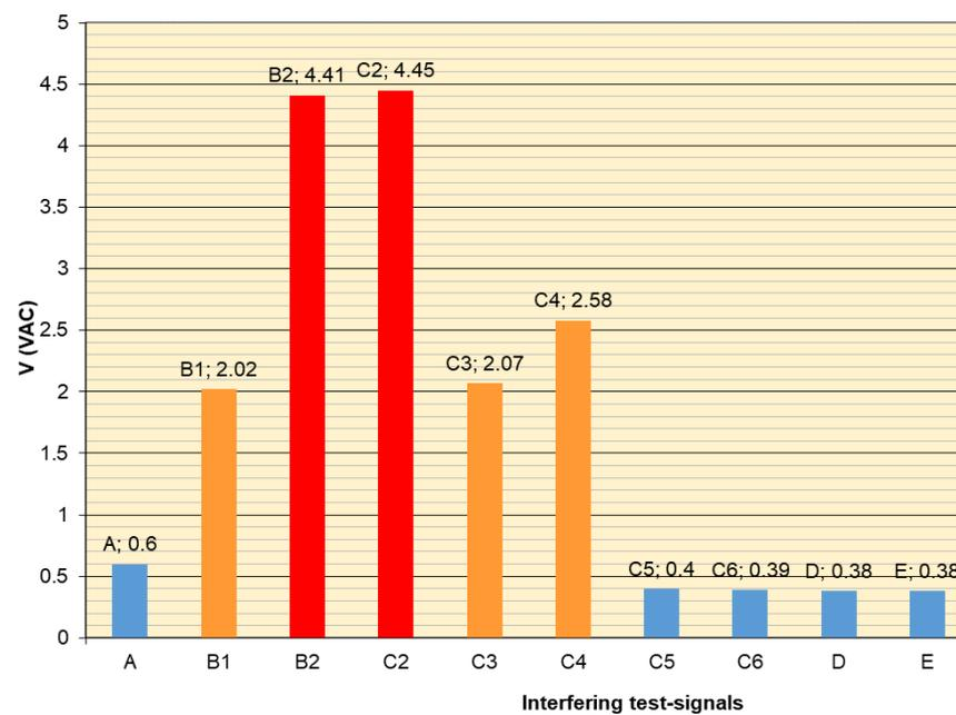
**Figure 18.** Measurements of susceptibility of the RF receiver LUN related to undesired signals of power electronics.
