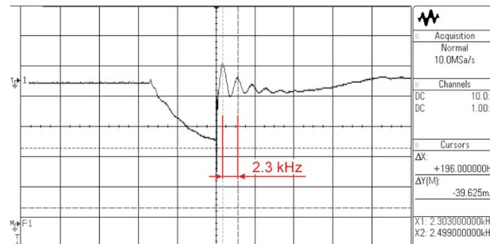
**Figure 8.** Details of simulated switching processing of SiC power component used in aircraft power electronics.
