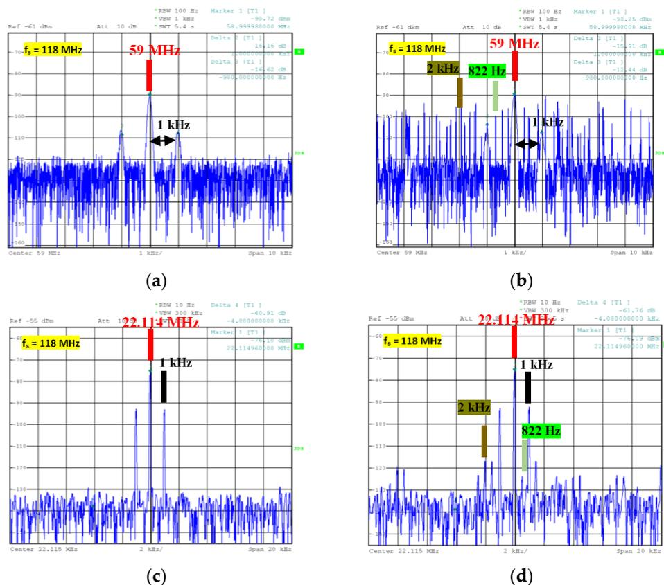
Figure 20. Resulting frequency spectrum for case of  $\frac{1}{2} f_s$ , (a) single amplitude modulation (AM) signal, (b) AM signal when DC-DC power converter is active, (c) single AM signal image frequency rejection, (d) DC-DC converter image frequency rejection.
