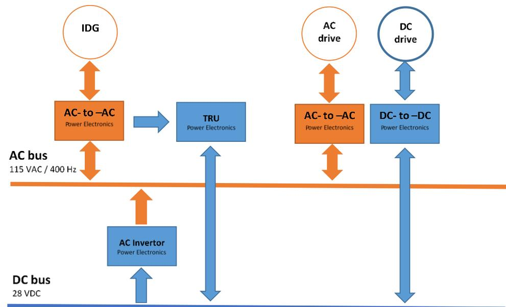
**Figure 2.** Power processing of onboard aircraft electronics.
