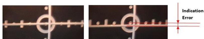
Figure 12. Indication error caused by ILS/GP disturbance.
