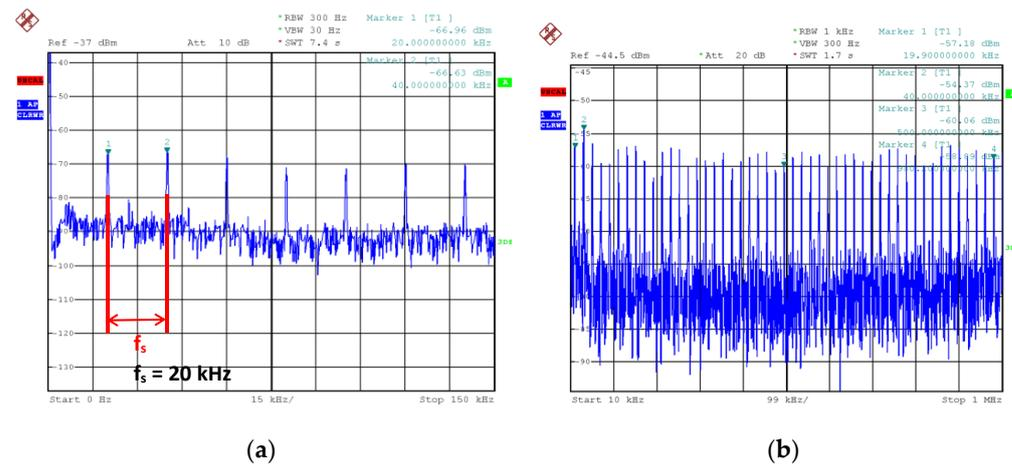
**Figure 3.** Power electronics electromagnetic interference (EMI): (a) conductive; (b) radiative.
