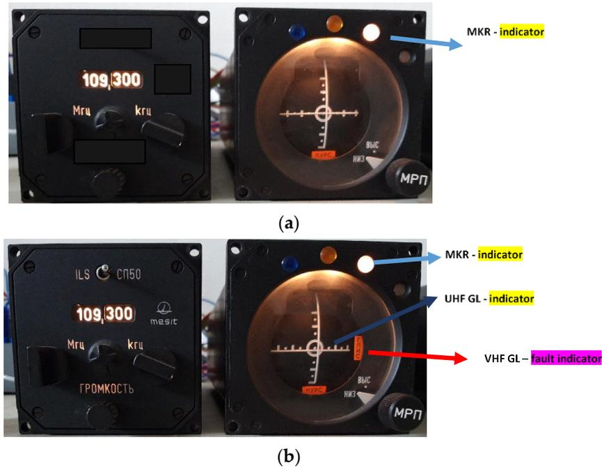
Figure 11. Disturbed marker (MKR) and GP channel of ILS receiver, (a) only inner marker interference, (b) disrupted GP receiver.
