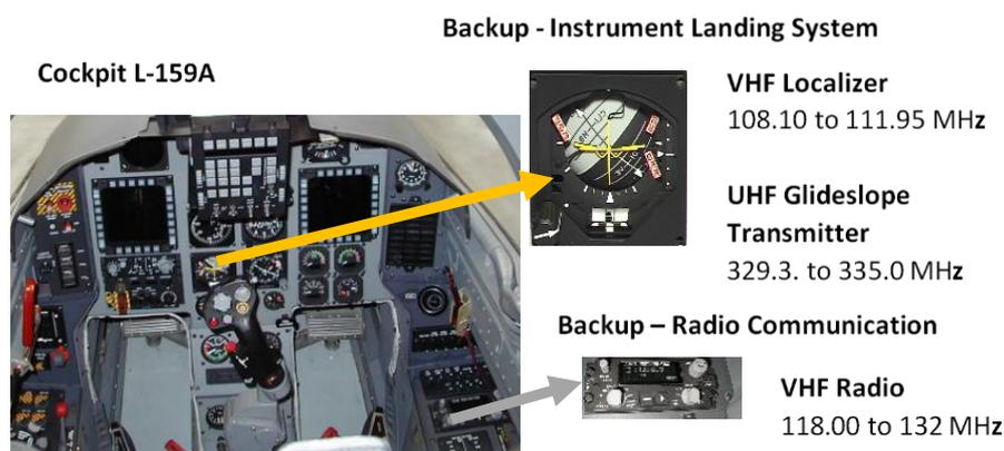
**Figure 1.** Very high frequency (VHF) radio systems in the cockpit of an L-159 aircraft.
