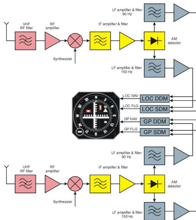
Figure 9. Instrument landing system (ILS) receiver block diagram.
