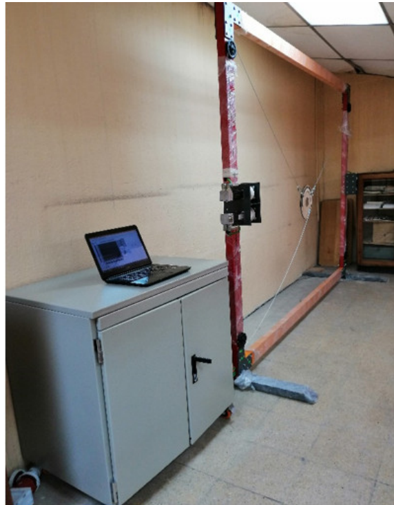
Figure 12. Planar CDPR assembled in the labs of Salesian Polytechnic University in Ecuador.
