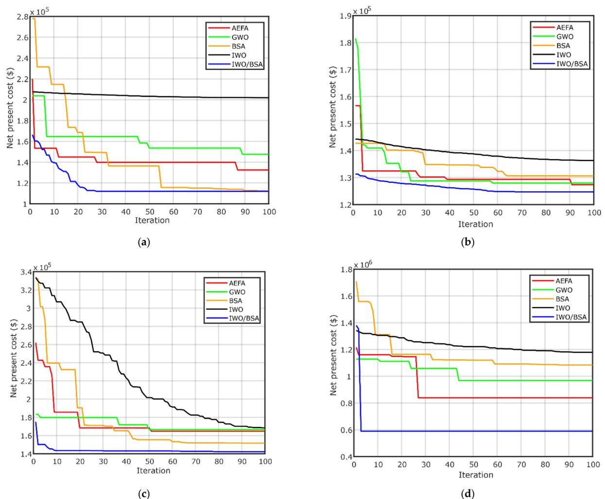
Figure 9. The NPC convergence using the proposed AEFA, GWO, BSA, IWO and the proposed IWO/BSA for all scenarios, (a) PV/WT/biomass/battery, (b) PV/biomass, (c) PV/diesel/battery, (d) WT/diesel/battery.
