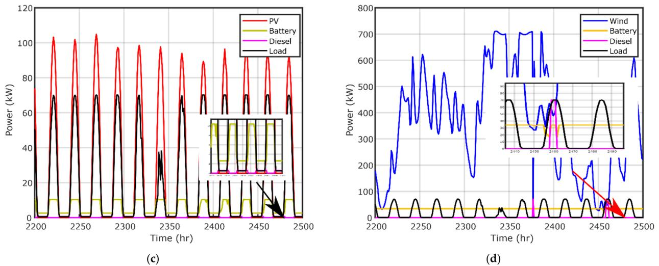
**Figure 12.** Time-response of PV, WT, battery, diesel generator, biomass, load powers obtained via the proposed IWO/BSA algorithm for all scenarios during some hours, (a) PV/WT/Biomass/Battery, (b) PV/Biomass, (c) PV/Diesel/Battery, (d) WT/Diesel/Battery.
