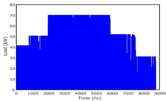
(c) Load for the PV/diesel/battery system
