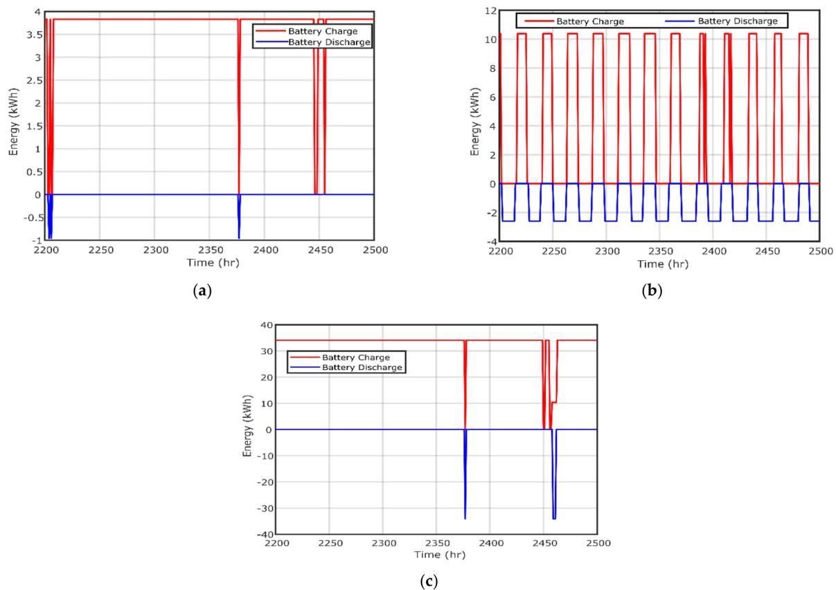
**Figure 14.** Charge and discharge of battery in scenarios, (a) *PV/WT/biomass/battery*, (b) *PV/diesel/battery*, (c) *WT/diesel/battery*.
