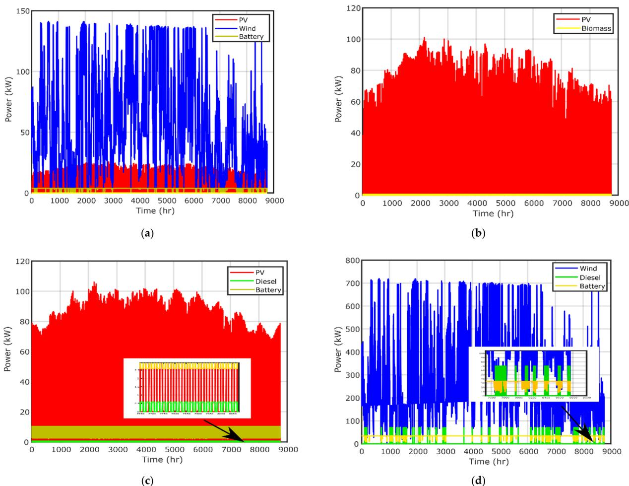
**Figure 10.** Annual contribution of *PV*, wind, battery, diesel, and biomass obtained by the proposed IWO/BSA algorithm, for scenarios (a) *PV/WT/biomass/battery*, (b) *PV/biomass*, (c) *PV/diesel/battery*, (d) *WT/diesel/battery*.
