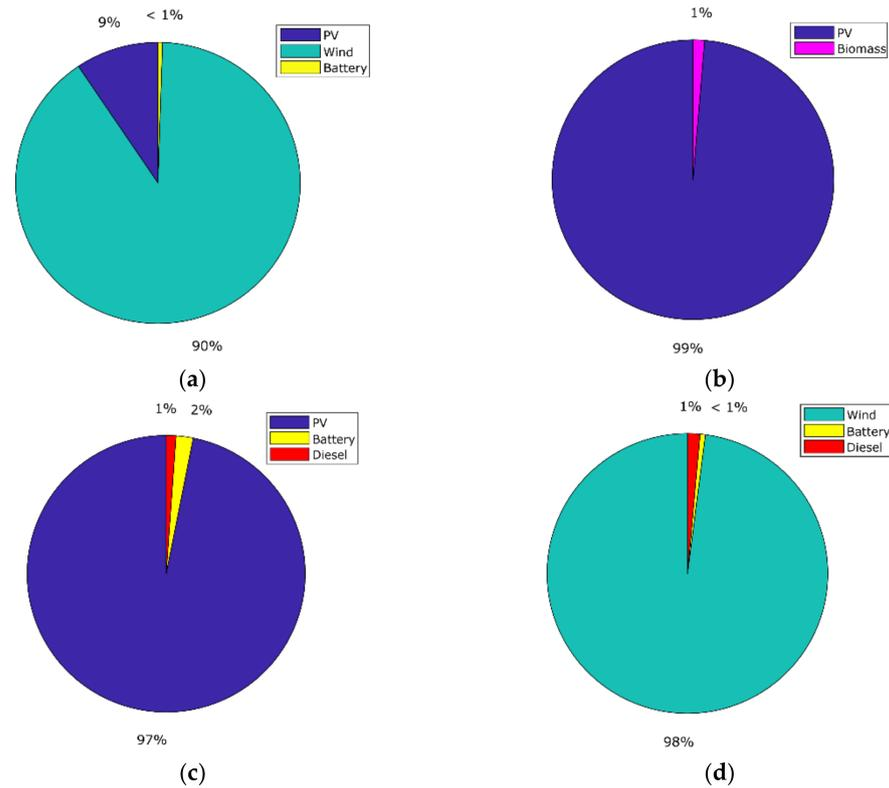
**Figure 11.** Annual contribution of PV, WT, battery, and diesel and biomass obtained by the proposed IWO/BSA algorithm, (a) PV/WT/biomass/battery, (b) PV/biomass, (c) PV/diesel/battery, (d) WT/diesel/battery.
