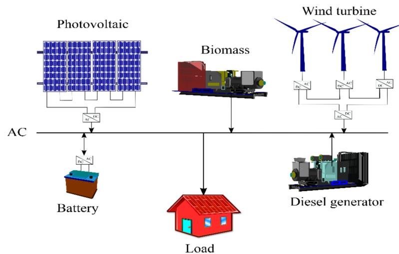
Figure 1. Isolated microgrid system components used for different scenarios.
