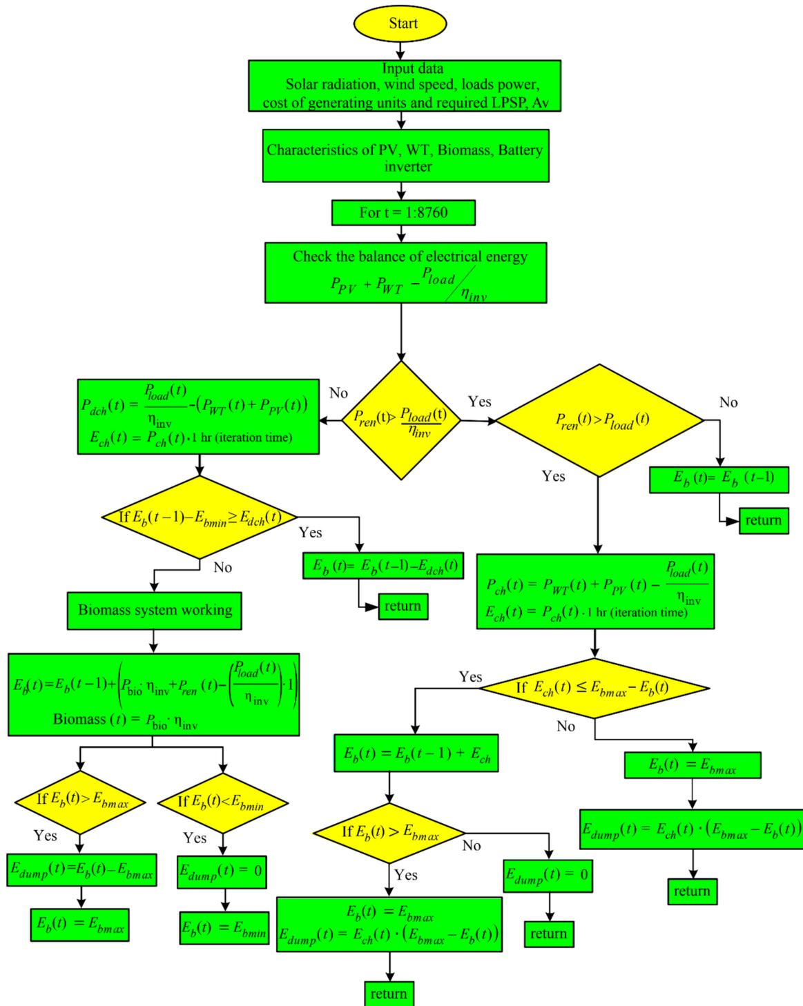
Figure 3. Power management of the PV/WIND/DIESEL/BESS.
