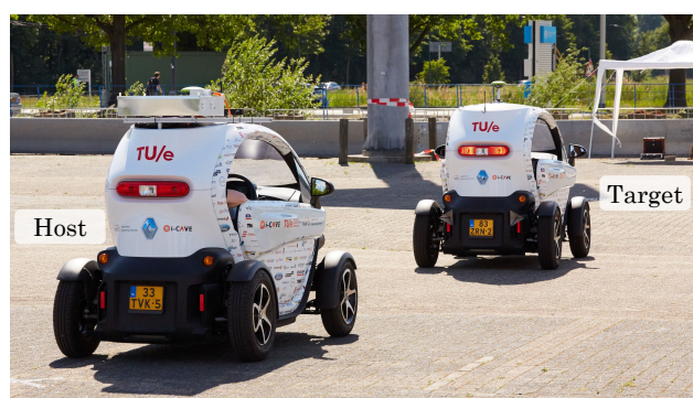
Figure 1. Two Renault Twizys modified for autonomous and cooperative driving in the i-Cave project [34,36]. The host vehicle (left) is following the target vehicle (right) in both longitudinal and lateral direction.
