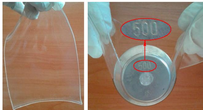
**Figure 6.** Experimental sample of hydrogel film.
