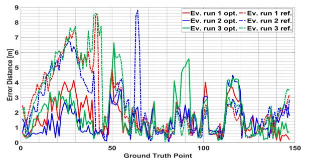
Figure 9. Position deviation of the evaluation runs for the Samsung Galaxy S7.
