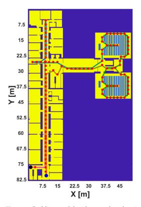
**Figure 7.** Building model with ground truth points (GTP) in red. The test runs started at GTP 1 (black) and ended at GTP 107 (blue). The path taken is approximately 583 steps or respectively 367 s long. The average walking speed was 1.6 m/s.
