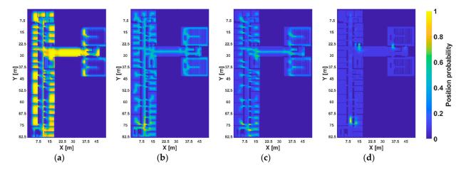
**Figure 5.** Resulting probability distributions: (**a**) reasoning map after five steps of only wall attenuation; (**b**) resulting probability distributions after 2, (**c**) 5, and (**d**) 20 steps.
