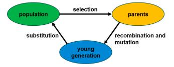
**Figure 6.** Structure of the Genetic Algorithm: The sequence of selection, recombination, mutation, and substitution is iteratively repeated until a stopping criterion is reached.
