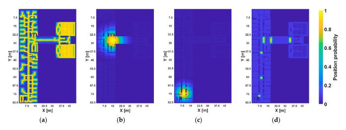
**Figure 3.** Measurement maps: (a) walkway structure of the indoor area; (b) Bluetooth Low Energy (BLE) fingerprinting based position estimation; (c) map of possible positions based on Wireless Local Area Network (WLAN) fingerprinting; (d) map of magnetic field anomalies.
