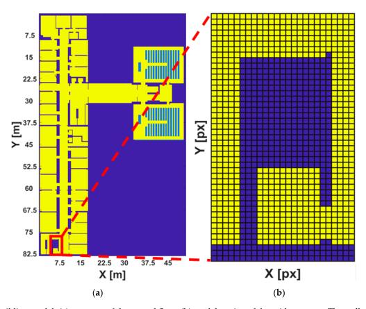
**Figure 1.** Building model: (a) structure of the second floor; (b) model section of the grid structure. The walkable indoor areas are represented by yellow pixels, while the areas unlikely to be entered are shown in azure-blue like desks or fixed rows of chairs in the lecture halls. All areas of the building which are not accessible are indicated by blue cells.
