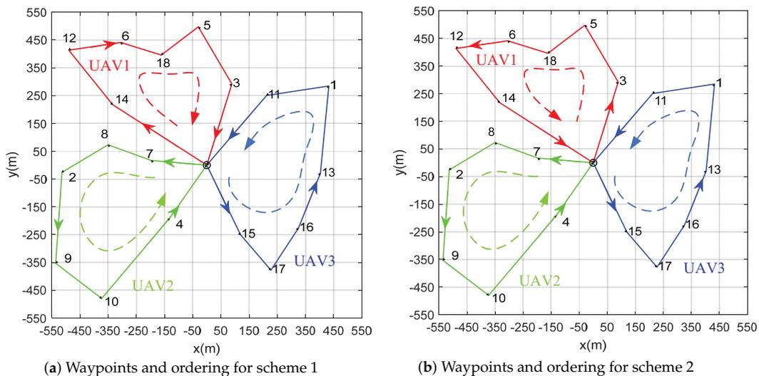
**Figure 3.** Illustration of the differences in the results of the modified genetic algorithm with two trajectory initializations: (a) The results with an initialization of the trajectories and visiting orders for the three UAVs in which two UAVs travel in the anticlockwise direction; (b) The results with another initialization of the scheme in which all UAVs travel in the anticlockwise direction.
