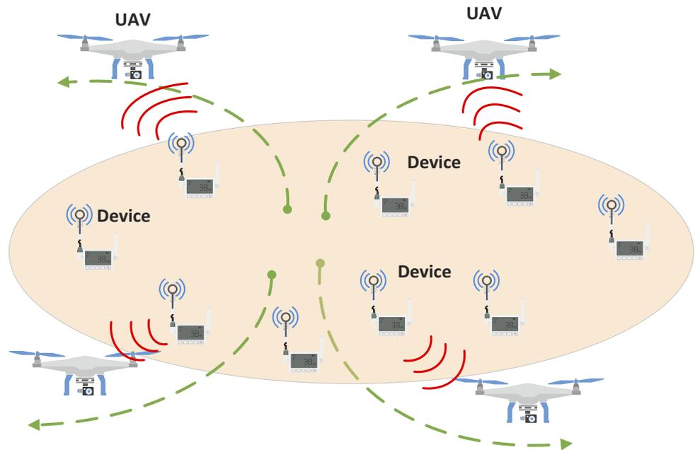
**Figure 1.** The multi-unmanned aerial vehicle (UAV)-enabled data collection scenario with channel interference, where multiple UAVs are flying in the sky to collect data from served devices and numerous sensors distributed over an area at fixed locations during a certain period. The dotted green lines represent the trajectories of the UAVs.
