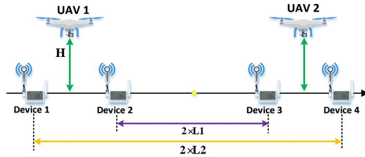
**Figure 2.** A basic network scenario with two UAVs and four devices, where the four devices are symmetrically distributed along a line and the two UAVs fly at a constant height to collect data from their served devices.
