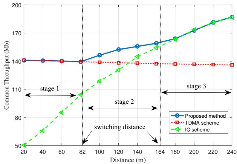
Figure 6. Common throughput of the network versus the distance between devices for different schemes.
