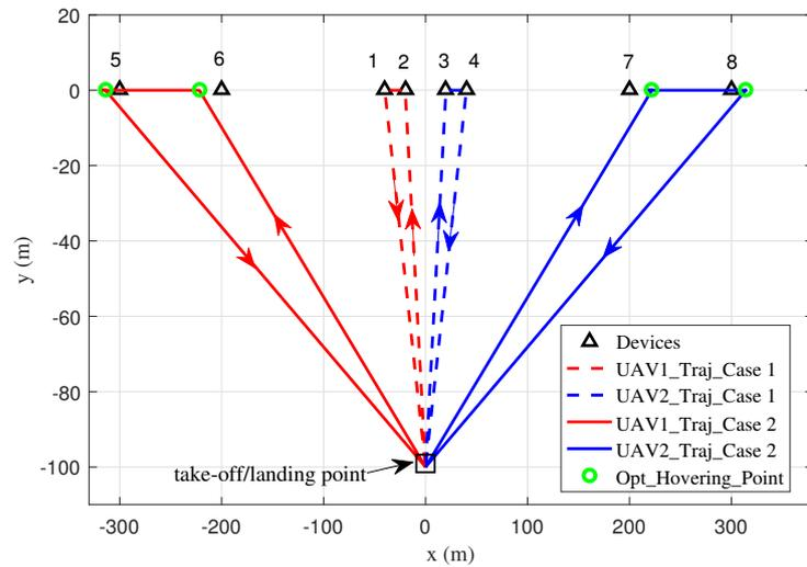
Figure 5. Optimal trajectories of the two UAVs for the quasi-stationary scenario with  $T = 26$  s.
