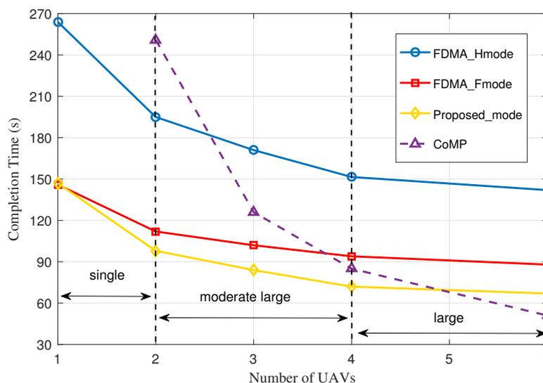
Figure 11. The completion time versus the number of UAVs under different schemes.
