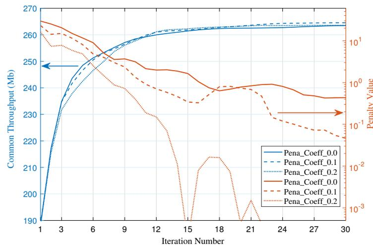
Figure 7. Convergence results of the proposed algorithm with different penalty coefficients.
