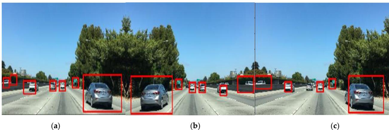
**Figure 16.** Confidence level effect. (a) Confidence = 0.85, the detection windows are too large to contain unnecessary information like the 2nd window from left (b) Confidence = 0.88, the detection windows are appropriate and contain the vehicles without omission (c) Confidence = 0.90. The 2nd car from left is not detected since confidence is too high.
