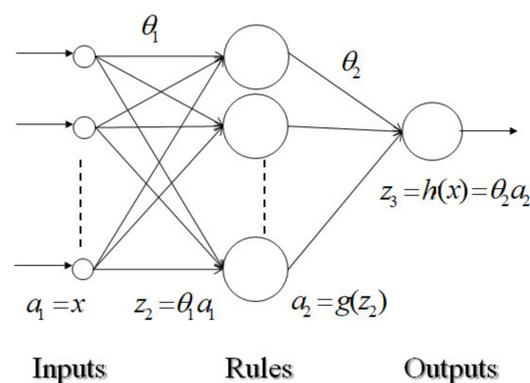
Figure 1. The schema of the fuzzy logic model.
