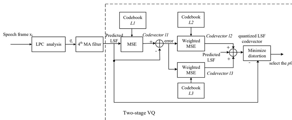
Figure 1. Structure of the two-stage vector quantization (VQ) for line spectrum frequency (LSF) coefficients.
