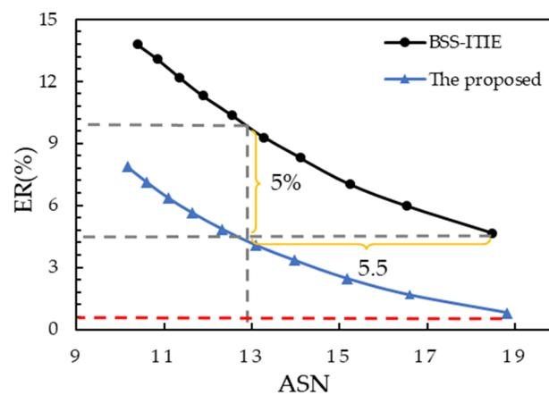
**Figure 6.** Comparison of the ER and ASN between the BSS-ITIE [28] method and the proposed algorithm.
