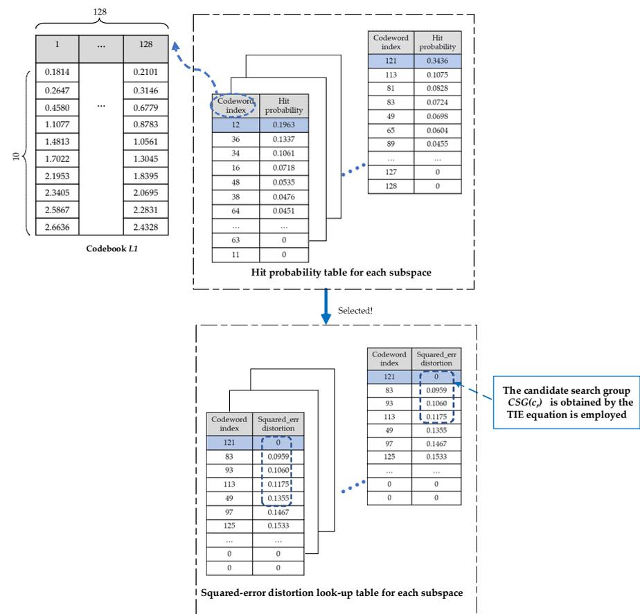
**Figure 3.** The squared-error distortion look-up table is designed for each subspace.
