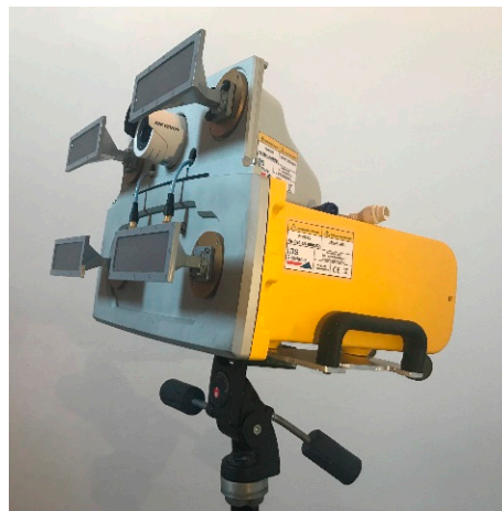
Figure 5. IBIS-FM MIMO Radar by IDS Company in the configuration with four antennae connected.
