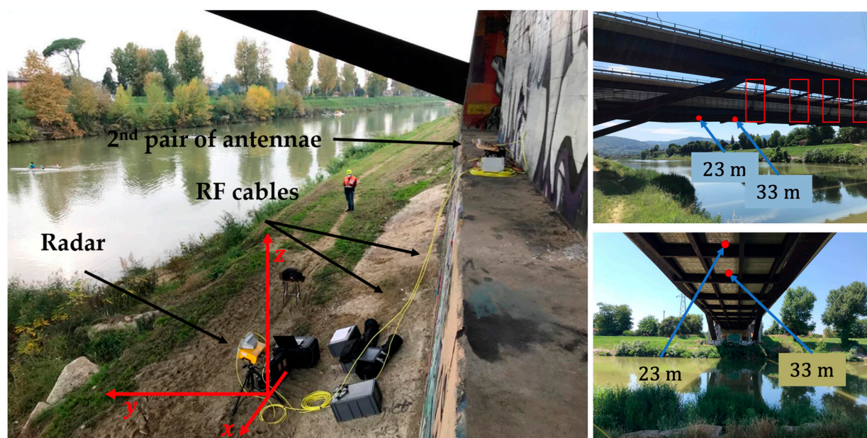
Figure 11. Geometry of the experimental setup during the “Vurlungo” monitoring campaign. The red dots indicate the targets selected for analysis. The point at 23 m is Target A and the point at 33 m is Target B. The squares indicate the steel stays that connect the bridge to the carriageway.
