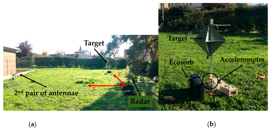
Figure 7. (a) Geometry of the experimental setup in a controlled environment; (b) detail of the target used during the controlled environment experimental session.
