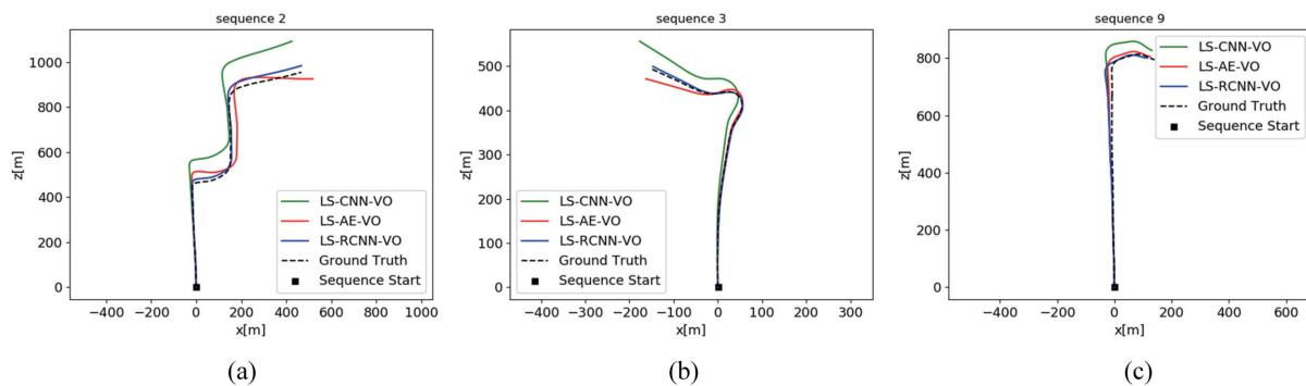
**Figure 9.** Comparison of the moving trajectories detected by the three models with the ground truth for sequence 02 (a), 03 (b), and 09 (c) of Malaga dataset.
