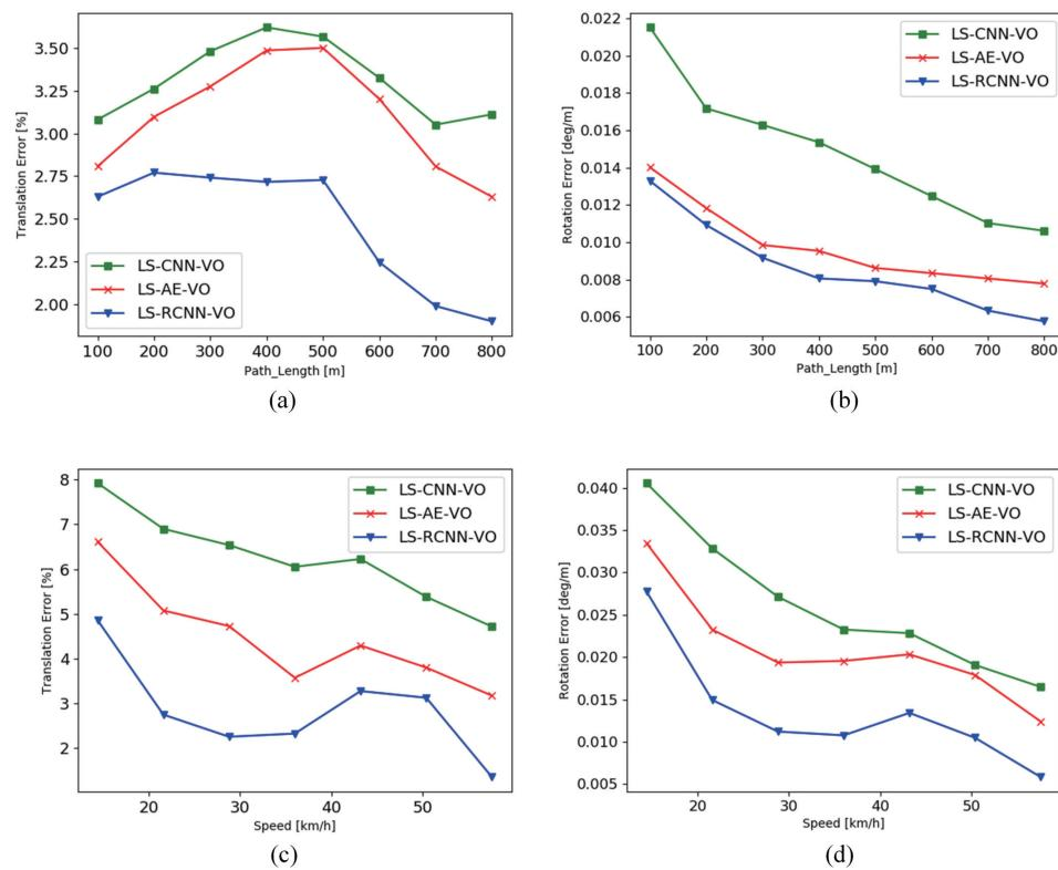
**Figure 6.** Comparison of the average translation error (ATE) and the average rotational error (ARE) of the three models at different path lengths and speeds on KITTI dataset. (a) ATE versus path length, (b) ARE versus path length, (c) ATE versus speed, and (d) ARE versus speed.
