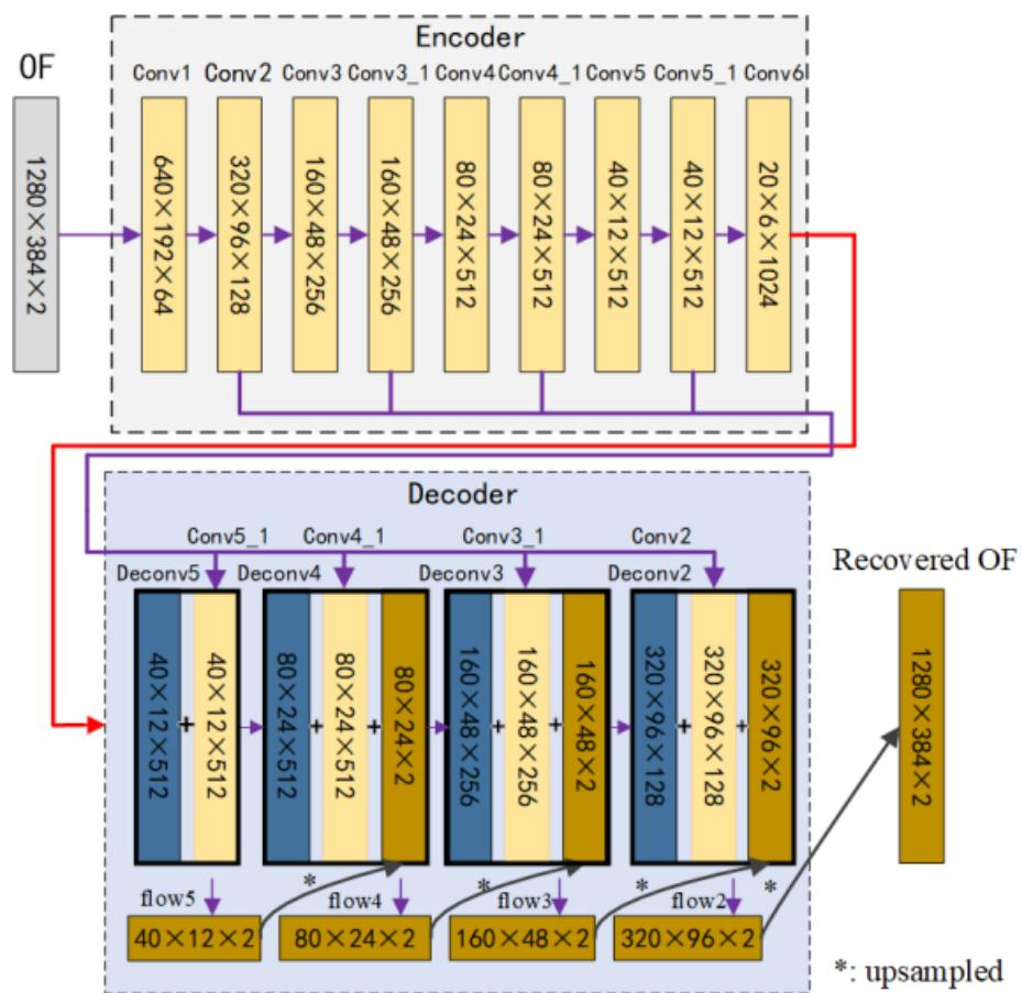
**Figure 2.** The process of encoding and decoding.
