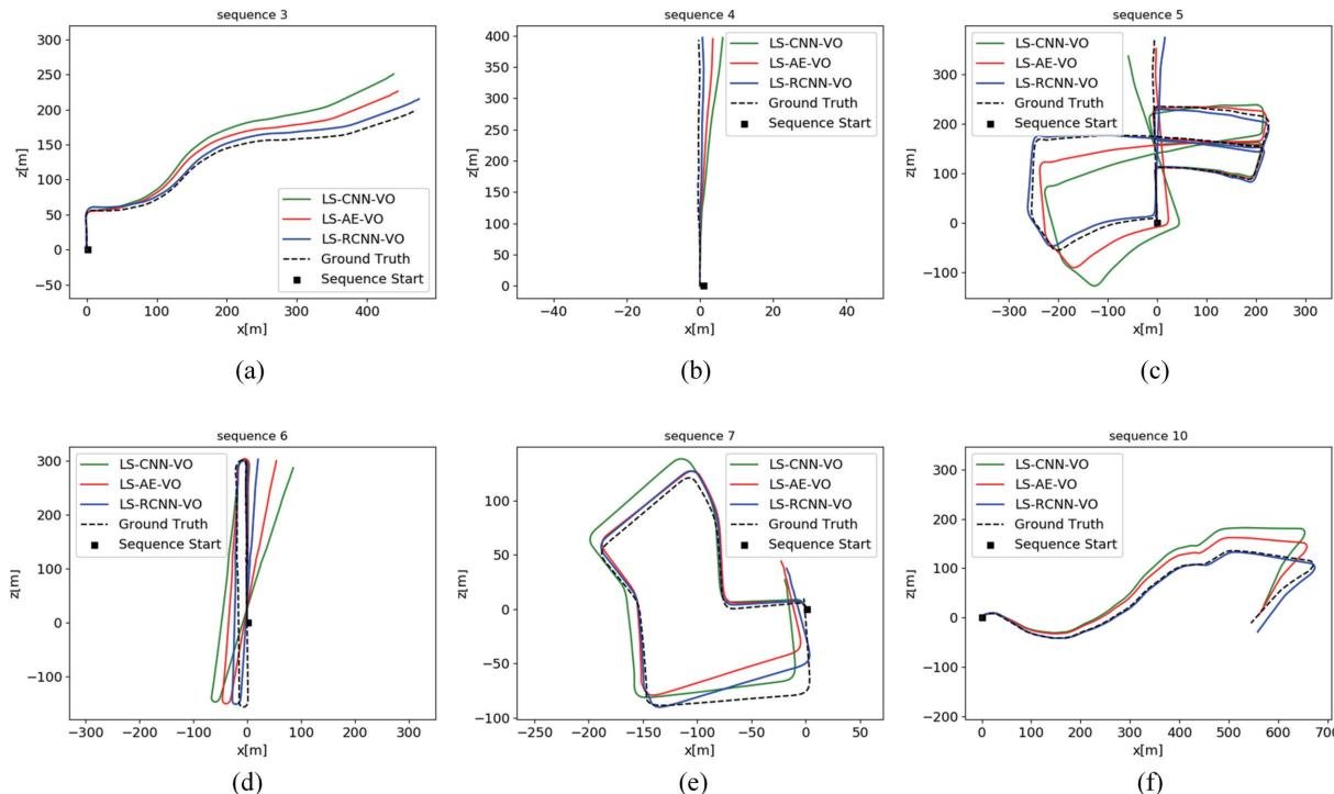
**Figure 8.** Comparison of the moving trajectories detected by the three models with the ground truth for sequence 03 **(a)**, 04 **(b)**, 05 **(c)**, 06 **(d)**, 07 **(e)**, and 10 **(f)** of KITTI dataset.
