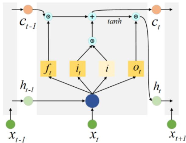
**Figure 3.** The internal structure of an Long Short-term Memory (LSTM) unit where  $\odot$  and  $\oplus$  denote element-wise product and addition of two vectors, respectively.
