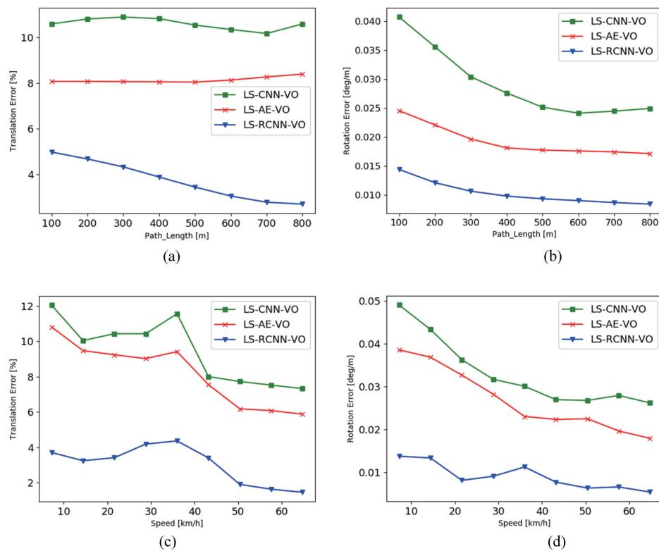
**Figure 7.** Comparison of the ATE and the ARE of the three models at different path lengths and speeds on Malaga dataset. **(a)** ATE versus path length, **(b)** ARE versus path length **(c)** ATE versus speed, and **(d)** ARE versus speed.
