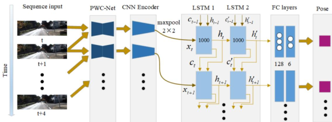
**Figure 5.** The architecture of LS-RCNN-VO model in its end-to-end form.
