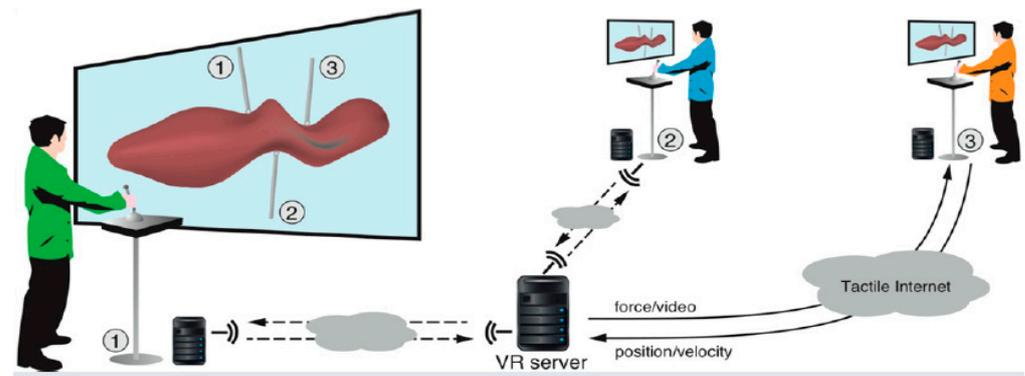
Figure 12. Physical coupling of several users via VR simulation with haptic feedback [13].
