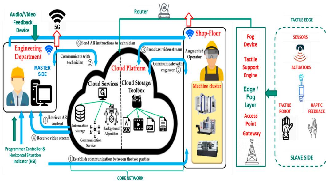
**Figure 17.** Integrating 5G and TI applications for integrated and adaptive AR maintenance and shop-floor rescheduling (adapted from [59]).
