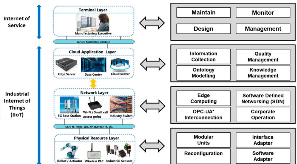
Figure 19. Hierarchical architecture of a smart factory (adapted from [71]).
