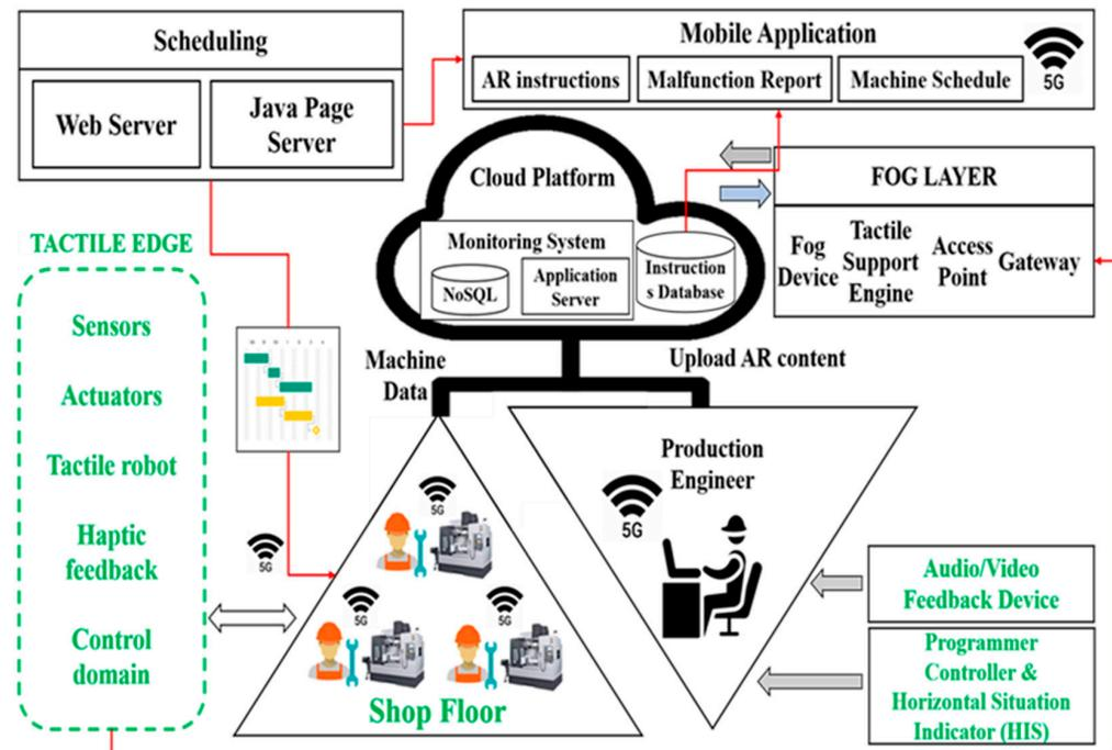
**Figure 16.** Integrating 5G and TI applications for integrated and adaptive AR maintenance and shop-floor rescheduling (adapted from [67]).
