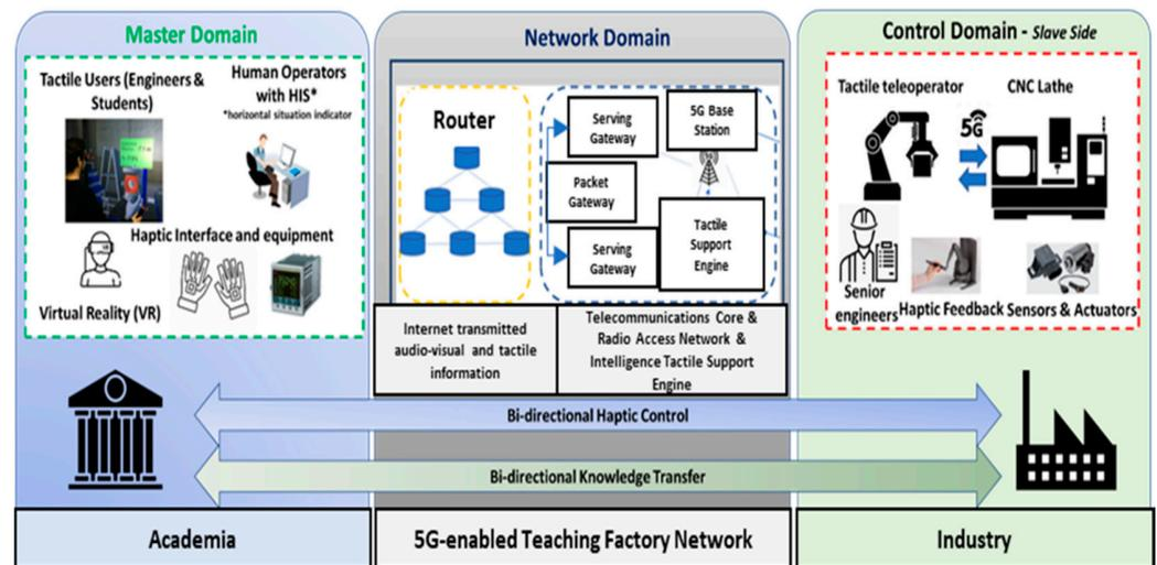
Figure 18. A generalized architecture of a wireless tactile internet system in a teaching factory [69].
