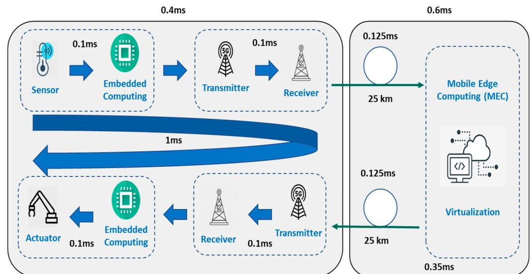
Figure 9. The various latency components of a typical TI system [41].
