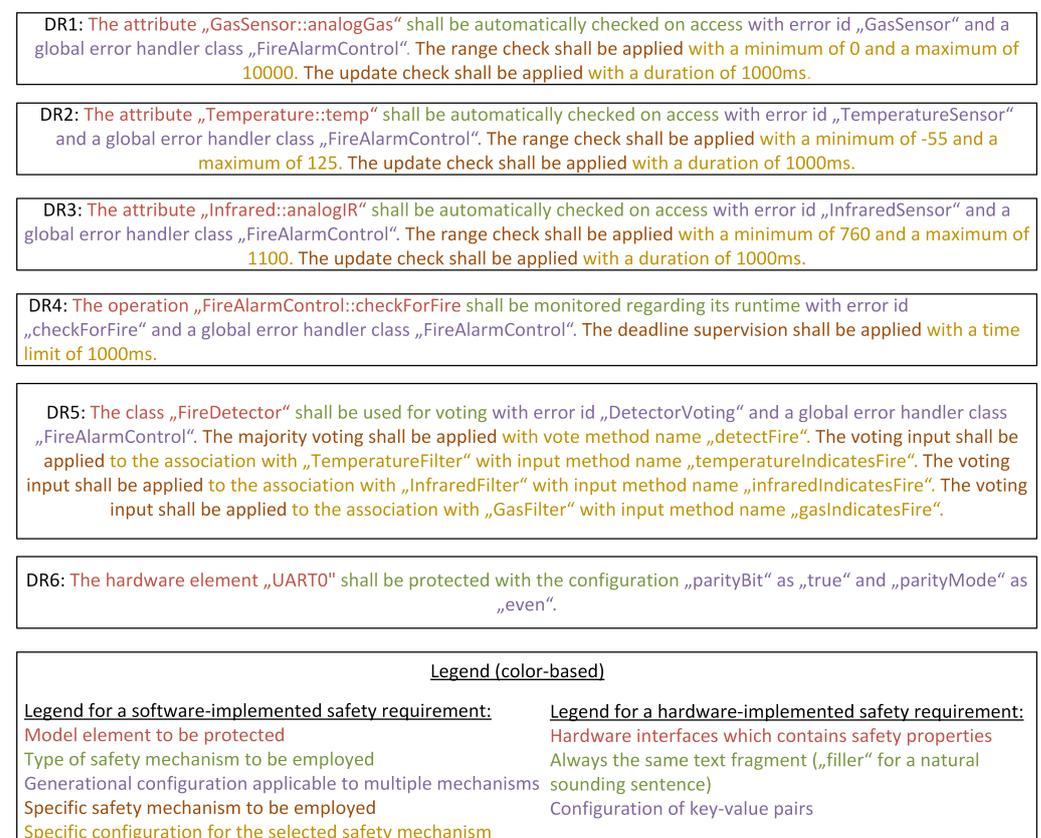
**Figure 3.** Derived safety requirements for the application example.
