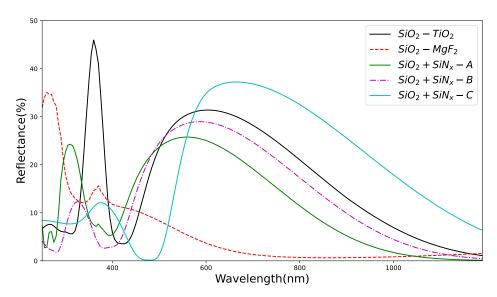
Figure 4. Reflectance spectra as a function of wavelength for some double-layer anti-reflection coating.
