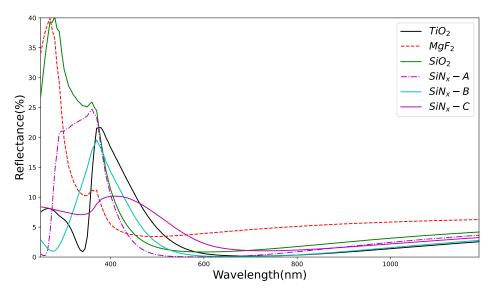
**Figure 3.** Reflectance spectra as a function of wavelength for some optimised single-layer antireflection coating.
