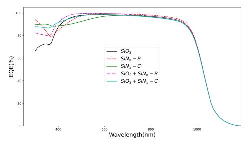
Figure 6. EQE measurement carried on selected ARC layers.
