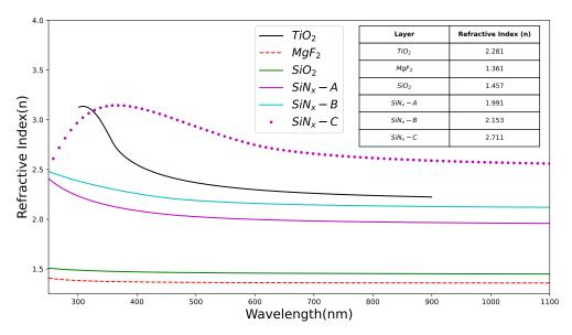
Figure 2. Refractive indices of various ARC layers.
