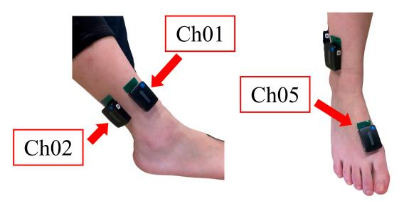
**Figure 2.** Ch01 is sensor 1 placed on the surface where the EDL muscle is located. Ch02 is sensor 2 placed on the surface where the soleus muscle is located. Ch05 is the accelerometer placed on the dorsum of the foot between the first and second metatarsals.
