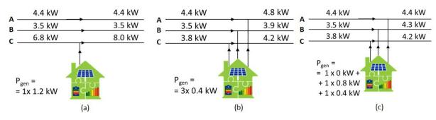
**Figure 1.** The approach used by the PSM algorithm for loss minimization: (**a**) unbalanced one-phase injection, (**b**) three-phase balanced injection, (**c**) unbalanced three-phase injection.
