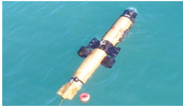
Figure 1. Torpedo-shaped vehicle and the thrusters' configuration.
