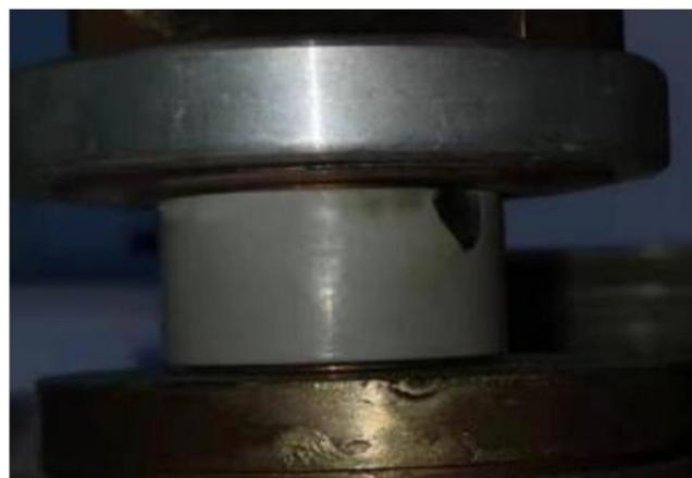
**Figure 7.** Surface breakdown of a varistor under a high current impact.
