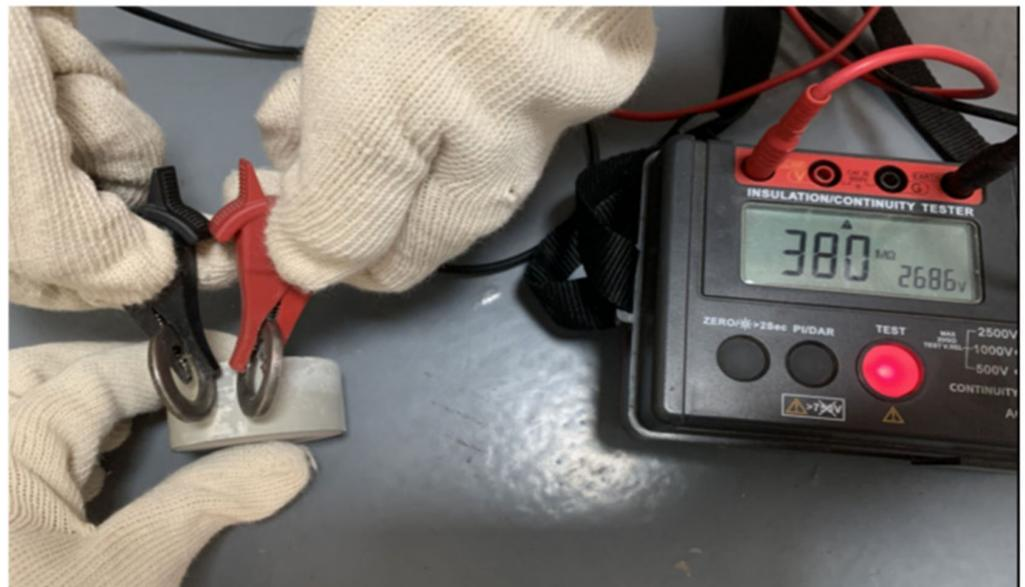
Figure 10. Insulation resistance test.
