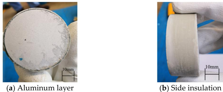
**Figure 5.** Typical appearance of a defective arrester varistor.
