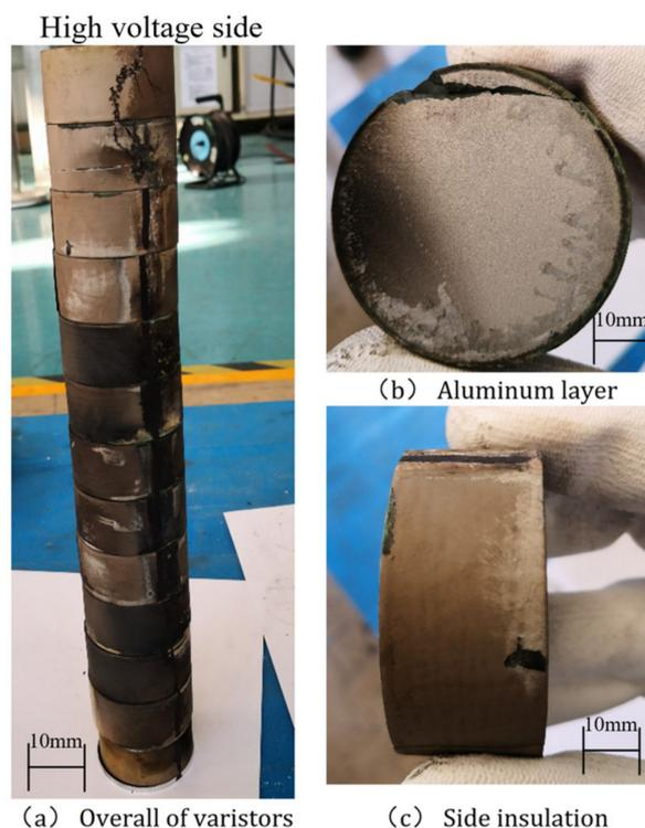
**Figure 6.** Typical appearance of a defective arrester varistor.
