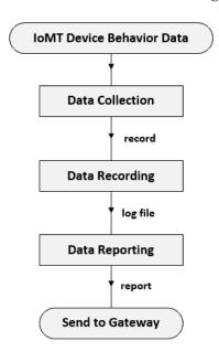
Figure 4. The monitoring and data acquisition (MDA) component.
