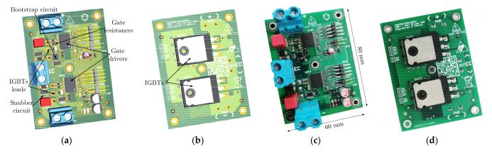
**Figure 11.** Developed HB cell: (a) 3D model, top view; (b) 3D model, bottom view; (c) implemented prototype, top view; (d) implemented prototype, bottom view.
