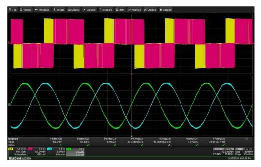
**Figure 16.** Experimental results of voltage and current at the output of the modular three-phase VSI, steady state (50 V/div, 2 A/div, 10 ms/div).
