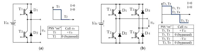
Figure 1. The most common power cells and their voltage levels: (a) HB cell; (b) FB cell.
