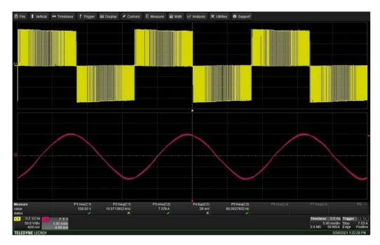
**Figure 15.** Experimental results of voltage and current at the output of the modular single-phase VSI, steady state (50 V/div, 5 A/div, 5 ms/div).
