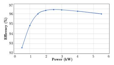
Figure 18. Efficiency curve of the power stage of a FB VSI for an input voltage of 180 V in DC-link.
