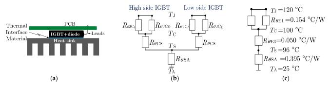
Figure 10. (a) IGBT+diode on the heat sink; (b) thermal resistance circuit and (c) parameters of the thermal circuit.
