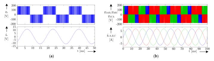
**Figure 12.** Simulated results of voltage and load current at the output of the inverter with open loop SPWM and in steady state; (**a**) single-phase FB VSI; (**b**) three-phase VSI.
