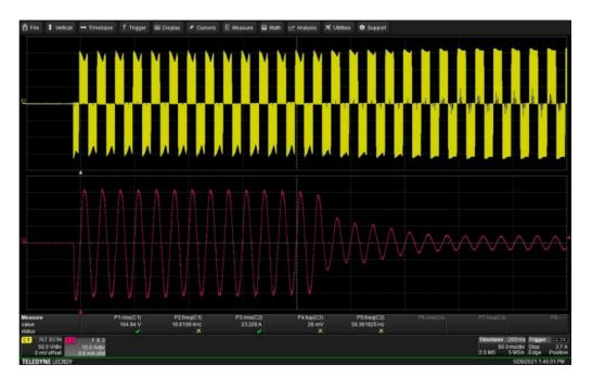
**Figure 14.** Experimental results of voltage and current at the output of the modular single-phase FB VSI, in dynamic state (50 V/div, 10 A/div, 50 ms/div).
