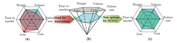
**Figure 4.** Power electronics performance trends: (**a**) achievable performance using state-of-the-art technology (blue) and performance limits due to physical barriers (red), (**b**) improvements over time, (**c**) expected performance (green).
