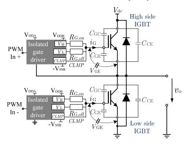
Figure 7. HB cell with basic push-pull resistive gate drives and parasitic capacitances of the IGBTs.
