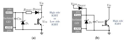
Figure 8. (a) Desaturation circuit; (b) Bootstrap.
