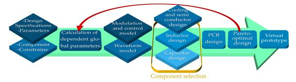
Figure 5. Simplified workflow of the virtual prototyping routine of the MODO-based process.
