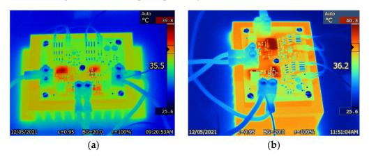
**Figure 17.** Temperature distribution of an HB cell with 50% of the nominal load: (**a**) after 30 min of operation; (**b**) after 3 h of operation.
