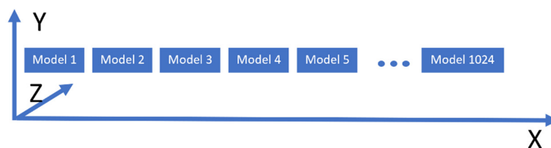
Figure 5. Overview of the work group layout of the compute shader used to calculate the switching criterion, with \text{local\_size\_x} = 1024 , \text{local\_size\_y} = \text{local\_size\_z} = 1 . Each box represents an instance of the data structure associated with a nominal model used to pass information to and from the GPU.
