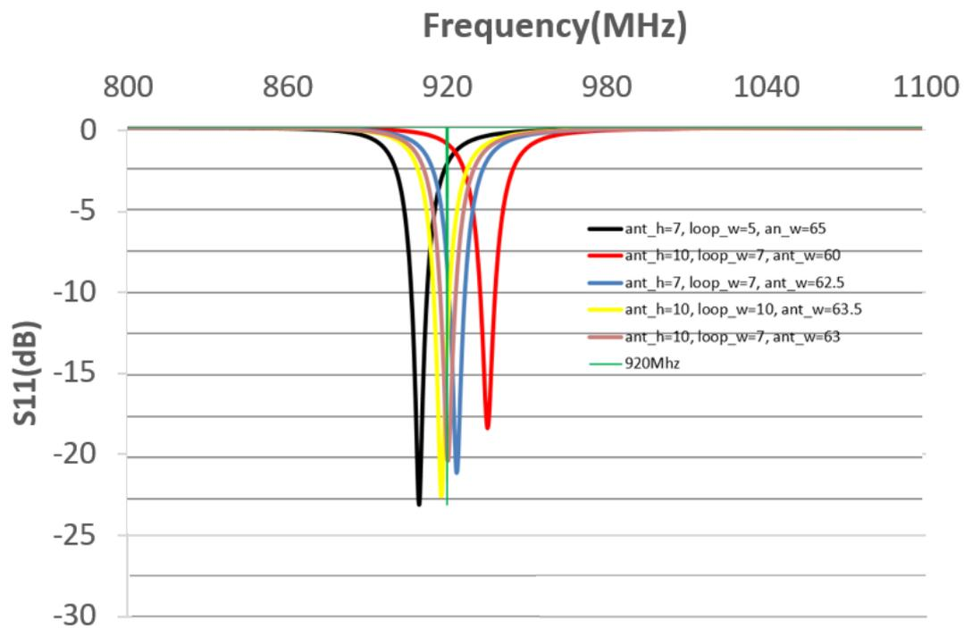
Figure 7. Optimization using parameter sweep S11 (dB) vs. frequency (GHz).
