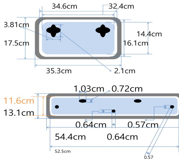
**Figure 1.** Size of a typical license plate holder. [26].
