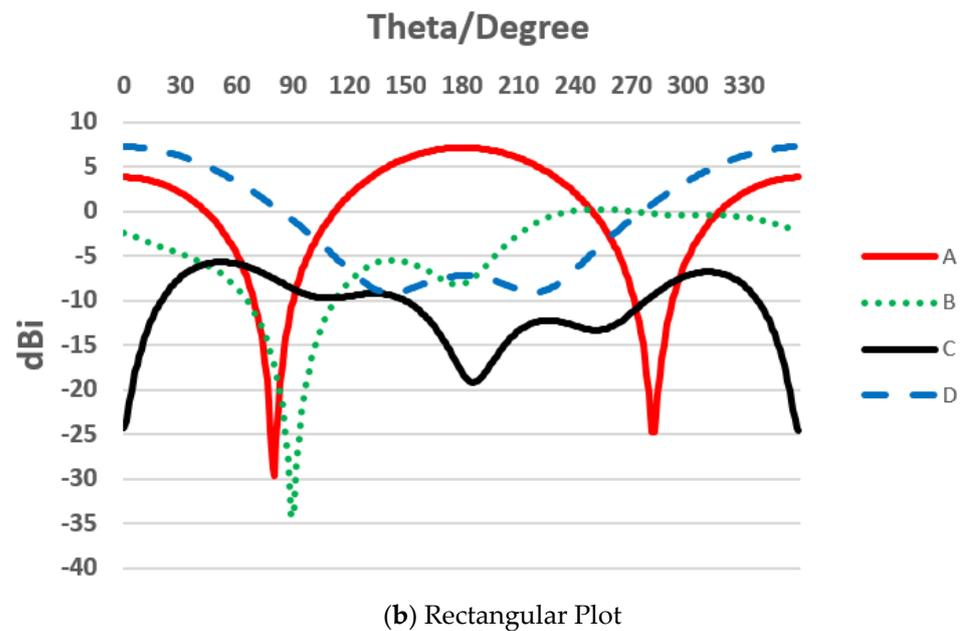
Figure 4. Radiation pattern of tag antenna.
