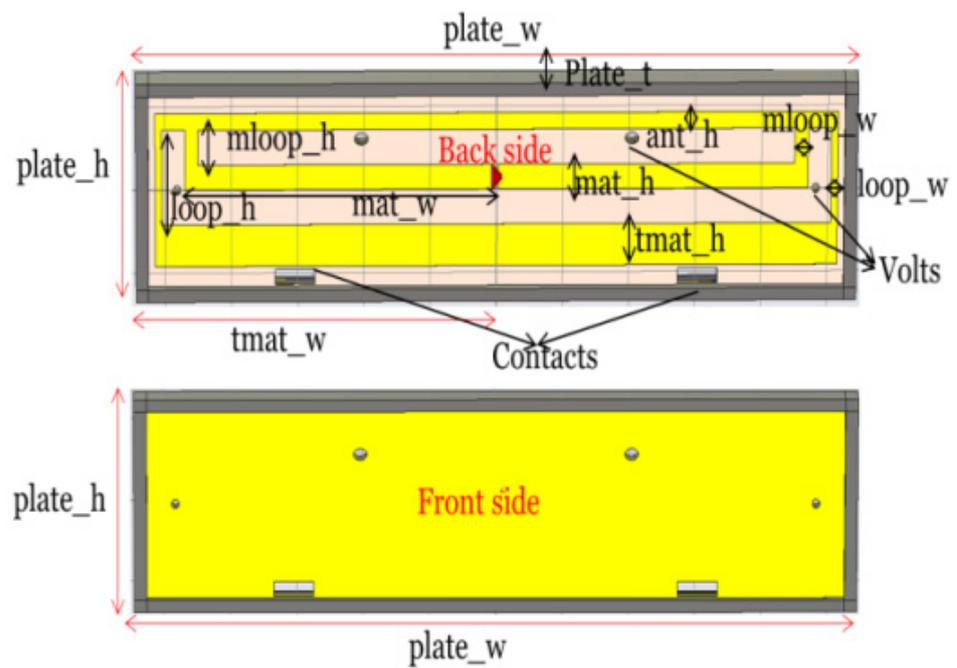
Figure 2. Parameters and design structure of the RFID tag antenna without bumper.
