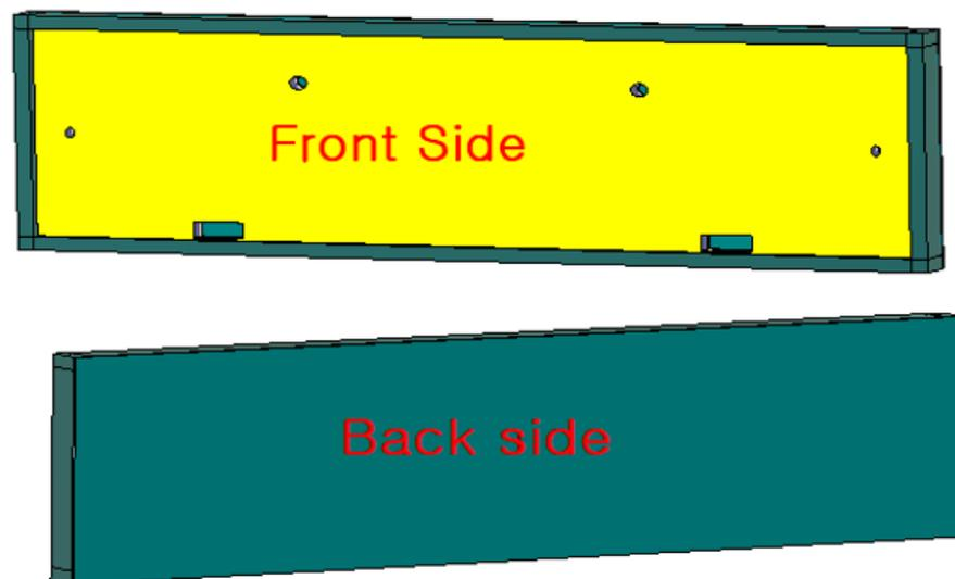
Figure 3. Front and back side of license plate RFID tag antenna with bumper.
