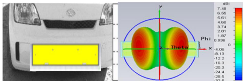
Figure 5. The three-dimensional radiation pattern of the tag antenna at 920 MHz.
