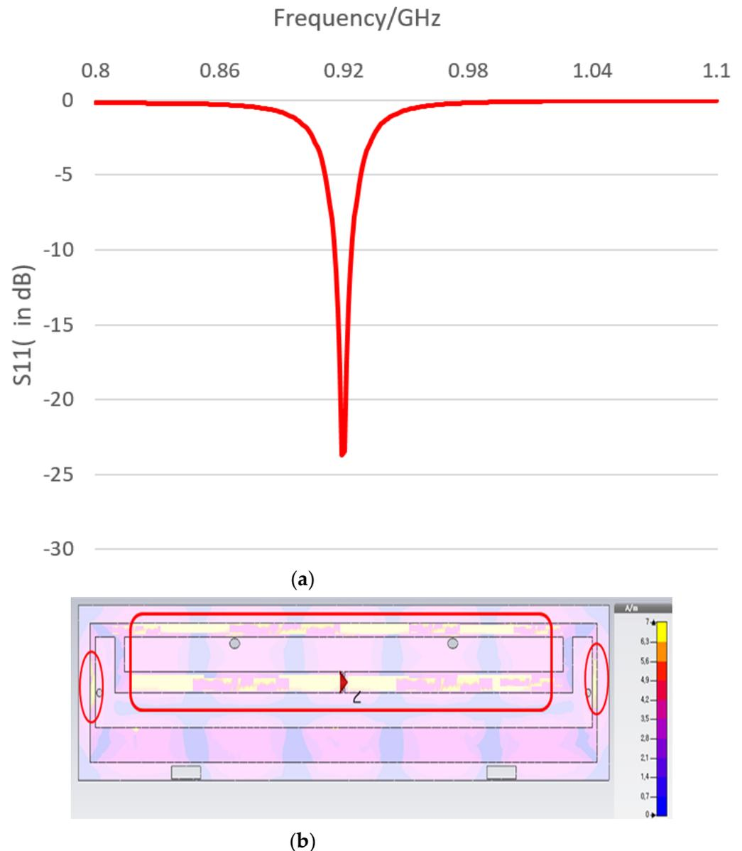
**Figure 6.** (a) Simulated return loss of tag antenna at 920 MHz. (b) Current density of the tag antenna at 920 MHz.
