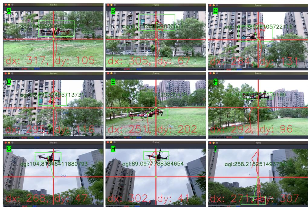
**Figure 17.** Airborne Object target Tracking (AOT) (drone to drone tracking).
