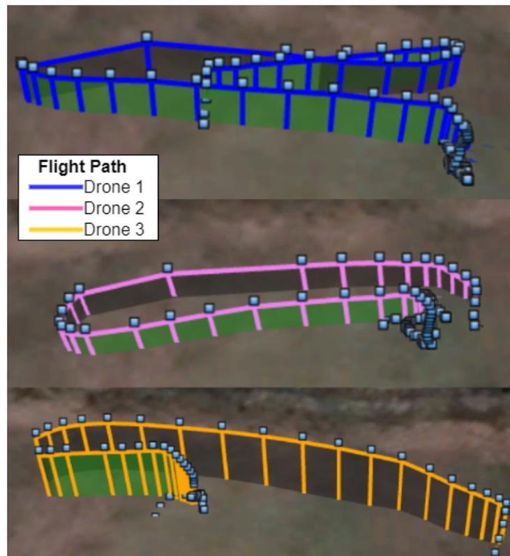
Figure 15. Individual drone flight paths were logged during the test flight and depicted using the Google Earth application.
