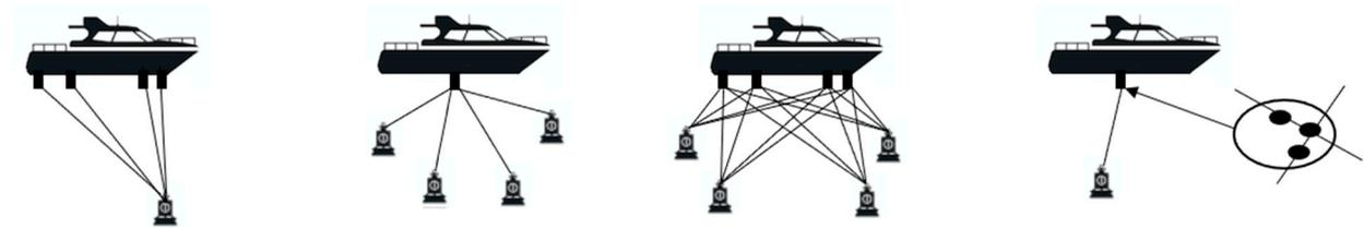
**Figure 1.** Primary Types of Acoustic Positioning System, created based on Keith Vickery's ACOUSTIC POSITIONING SYSTEMS "A PRACTICAL OVERVIEW OF CURRENT SYSTEMS" <https://dynamic-positioning.com/proceedings/dp1998/SVickery.PDF>, accessed on 25 August 2021) using graphics designed by macrovector/FreePik.
