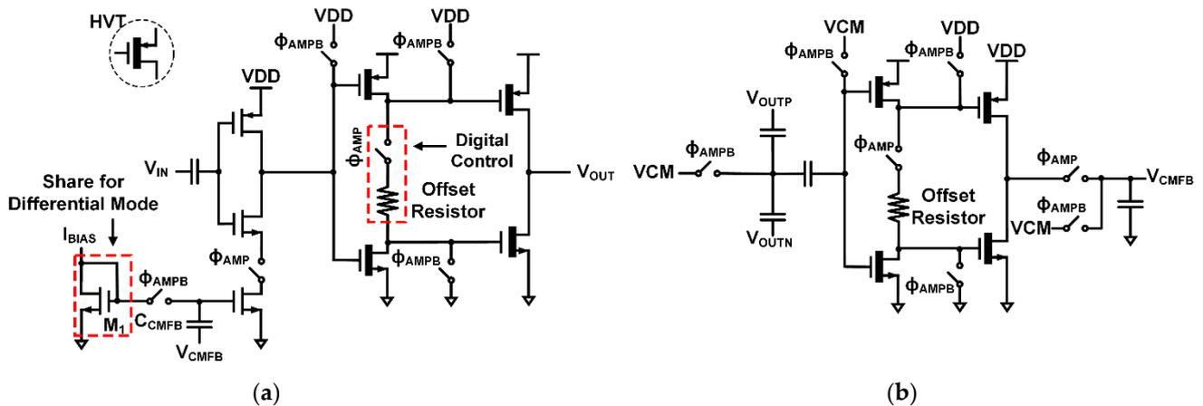
Figure 6. (a) The proposed ring amplifier structure in the single-ended mode. (b) The CMFB circuit with a single loop.
