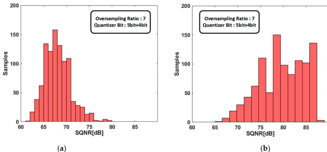
**Figure 3.** The SQNR histogram for different open-loop gain of inter-stage amplifier with 5% variation and no filter calibration: (a) the open-loop gain of 40 dB and (b) the open-loop gain of 60 dB.
