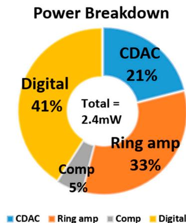
Figure 16. The power consumption breakdown of the proposed ADC.
