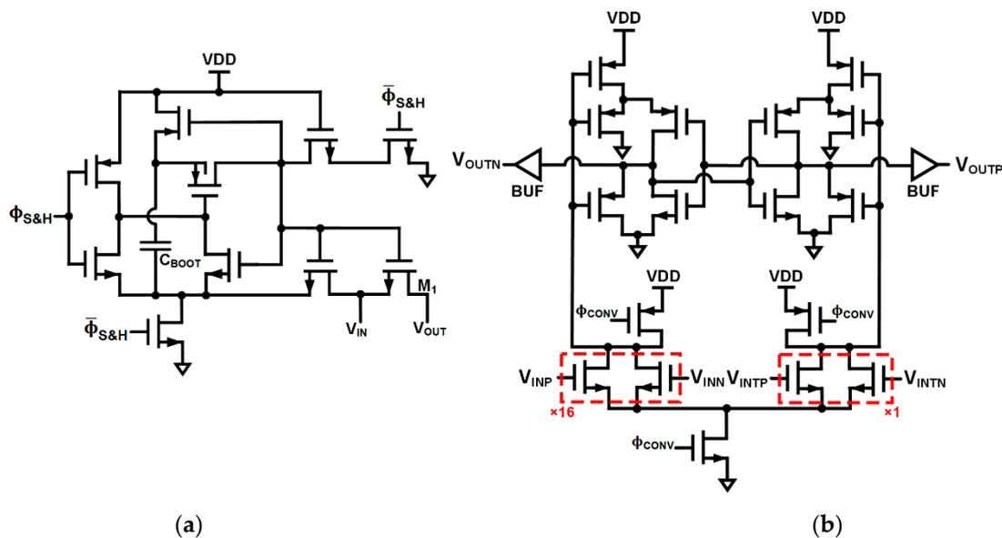
Figure 11. The schematic of (a) the bootstrap switch and (b) the multi-input two-stage dynamic comparator.
