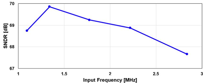
Figure 15. The measured SNDR versus input frequency.
