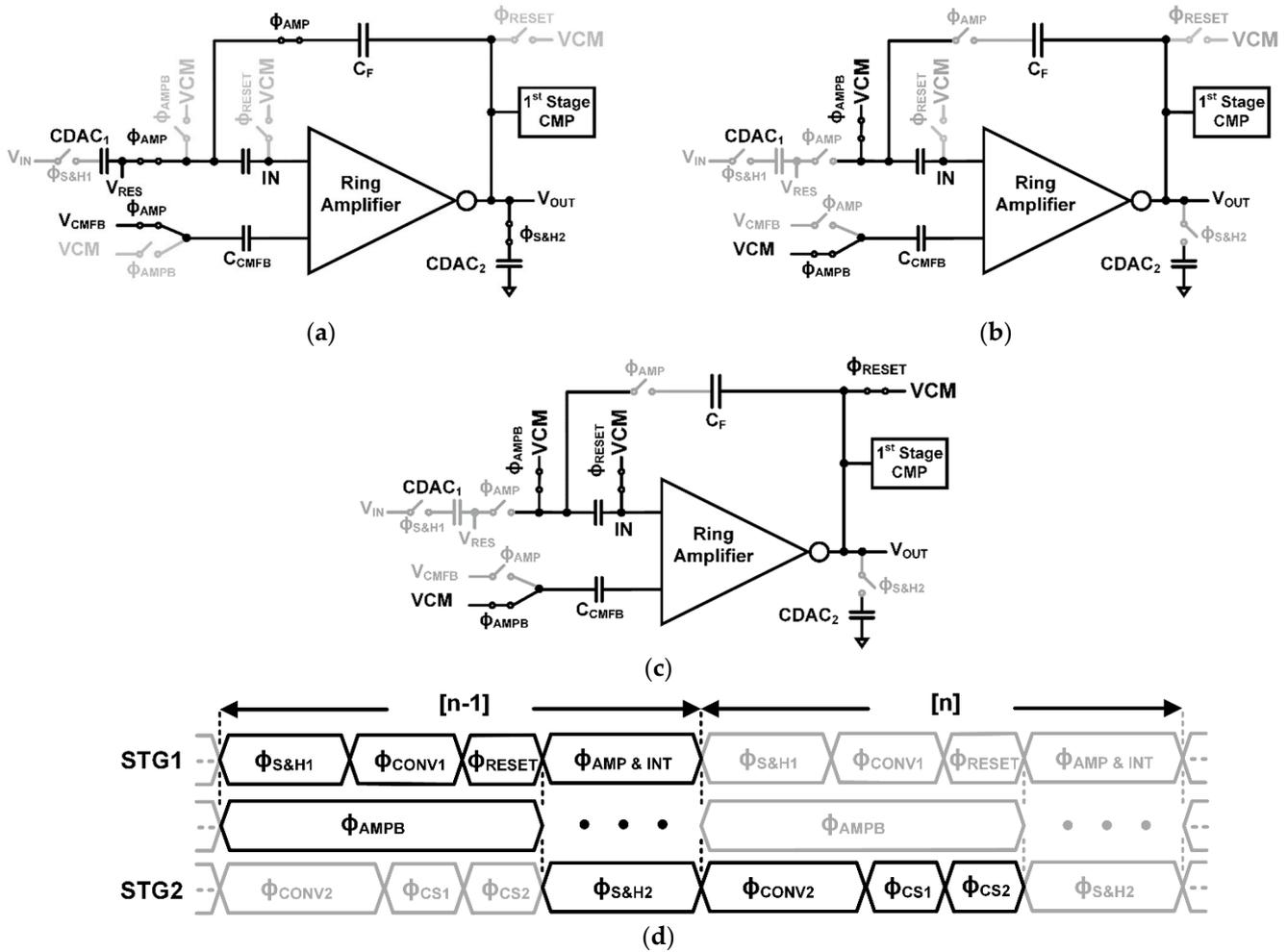
Figure 9. The ring amplifier-based integrator and its three phases of (a) amplification, (b) nonamplification without reset, and (c) nonamplification with reset; and (d) the operation timing diagram.
