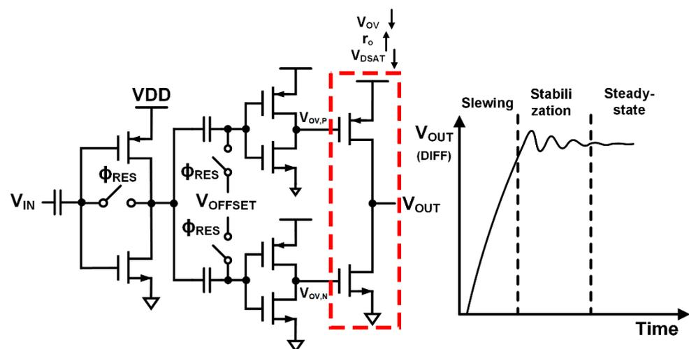
**Figure 5.** The conventional ring amplifier structure with three inverters (single-ended view) and its transient response (differential mode).
