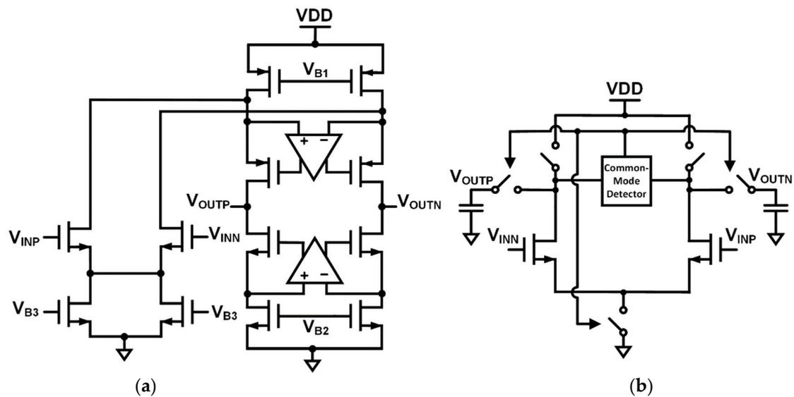
**Figure 4.** The implementation of inter-stage gain using (a) the folded cascode op-amp in closed-loop and (b) the dynamic amplifier in open-loop.
