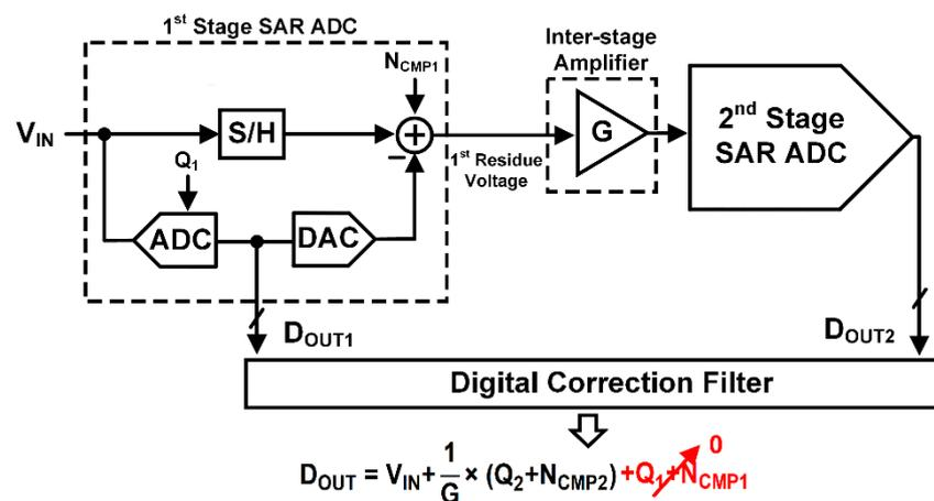
**Figure 1.** The conventional pipelined SAR ADC block diagram.
