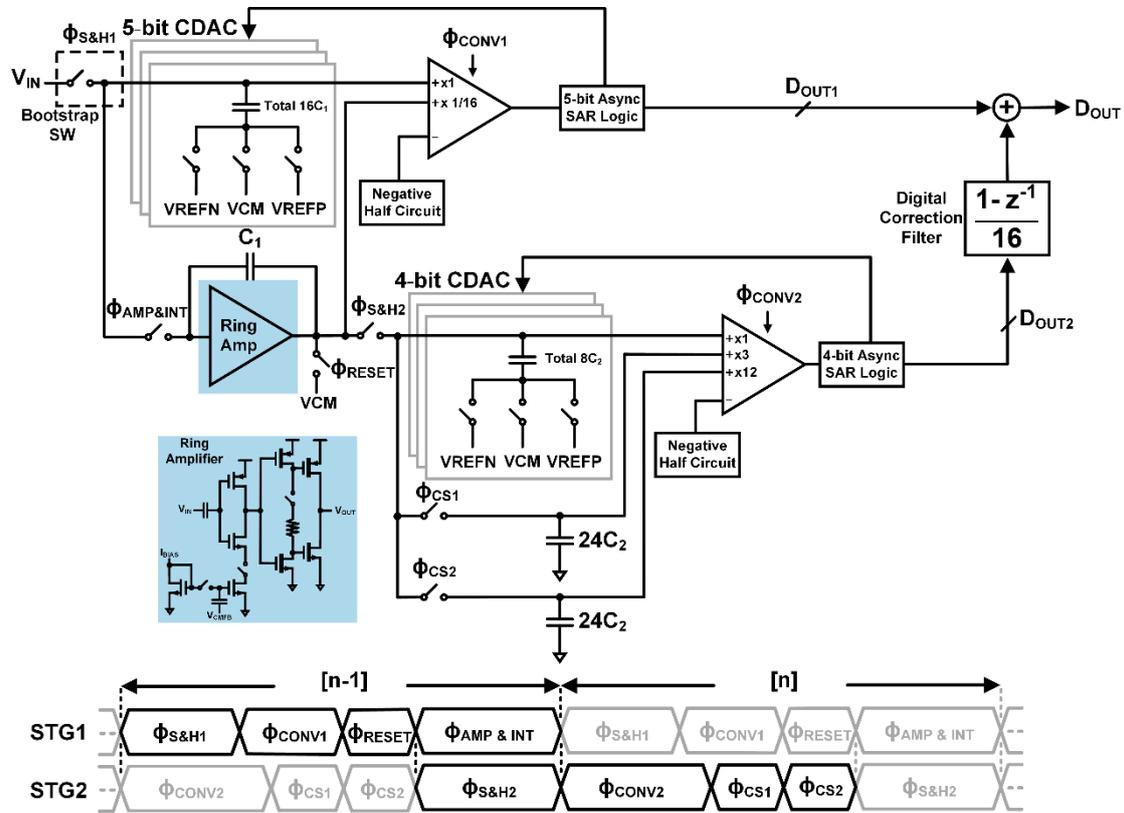
Figure 10. The circuit implementation of the proposed ADC and its operation timing diagram.
