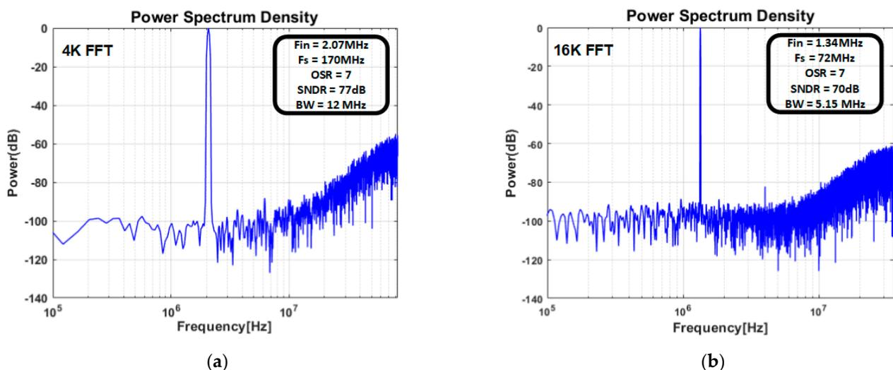
Figure 14. The output power spectral density without filter calibration from (a) the post layout simulation and (b) the measurement.
