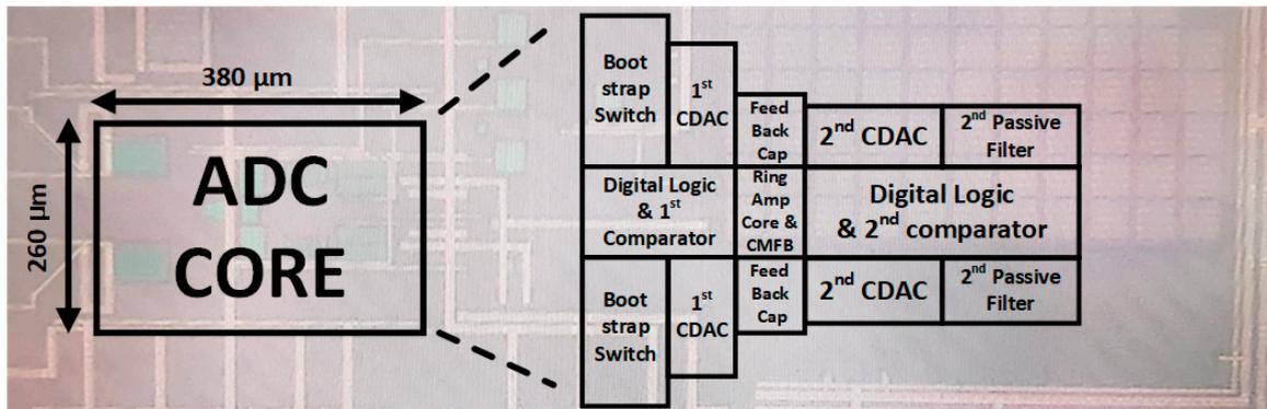
Figure 12. The die photograph of the ADC core.
