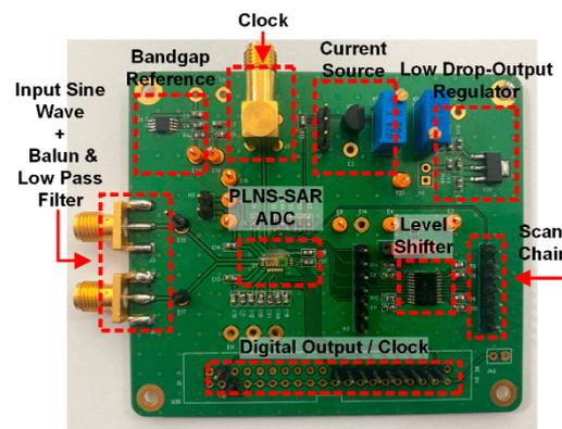
Figure 13. The evaluation board for the proposed ADC prototype.
