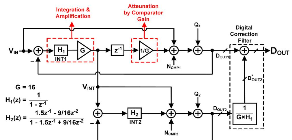
**Figure 2.** The pipelined noise-shaping SAR ADC block diagram.
