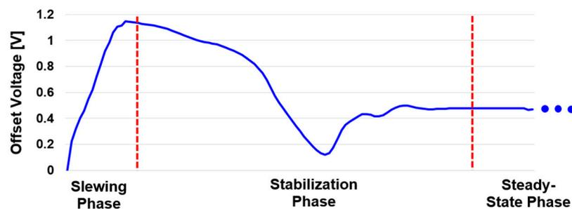
Figure 7. The transient of the offset voltage during amplification.
