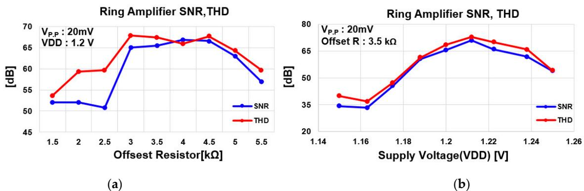
Figure 8. The SNR and THD of ring amplifier versus (a) the offset resistor and (b) the supply voltage.
