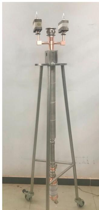
**Figure 13.** Prototype of the W-band TE<sub>02</sub> mode gyro-TWT.
