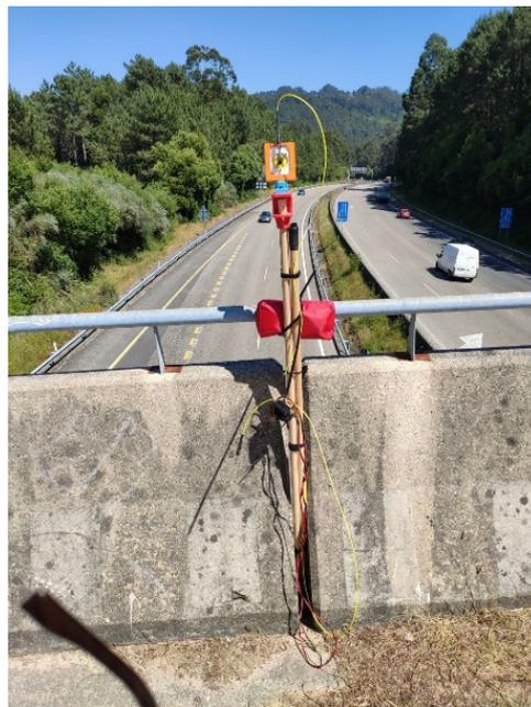
Figure 10. Transmitting antenna placed over the highway.
