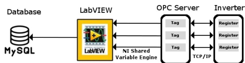
Figure 12. The software components of the monitoring system.
