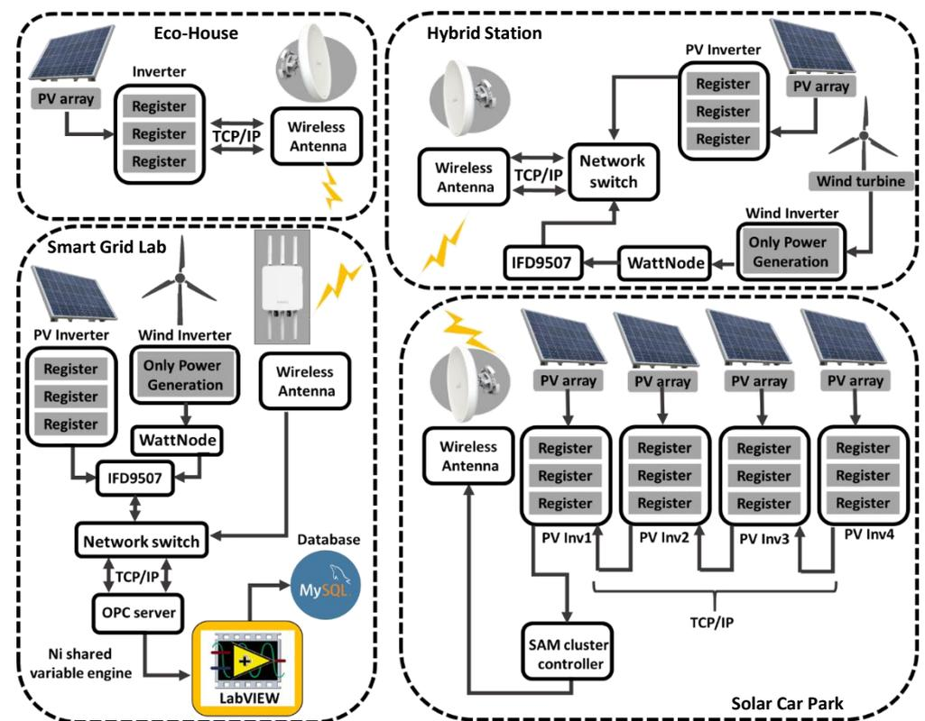
**Figure 8.** The layout of the real-time monitoring system. Notice that only the Smart Grid Lab and Hybrid Station include a wind turbine in their DERs. All locations communicate with the server through a bidirectional communication channel.
