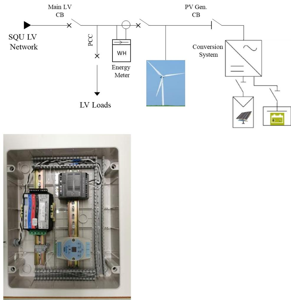
**Figure 11.** The Hybrid Station. The top figure shows the single line diagram of PV-Battery, while the bottom figure shows how the WattNode and IFD9507 converter are interfaced to the hybrid inverter.
