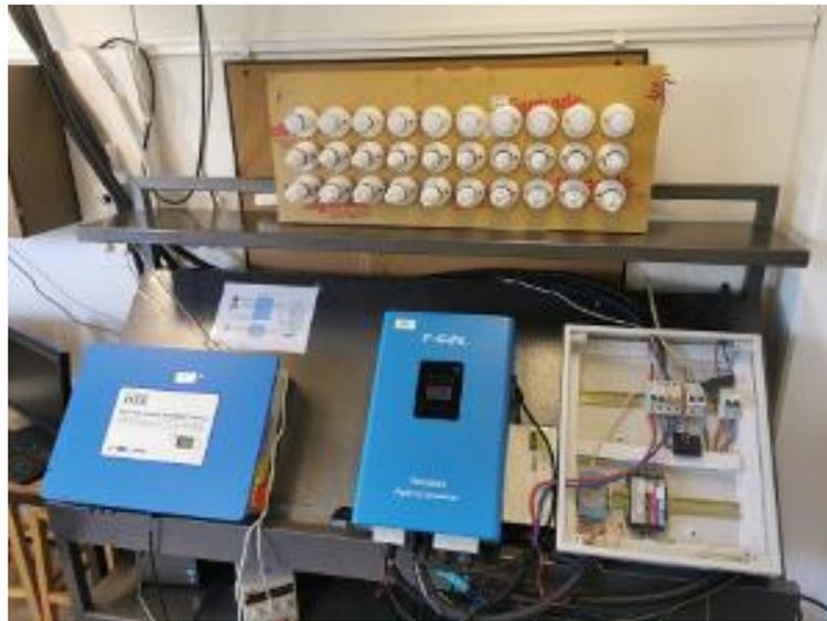
**Figure 9.** System implementation at the Smart Grid Lab. The top figure shows a block diagram of the system, while the bottom shows the actual implementation in the lab.
