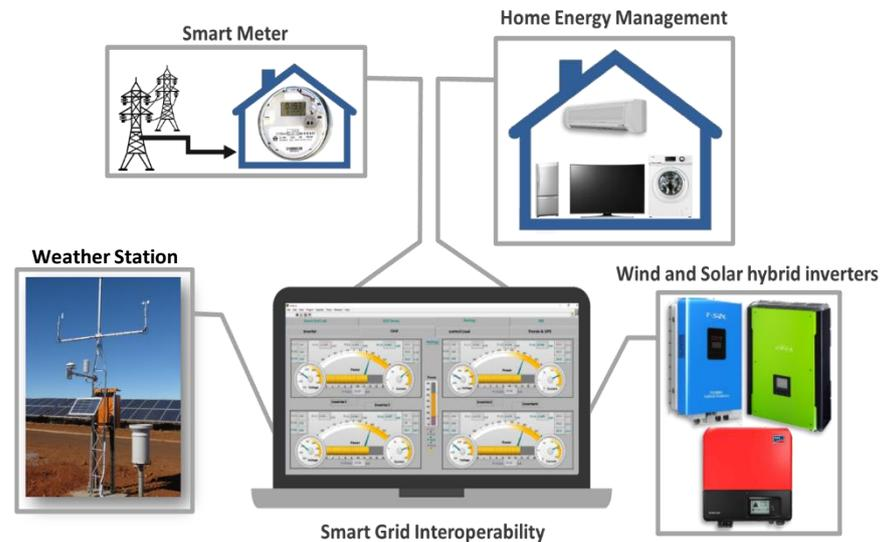
**Figure 2.** An RES monitoring system. The monitoring system collects and logs data from solar panels, wind turbines, storage batteries, inverters, smart meters, and an optional weather station.
