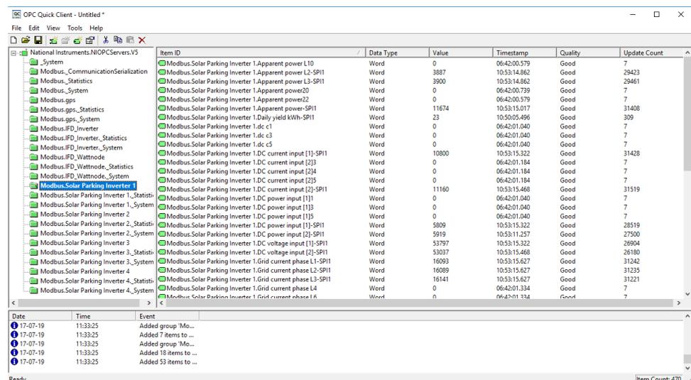
Figure 14. OPC Quick Client for debugging and troubleshooting.
