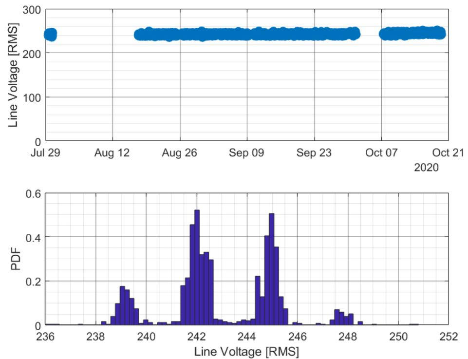
**Figure 21.** The line-to-neutral voltage at the Hybrid Station. Top plot: real-time measurements, Bottom: PDF of line voltage.
