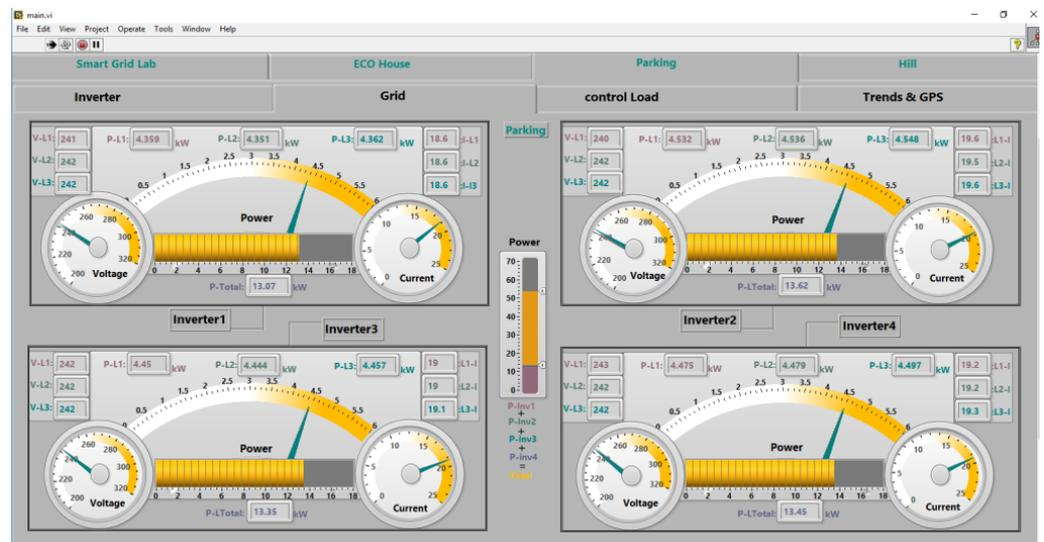
Figure 18. LabVIEW visualization of inverter’s AC-side quantities.
