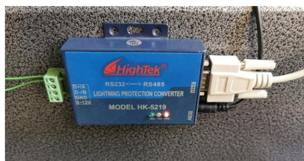
**Figure 6.** Connection of WattNode to the server via an RS232-to-RS485 converter.
