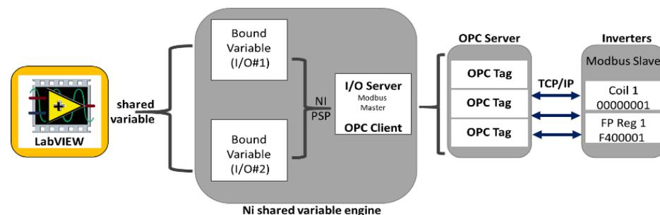
Figure 15. NI shared variable engine for connectivity between LabVIEW and OPC.
