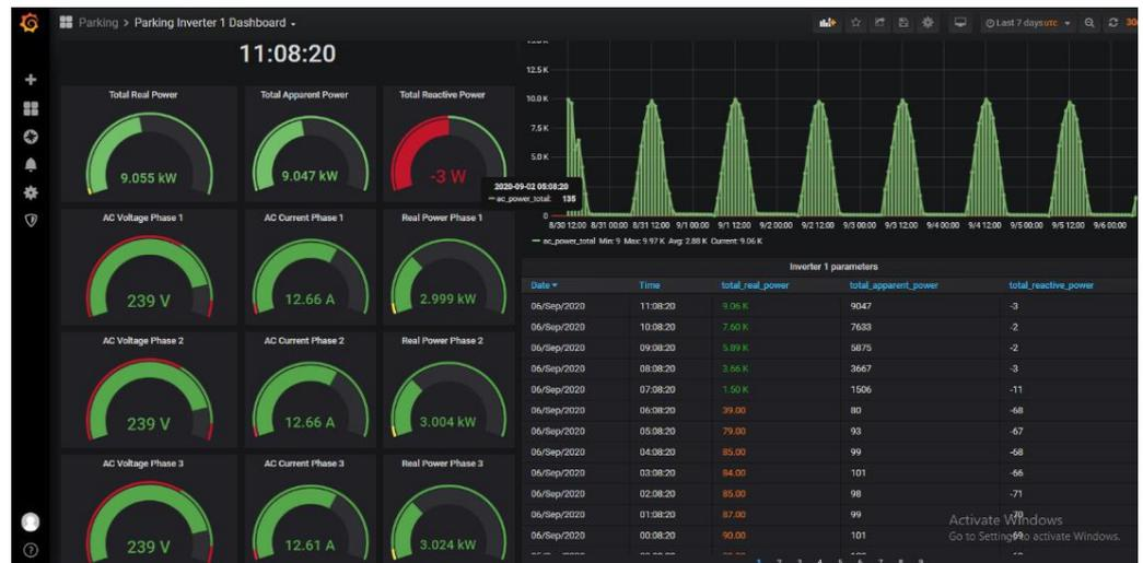
Figure 20. A Grafana dashboard that shows the parameters queried from the Solar Car Park DER.
