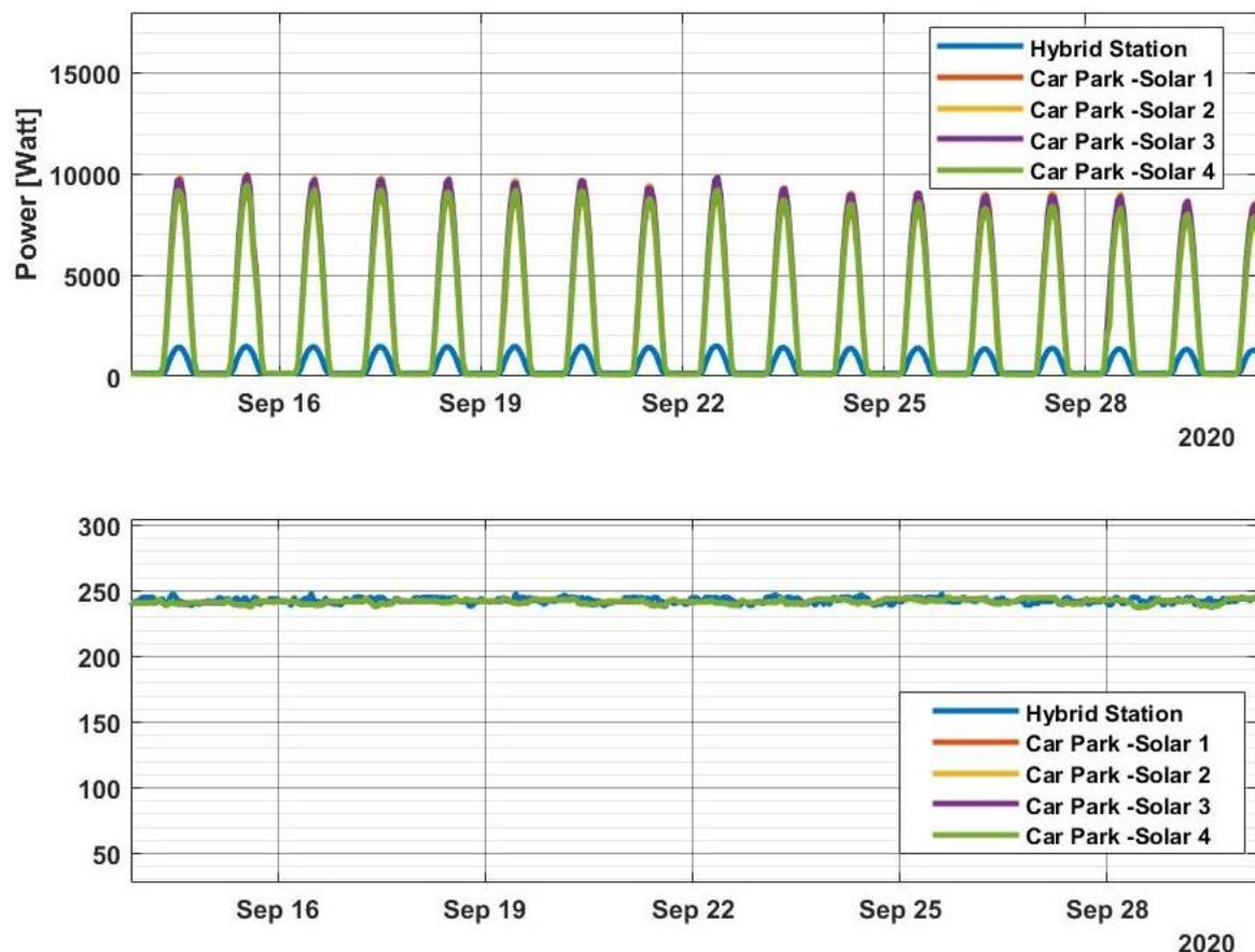
Figure 23. Power (top) and voltage levels (bottom) measured from the inverters at the Hybrid Station and Solar Car Park.
