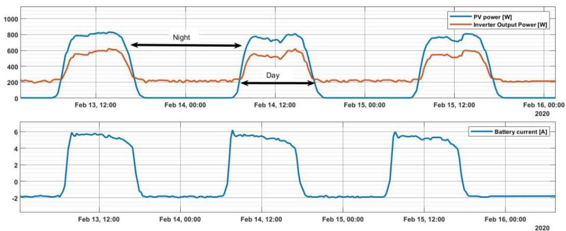
**Figure 22.** Microgrid PV system power and battery monitoring. The (top) plot shows the generated power from the PV panels and the output from the inverter. The (bottom) plot shows the current value on the battery side.
