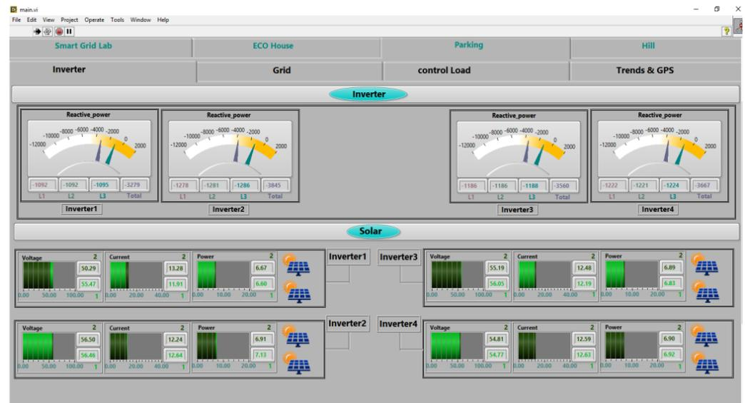
Figure 17. LabVIEW visualization of inverter’s DC-side quantities.
