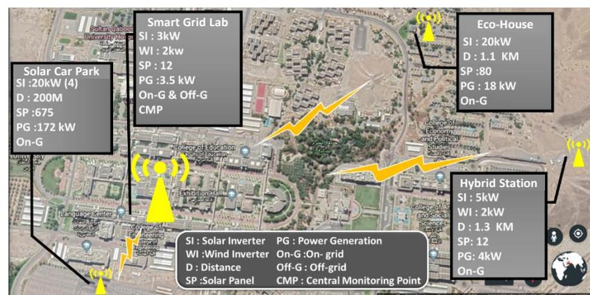
**Figure 1.** Locations of the renewable energy systems at the Sultan Qaboos University campus. The figure is annotated with information about Solar Inverters (SI), Wind Inverters (WI), Distance (D), Solar Panels (SP), Power Generation (PG), On-Grid (On-G), Off-Grid (Off-G), and Central Monitoring Point (CMP).
