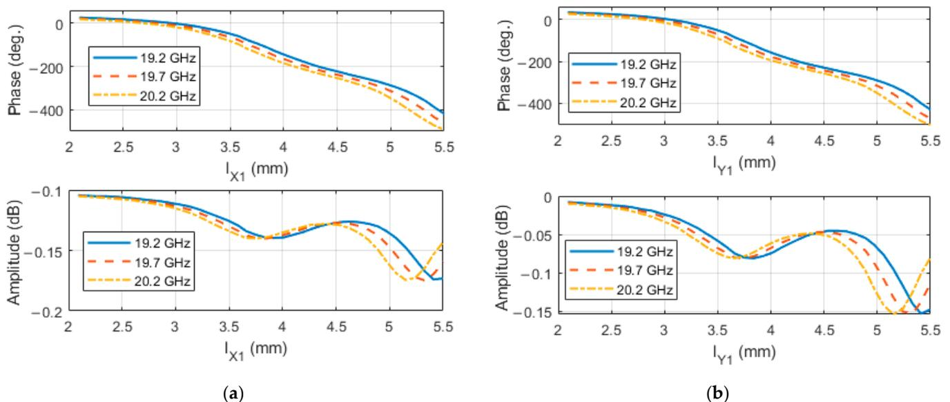
**Figure 5.** Phase and amplitude of the reflection coefficient associated with the (a)  $x$  component and (b)  $y$  component of the incident field, at several frequencies in the 20 GHz band.
