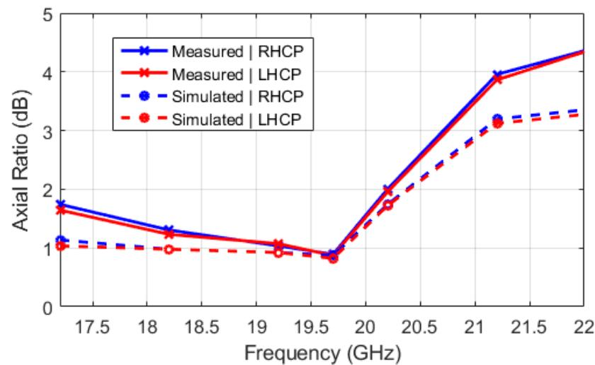
**Figure 11.** Measured and simulated axial ratio as a function of frequency.
