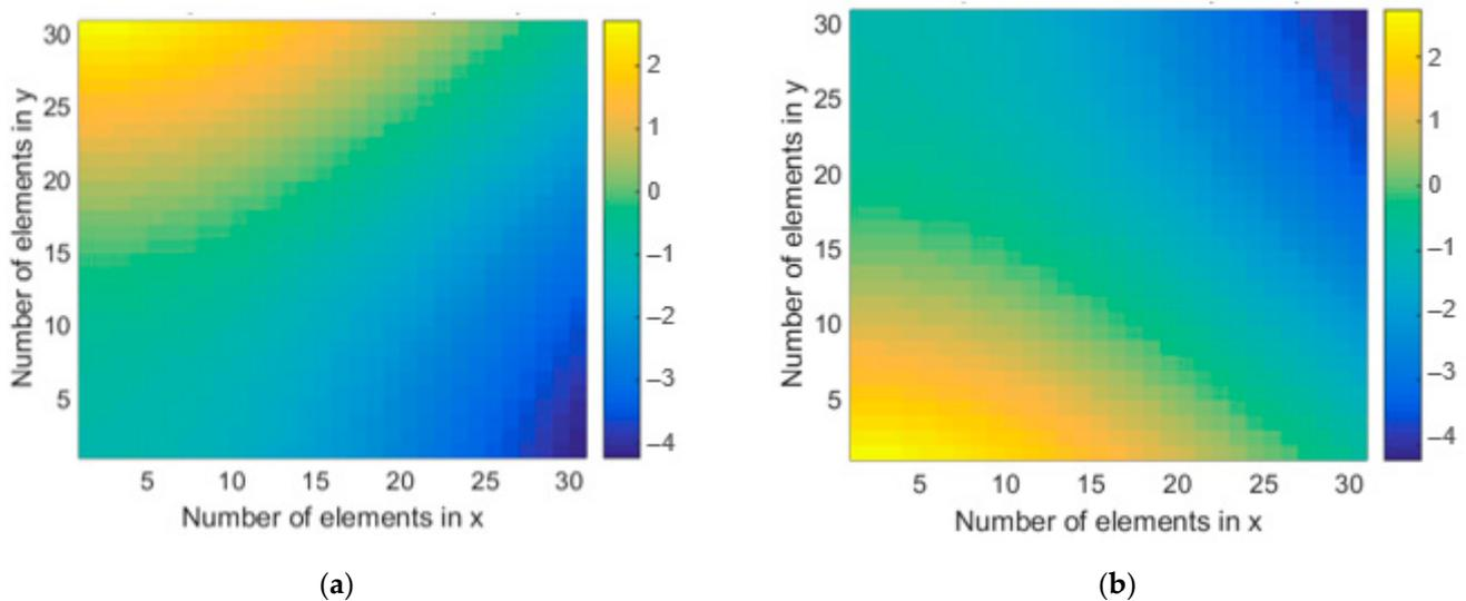
**Figure 4.** Amplitude difference (in dB) between the  $x$  and  $y$  components for (a) the incident LP at  $45^\circ$  slant and (b) the incident LP at  $-45^\circ$  slant.
