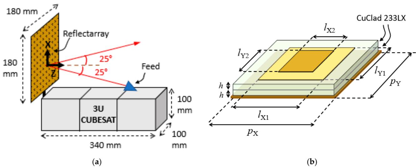
**Figure 2.** (a) Representation of the reflectarray antenna mounted on the CubeSat. (b) Dual-layer reflectarray cell formed by two stacked rectangular patches. All units are in mm.
