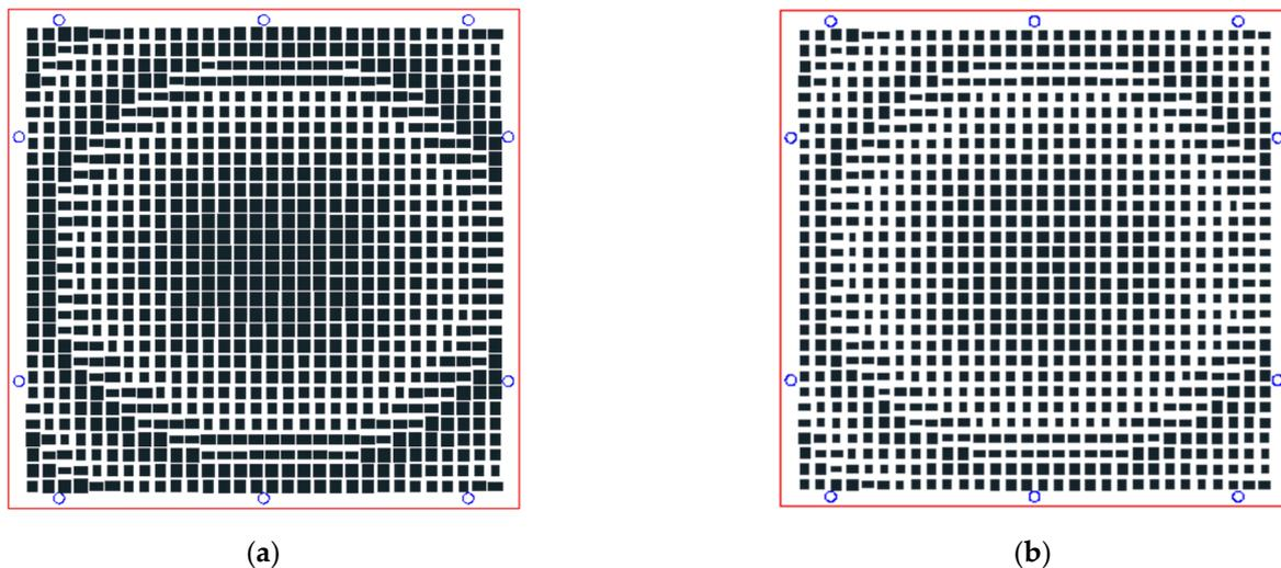
**Figure 6.** Photo-etching masks of the designed reflectarray antenna, corresponding to the (a) lower layer and (b) upper layer of rectangular patches.
