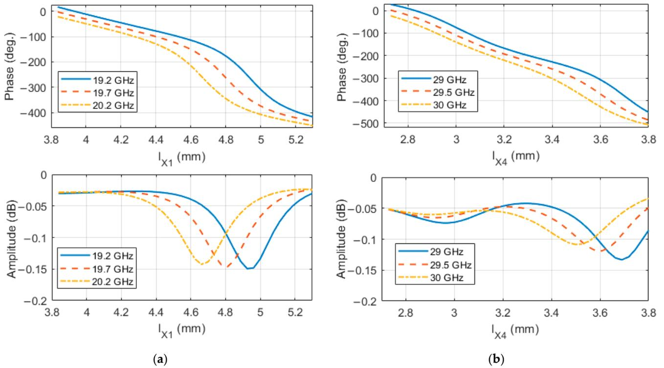
**Figure 14.** Phase and amplitude of the reflection coefficient associated with the  $x$  component of the incident field (a) at the lower band (19.2–20.2 GHz) and (b) at the upper band (29–30 GHz).
