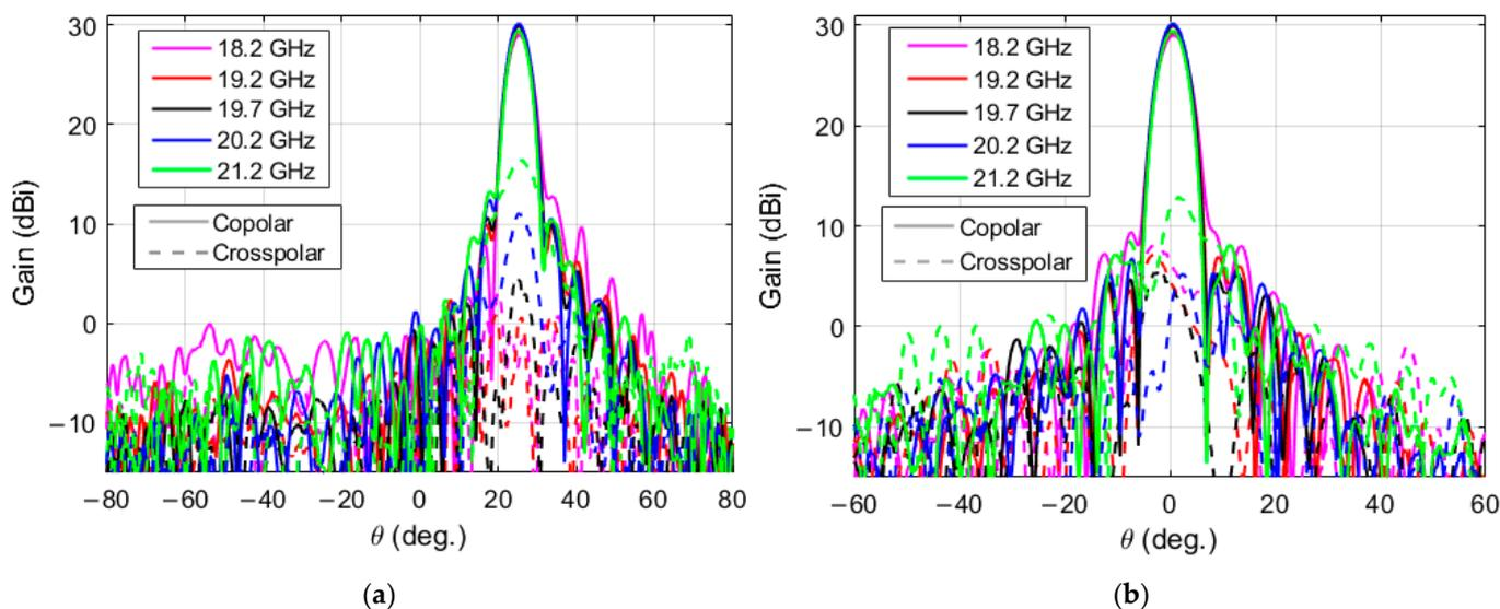
Figure 9. Measured radiation patterns at several frequencies (from 18.2 to 21.2 GHz) for the beam produced in LHCP: (a) in the  $xz$ -plane and (b) in the azimuth plane.
