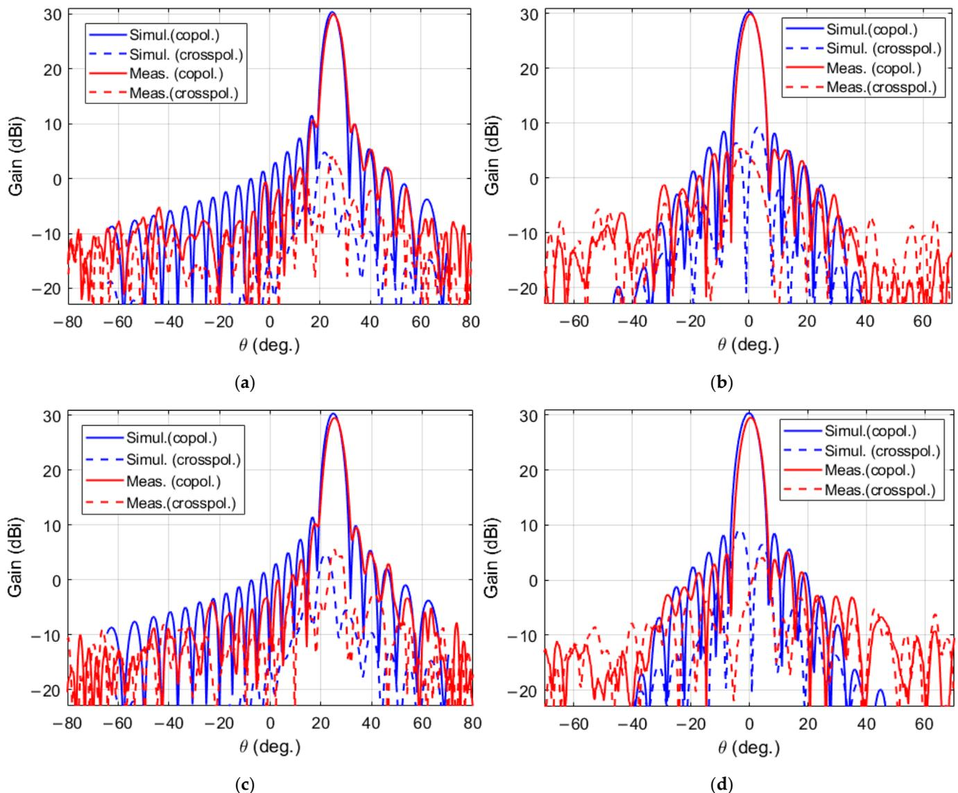
**Figure 8.** Comparison of simulated and measured radiation patterns at 19.7 GHz for the beam produced in RHCP (a) in the  $xz$ -plane and (b) in the azimuth plane, and for the beam produced in LHCP (c) in the  $xz$ -plane and (d) in the azimuth plane.
