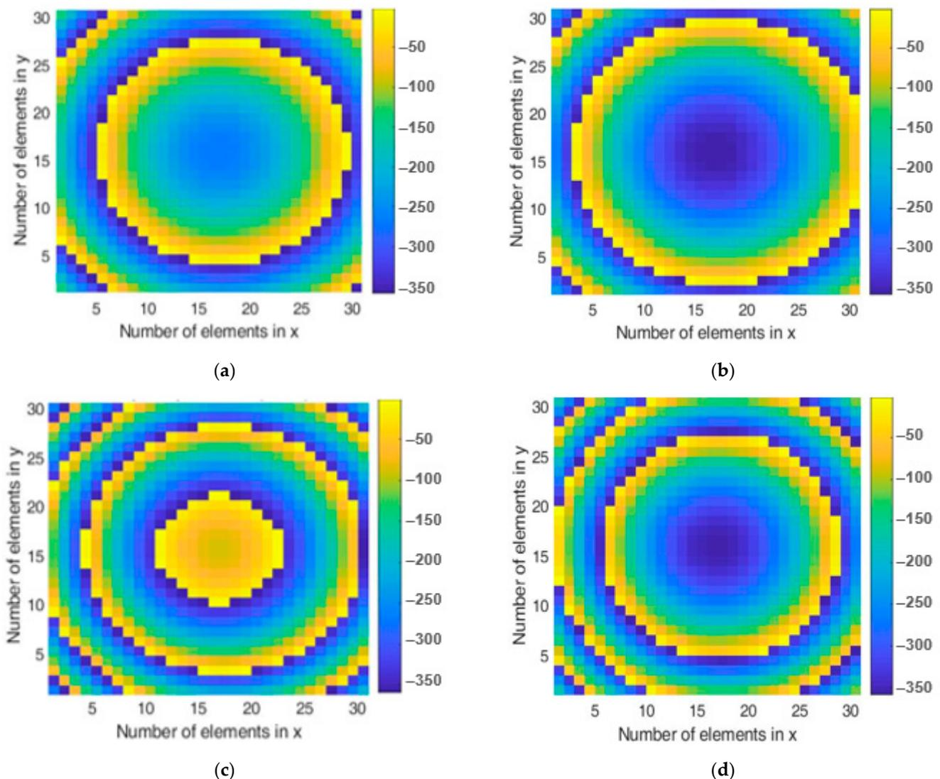
**Figure 12.** Phase shifts (in degrees) that must be introduced by the elements of the dual-band polarizer reflectarray in each component of the incident field: (a)  $x$  component at 19.7 GHz, (b)  $y$  component at 19.7 GHz, (c)  $x$  component at 29.5 GHz, and (d)  $y$  component at 29.5 GHz.
