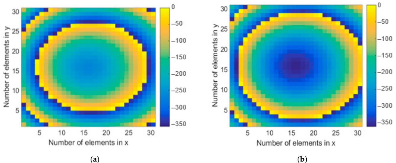
**Figure 3.** Phase shifts (in degrees) that must be introduced by the reflectarray elements in the (a)  $x$  component and (b)  $y$  component of the incident field to produce a dual-CP beam at 19.7 GHz.
