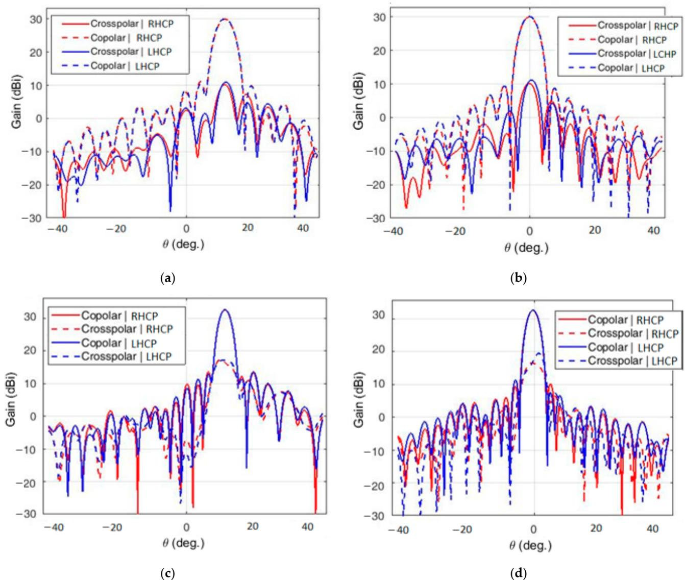
**Figure 16.** Simulated radiation patterns: at 19.7 GHz (a) in the  $xz$ -plane and (b) in the azimuth plane, and 29.5 GHz (c) in the  $xz$ -plane, and (d) in the azimuth plane.
