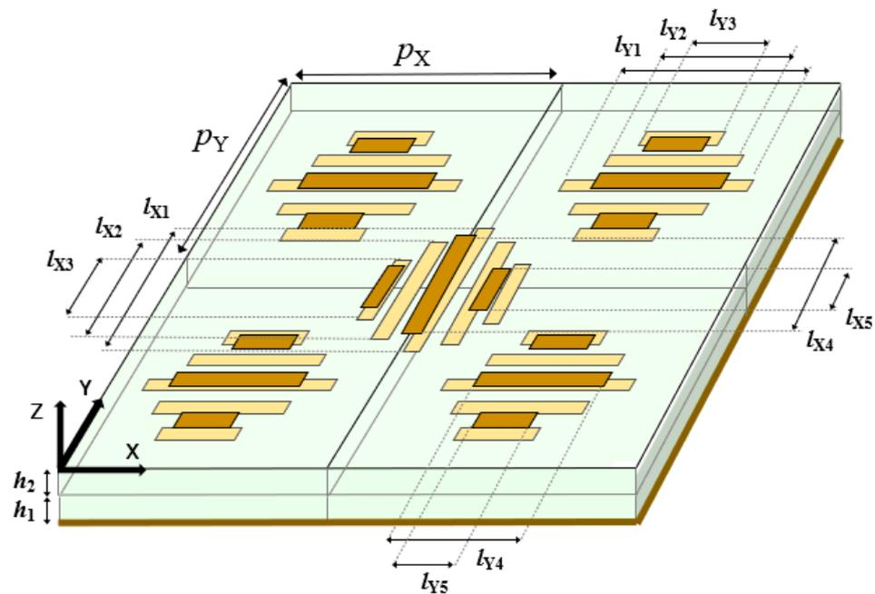
**Figure 13.** Dual-layer reflectarray cells are formed by orthogonally arranged groups of dipoles, each comprising five dipoles on the bottom dielectric layer and three dipoles on the upper layer.
