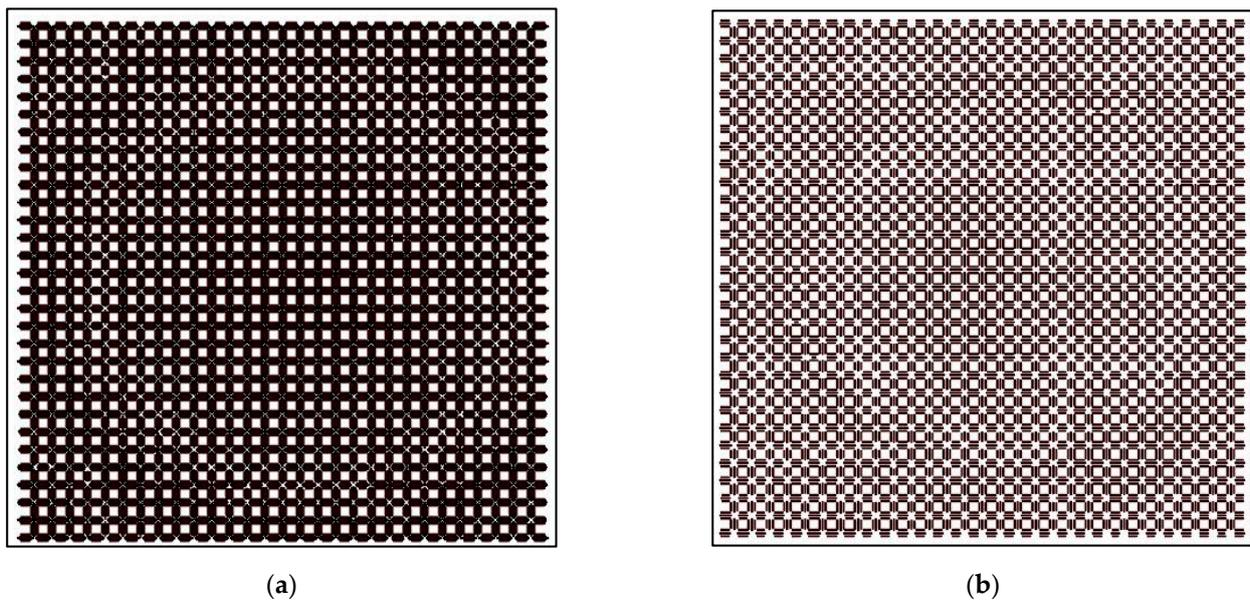
**Figure 15.** Photo-etching masks for the (a) lower layer and (b) upper layer of dipoles.
