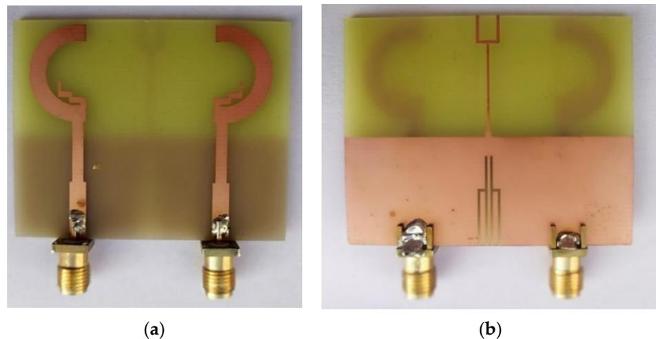
**Figure 6.** The actual picture of the antenna. (a) Top view; (b) bottom view.
