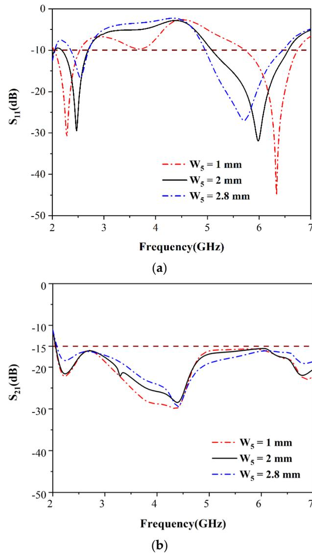
**Figure 3.** Simulated parameters with different values of  $W_5$ . (a) Reflection coefficients; (b) isolation.
