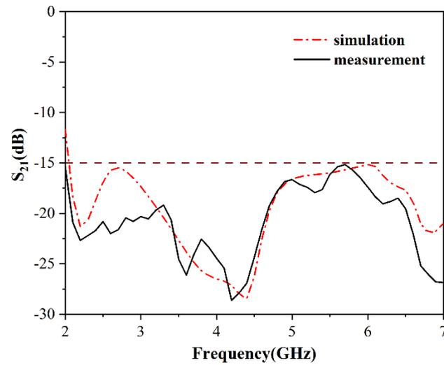
Figure 8. Simulated and measured isolation of the proposed antenna.
