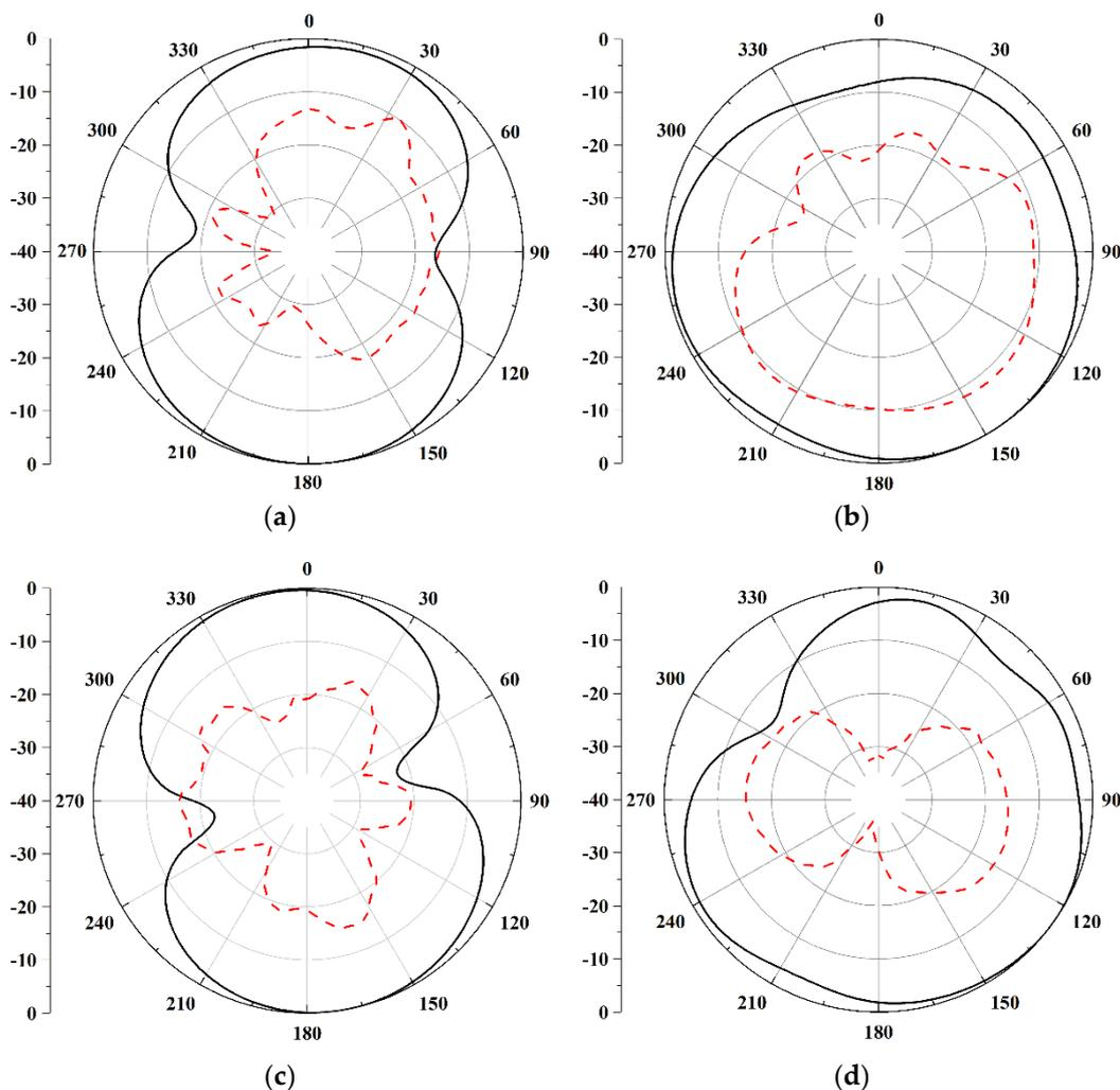
**Figure 10.** Radiation polarization of the proposed antenna. (a) 2.4 GHz E-plane; (b) 2.4 GHz H-plane; (c) 5.5 GHz E-plane; (d) 5.5 GHz H-plane.
