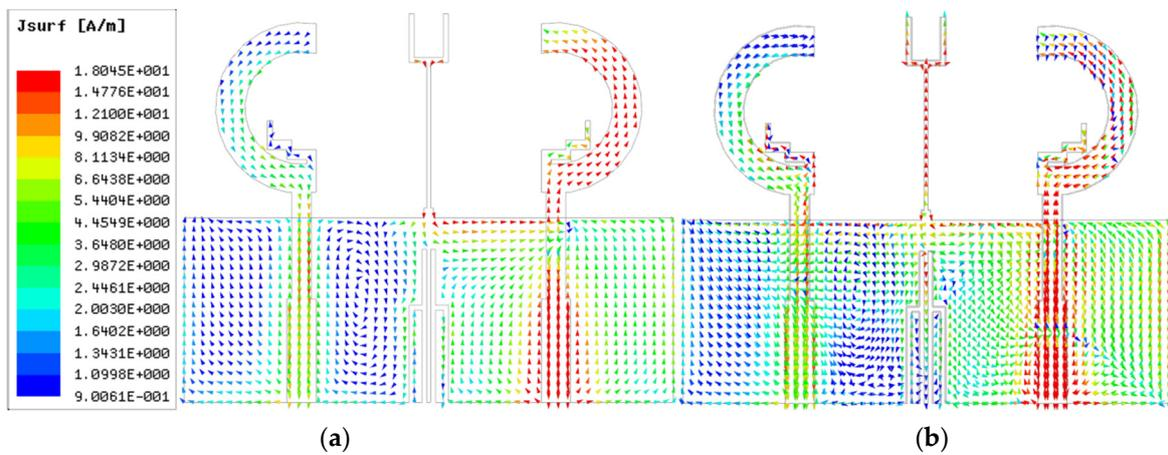
Figure 5. Simulated current distribution at two frequencies. (a) 2.4 GHz; (b) 5.5 GHz.
