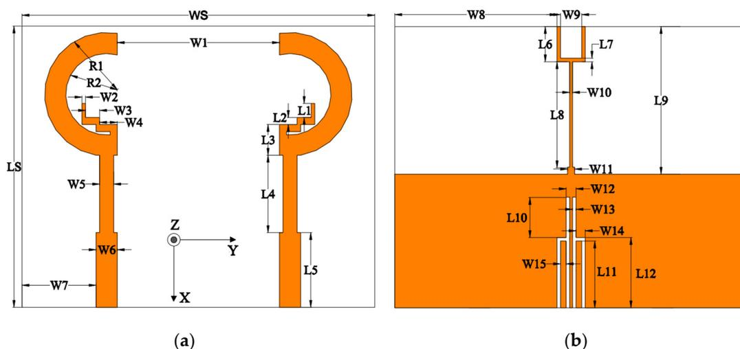
**Figure 1.** Geometry of the proposed antenna. (a) Top view; (b) bottom view.
