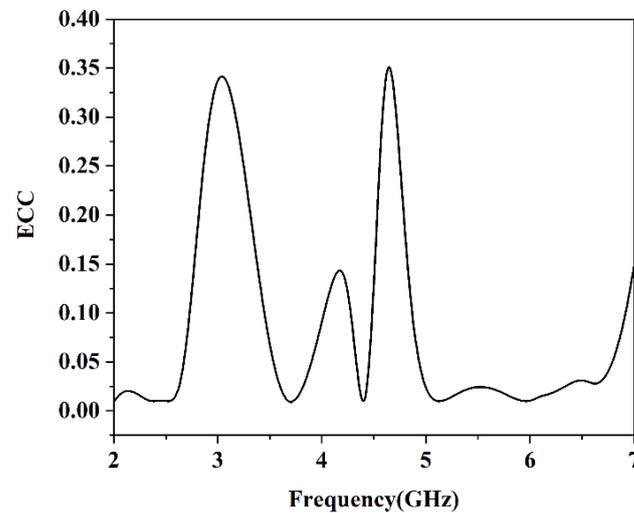
Figure 11. Calculated ECC of the MIMO antenna system.
