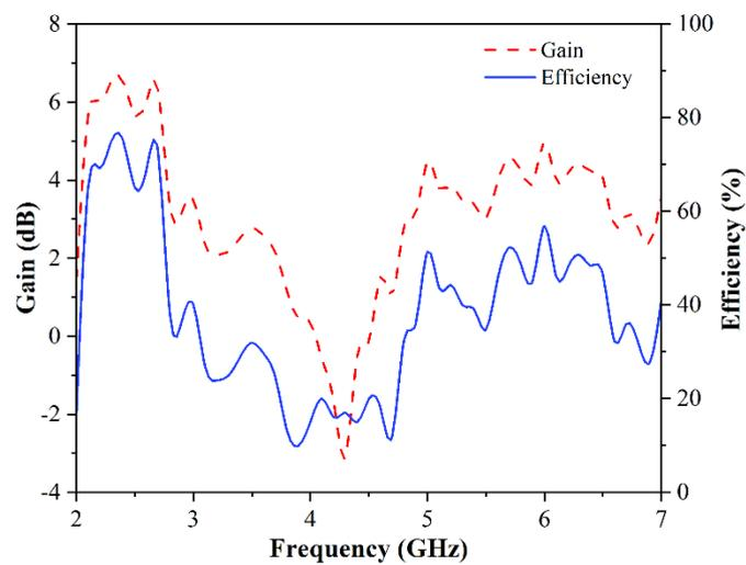
Figure 9. Measured peak gain and radiation efficiency.
