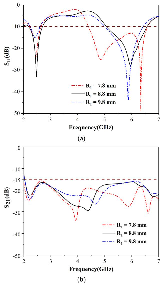
Figure 4. Simulated parameters with different values of  $R_1$ . (a) Reflection coefficients; (b) isolation.
