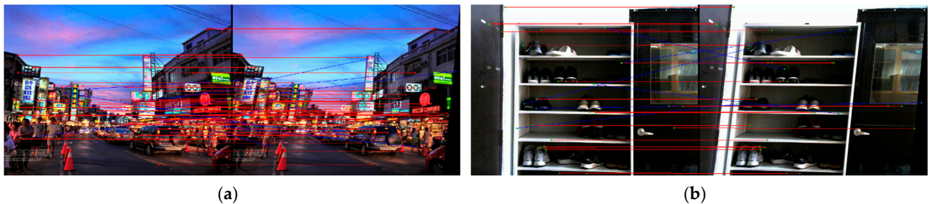
Figure 23. (a) Matching accuracy for a skewed outdoor image is 92.39%, where 85 out of 92 feature points are successfully matched; (b) Matching accuracy for a skewed indoor image is 88.89%, where 48 out of 54 feature points are successfully matched.
