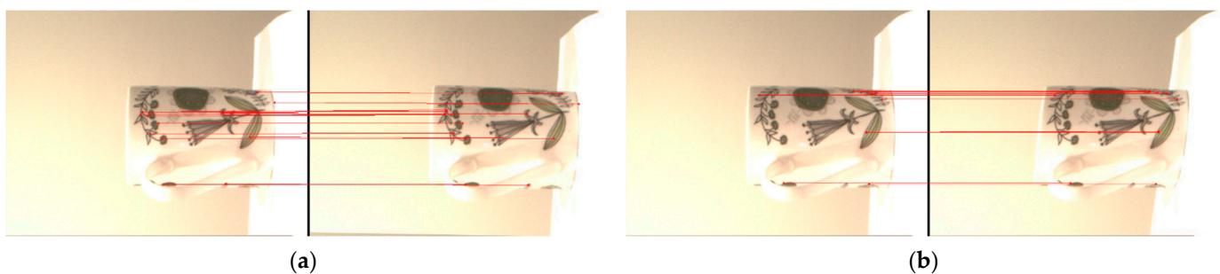
Figure 22. Feature matching results of the original image with (a) the rotated and (b) the skewed image.
