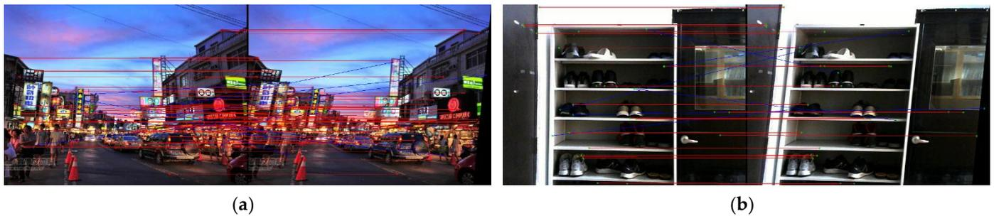
**Figure 23.** (a) Matching accuracy for a skewed outdoor image is 92.39%, where 85 out of 92 feature points are successfully matched; (b) Matching accuracy for a skewed indoor image is 88.89%, where 48 out of 54 feature points are successfully matched.
