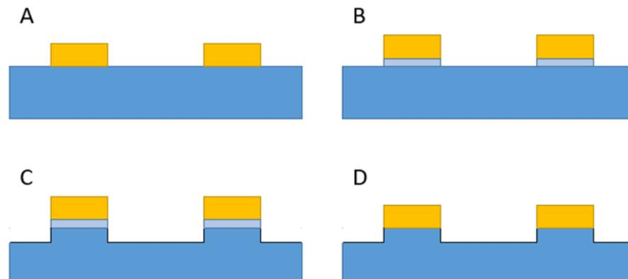
**Figure 2.** A cross-sectional view of lateral PCSS fabricated with (A) metal contacts, (B) a conductive GaN layer and metal contacts, (C) a conductive GaN layer and metal contacts with a mesa etched profile, (D) metal contacts with a mesa etched profile.
