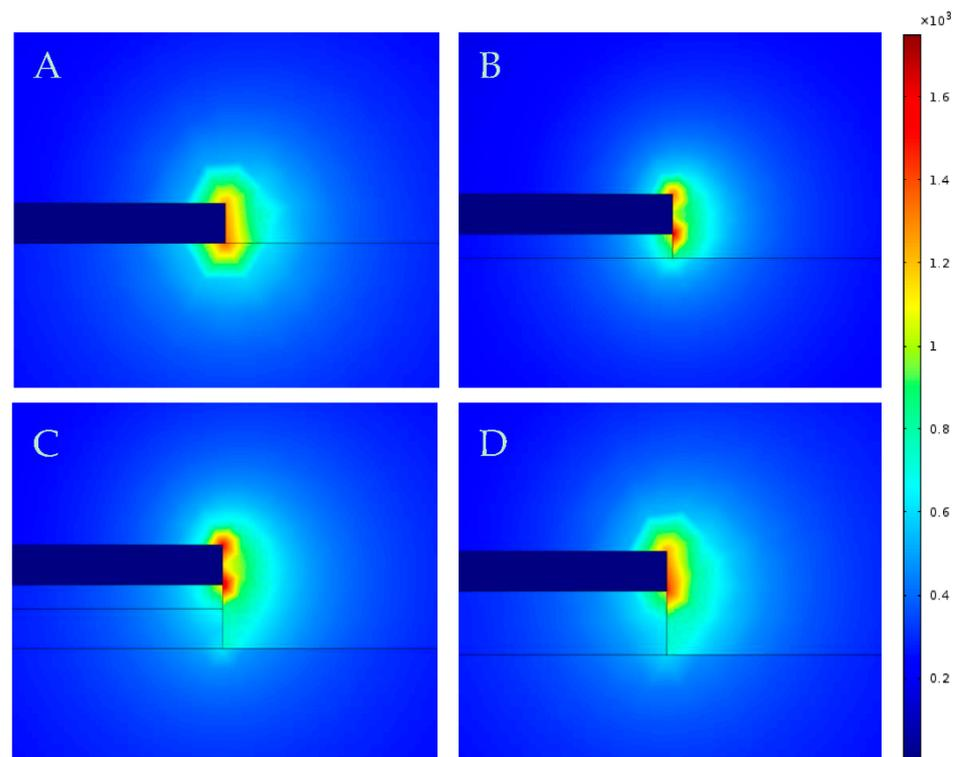
**Figure 3.** Electric field simulation results for lateral PCSS design showing field enhancements when charged to 100 kV/cm for (A) metal contacts, (B) a conductive GaN layer, (C) a conductive GaN layer and mesa etched profile, and (D) mesa etched profile.
