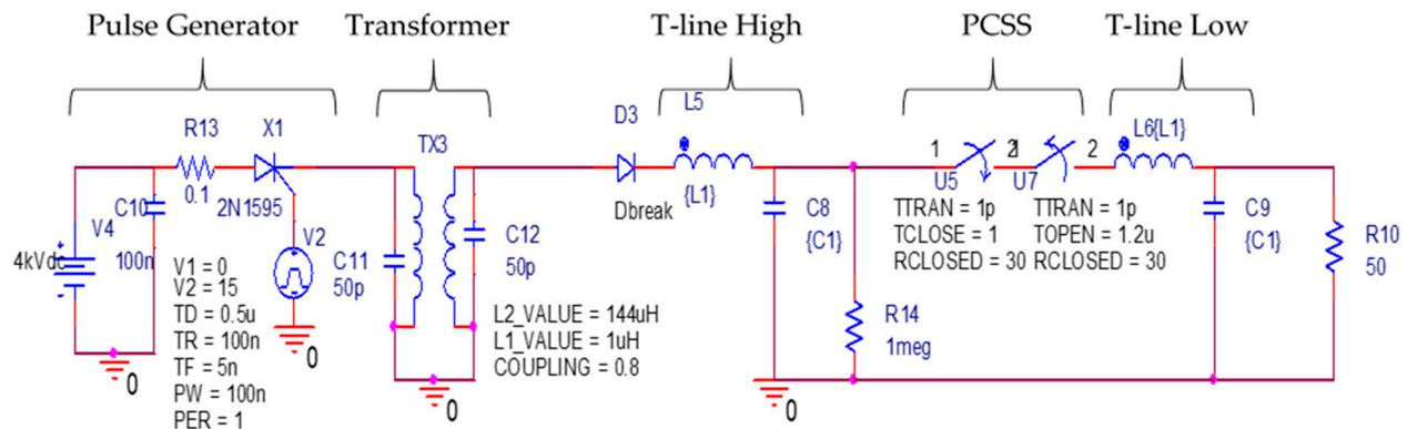
**Figure 1.** Electrical schematic diagram of pulse charging PCSS testbed (PCB). C10—energy storage capacitor; R13—current limiting resistor; X1—thyristor switch; TX3—step-up transformer with estimated parasitic capacitances C11, C12; L1—parasitic inductance; C8—pulse charged capacitance; R14—bleed resistor; U5, U7—behavior model of PCSS (closing and opening switch action); C9—parasitic load capacitance; R10—50 Ohm resistive load.
