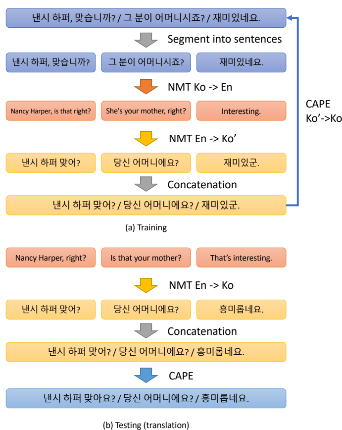
Figure 4. (a) Training a CAPE model requires a monolingual, discourse-/document-level corpus. Each consecutive text is segmented into a set of sentences first. Then, each sentence is translated and then back-translated. The resulting sentence group is concatenated again, and then the CAPE, which consists of a sequence-to-sequence model, is trained to minimize the errors of these round-trip translations. (b) At test time, a trained CAPE fixes sentence-level translations by taking them as a group.
