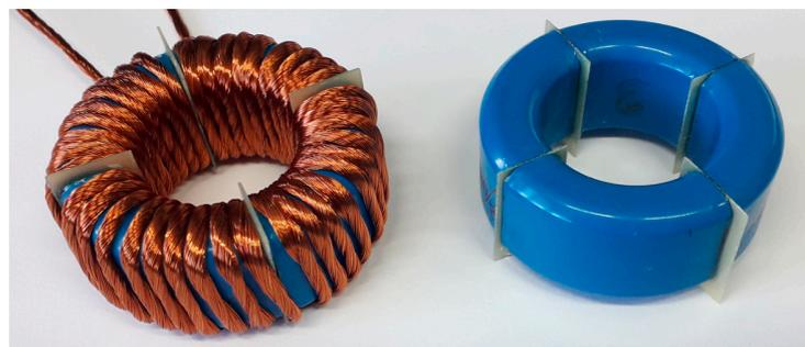
**Figure 4.** Ferrite toroidal inductor with distributed airgap optimized for high-frequency evaluation of selected transistor structures within considered PFC circuit.
