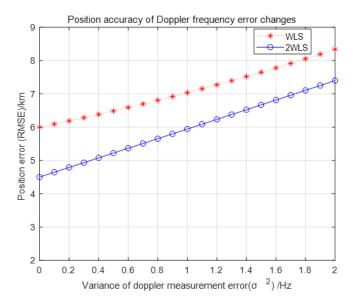
Figure 3. The relationship between the Doppler frequency error and positioning accuracy.
