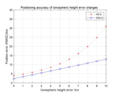
Figure 4. The relationship between the reflected ionospheric height error and positioning accuracy.
