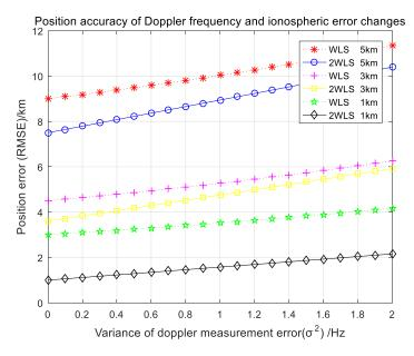
**Figure 5.** The relationship between the Doppler frequency error, ionospheric height error and positioning accuracy.
