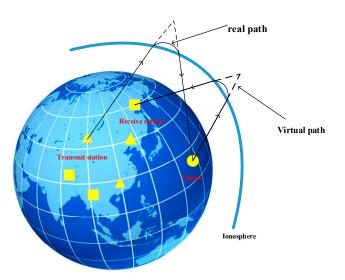
**Figure 1.** The propagation path of the signal after reflection from the ionosphere. The virtual path is equivalent to the propagation in the air. The true path is curved due to the reflection of the ionosphere.
