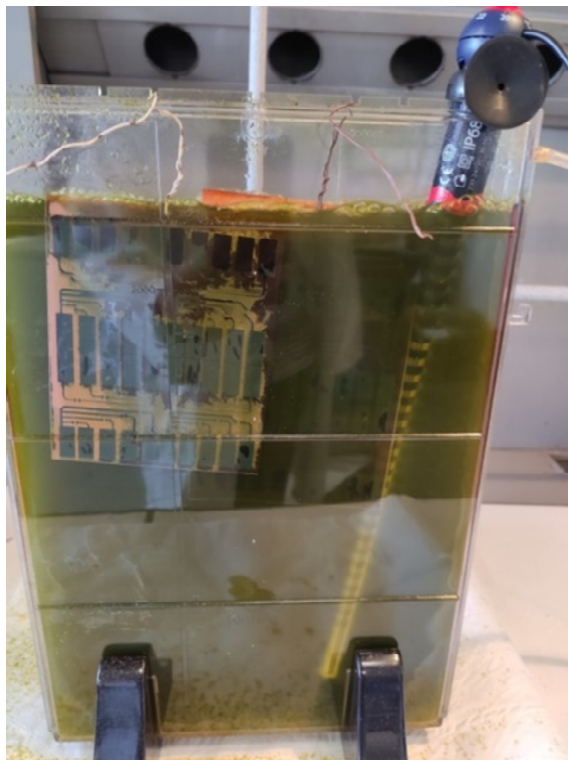
Figure 2. Vertical Etching tank.
