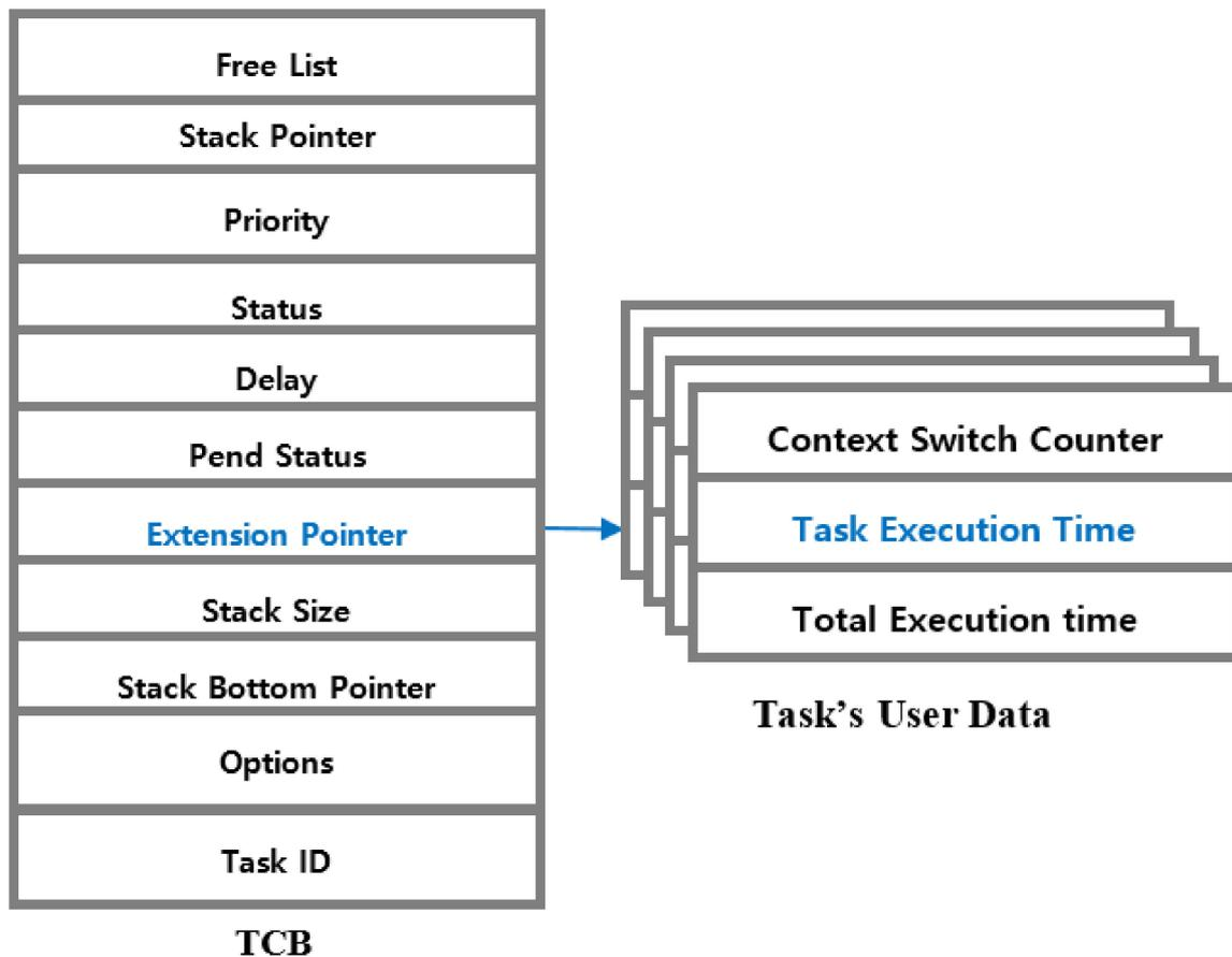
**Figure 2.** Task Control Block (TCB) extension for CPU usage monitoring.
