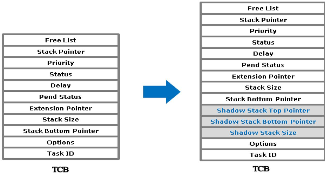
Figure 3. Task Control Block (TCB) with shadow stack information.
