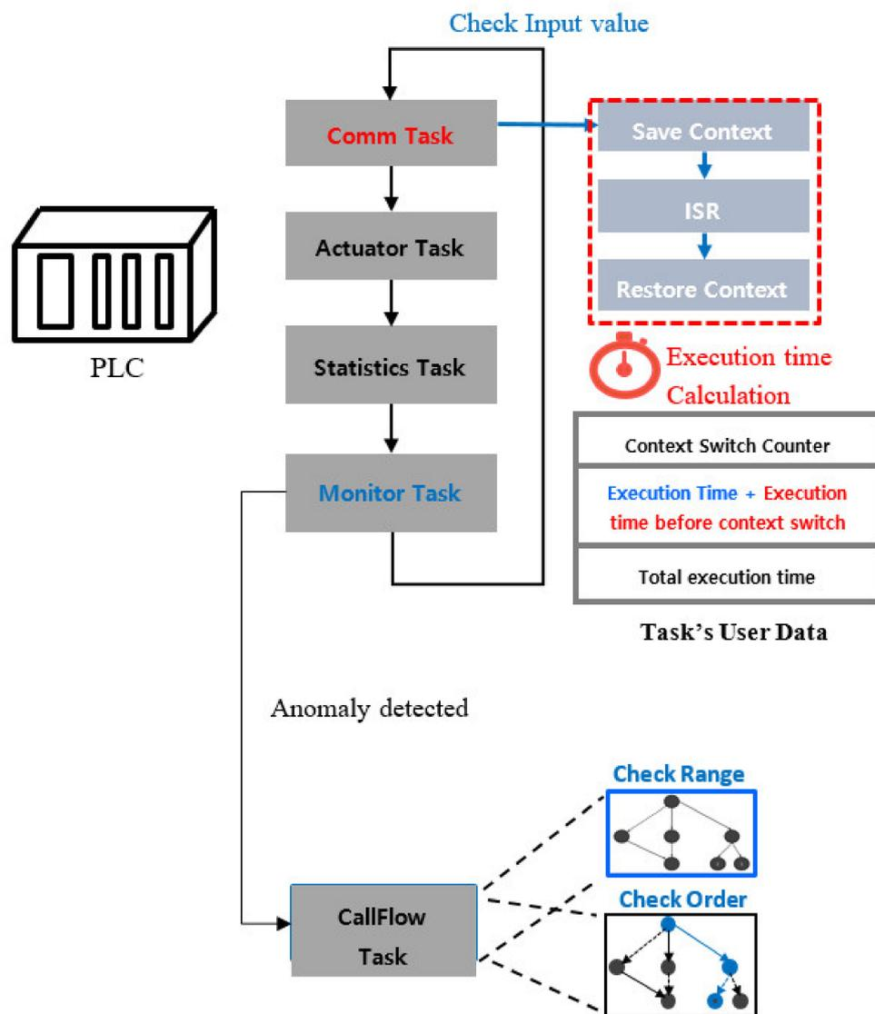
**Figure 1.** Measurement of task execution time and control-flow anomaly detection.
