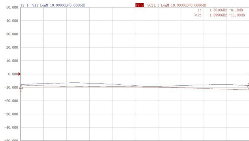
Figure 14. The measured S21 of mixer 2 (down-conversion).
